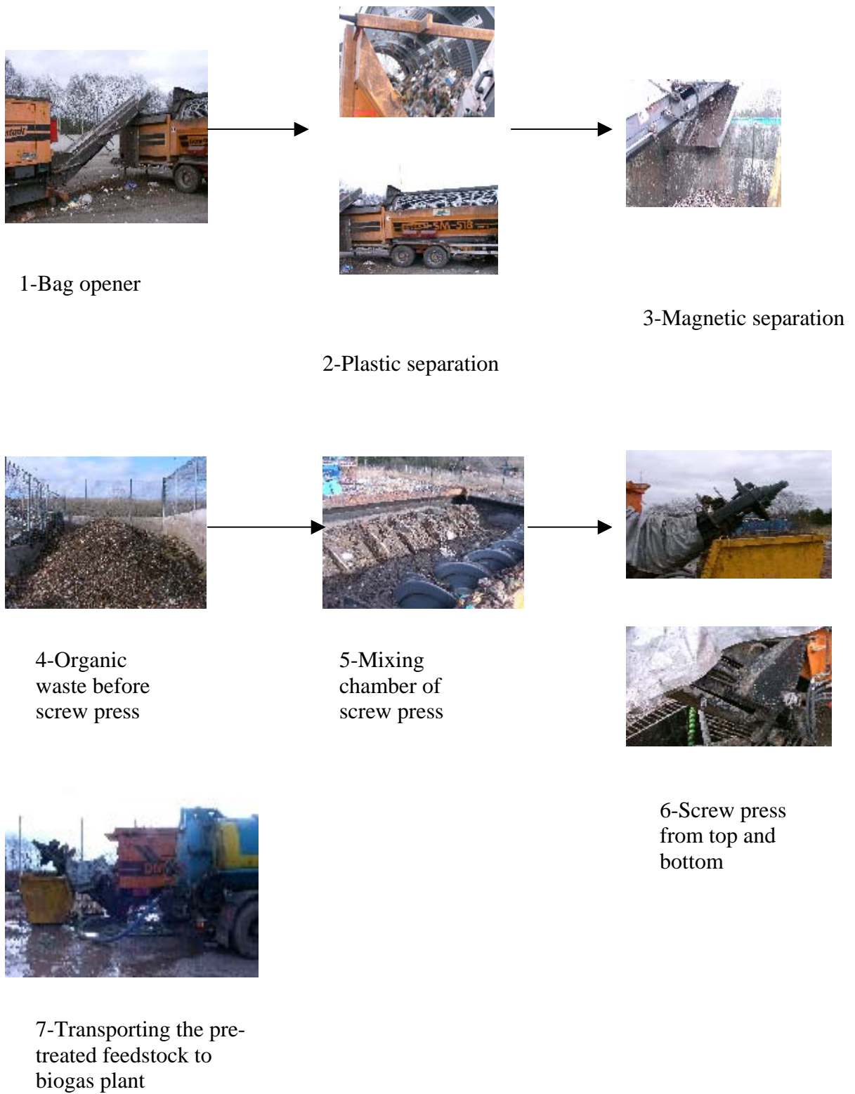
Figure 5.1 Pre-treatment processes in Eslöv.
