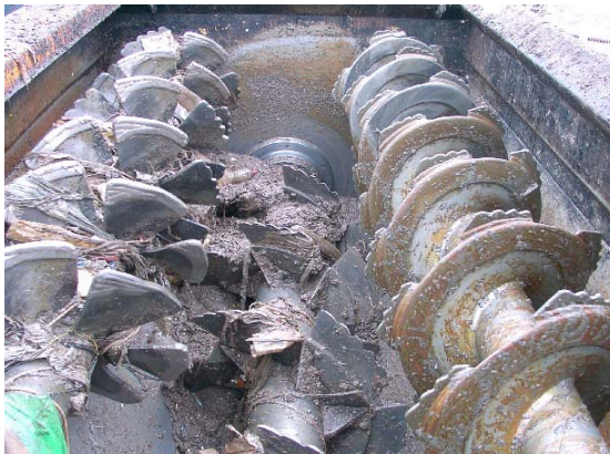
Figure 4.2 Mixing chamber with mills and screw shaft in the bottom followed with screw press.
