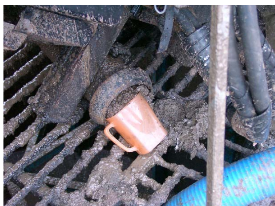
Figure 6.2 Sampling from slurry after screw press.
