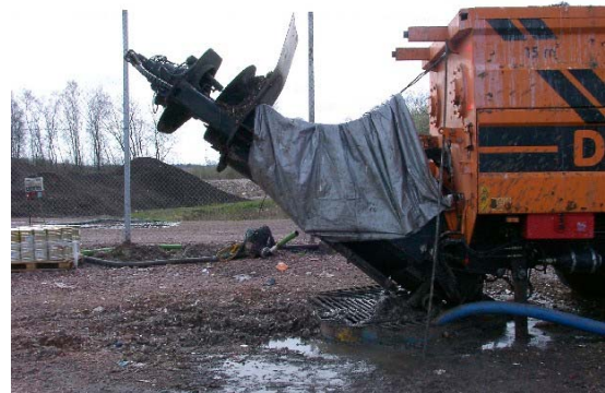
Figure 4.2 Mixing chamber with mills and screw shaft in the bottom followed with screw press.
