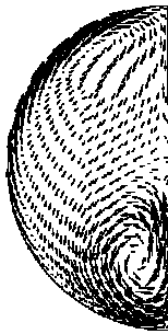
Figure 4.21: Secondary flow at station 5. Grid 2, RNG k-\epsilon , l = 0.0015 and I = 1\% .
