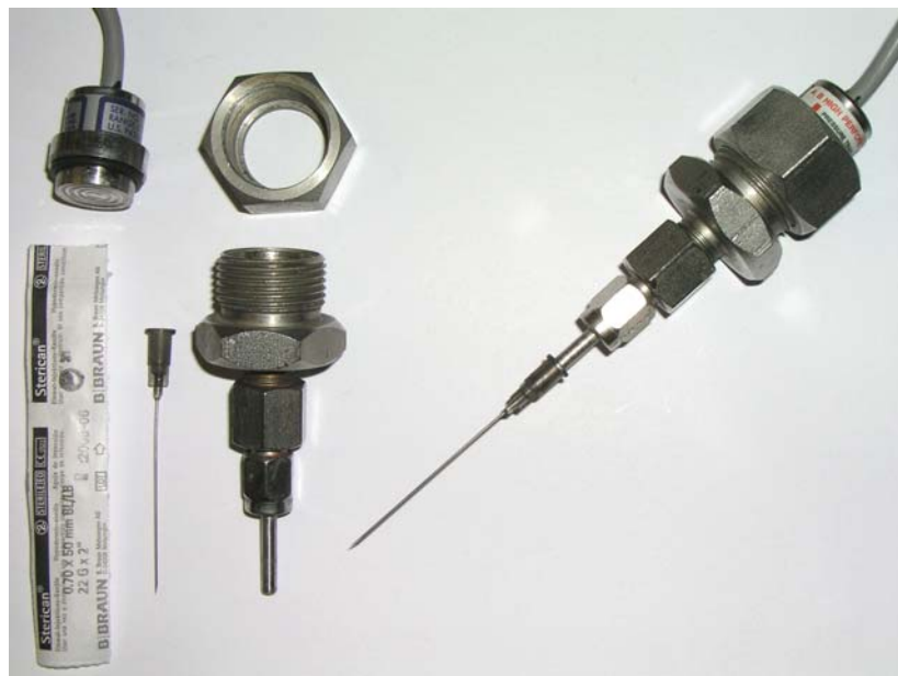
Figure 14. Picture of pressure gauge and the needle used to measure the capillary pore pressure.
