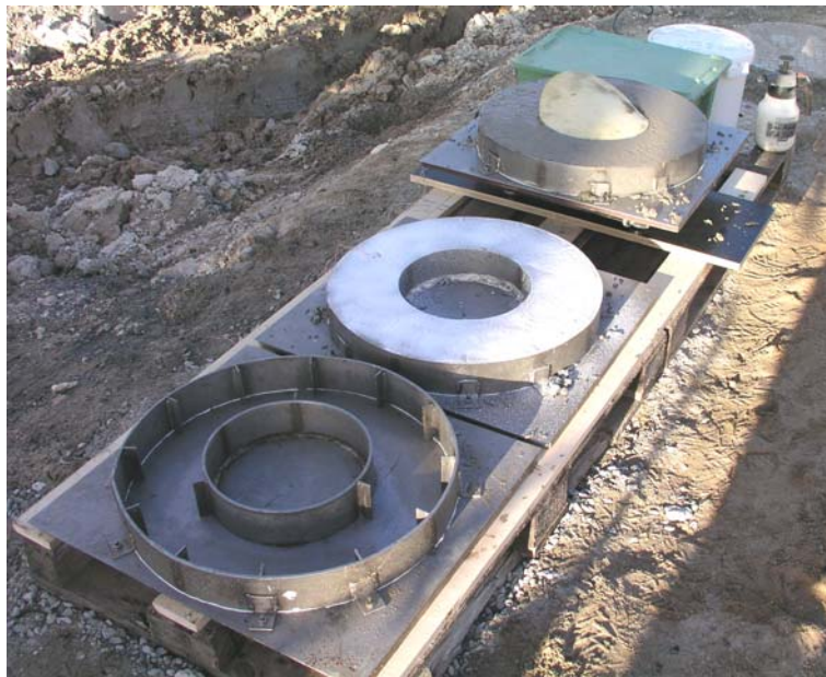
Figure 137. Ring test specimens in the field study.
