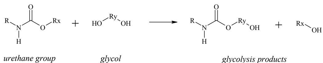
Figure 3.4 Glycolysis reaction of polyurethane.
