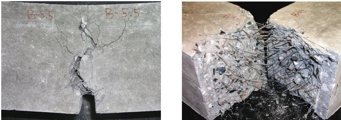
Figure 77. Examples of diffusive and multiple cracking in a notched beam specimen ( w/b 0.42 and V_f = 1.0 %, type RC-65/35).
