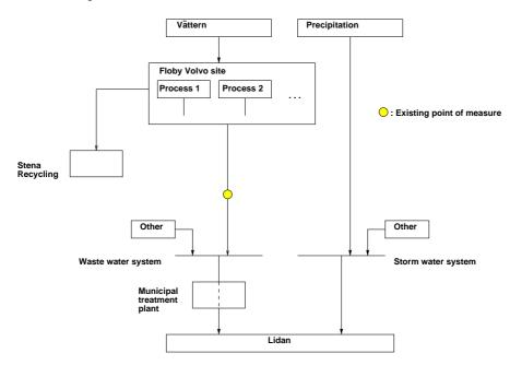
Figure 17: Diagram displaying what measurement points exist at the VCM site in Floby where water flow and pollution concentrations are measured. Level of pollution is measured occationally in the main sewer system but the magnitude of the flow is not measured. Measurements are taken occationally on the wastewater flow being shipped for off-site treatment.
