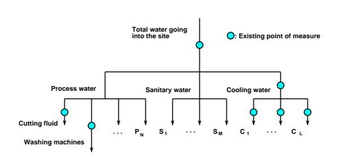
Figure 14: Diagram displaying what blue water flows are known at the VCM site in Skövde. P, S and C represent production processes, sanitary appliancies and cooling systems, respectively. The blue water flows to cutting processes and cooling systems are known.
