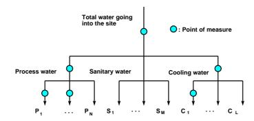
Figure 6: Flowchart used to display what blue water points of measurement are known at a site. The lines in the flowchart represent different blue water flows and the dots represent blue water measurement points. This chart does not represent any specific site and the dots have been placed ideally as an example.
