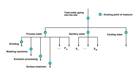
Figure 16: Diagram displaying what blue water flows are known at the VCM site in Floby. P, S and C represent production processes, sanitary appliancies and cooling systems, respectively. The blue water flows to the most water consuming processes are known.
