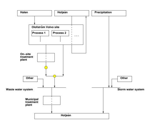
Figure 13: Diagram displaying what measurement points exist at the VCM site in Olofström where water flow and pollution concentrations are measured. Measurements are continuously made on the waste water coming out of the on-site treatment plant and in the main wastewater sewer.
