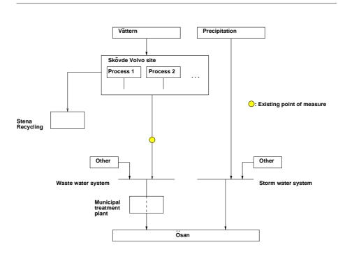
Figure 15: Diagram displaying what measurement points exist at the VCM site in Skövde where water flow and pollution concentrations are measured. Level of pollution is measured occationally in the main sewer system but the magnitude of the flow is not measured. The flow of the water going to the off-site treatment plant is measured but not the pollution concentrations.
