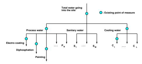
Figure 10: Diagram displaying what blue water flows are known at the VCM site in Ghent. P, S and C represent production processes, sanitary appliancies and cooling systems, respectively. The blue water flows of approximately 90% of the production processes and 75% of the cooling systems are measured continuously.
