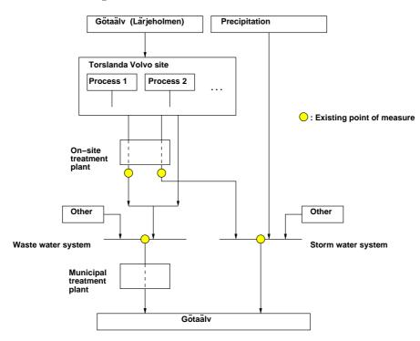
Figure 9: Diagram displaying what measurement points at the VCM site in Torslanda exist where water flow and pollution concentrations are measured. Measurements are made continuously on the waste water coming out of the on-site treatment plant and in the main sever systems.
