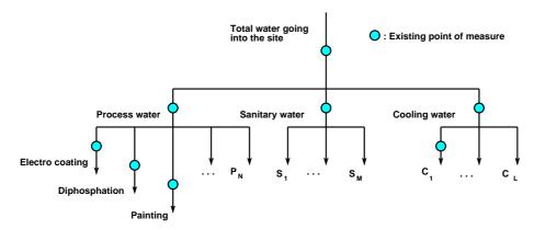
Figure 8: Diagram displaying what blue water flows are known at the VCM site in Torslanda. P, S and C represent production processes, sanitary appliancies and cooling systems, respectively. The blue water flow within each house on the site as well as the flow of the most water consuming processes and some cooling systems are measured continuously.
