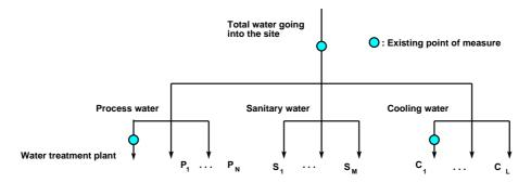
Figure 12: Diagram displaying what blue water flows are known at the VCM site in Olofström. P, S and C represent production processes, sanitary appliancies and cooling systems, respectively. The blue water flows to water treatment plant and some cooling systems are known.
