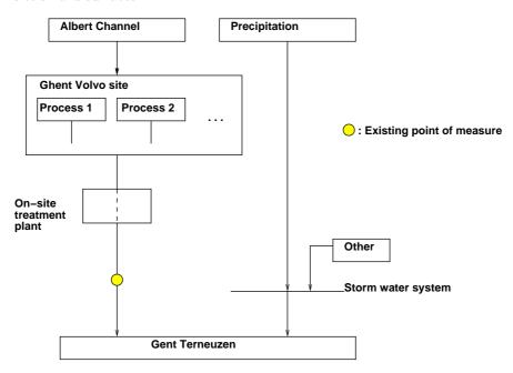
Figure 11: Diagram displaying what measurement points exist at the VCM site in Ghent where water flow and pollution concentrations are measured. Measurements are continuously made on the waste water coming out of the on-site treatment plant.
