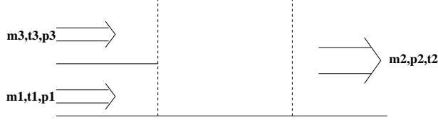
Figure A.3: Mixing of two flow streams
