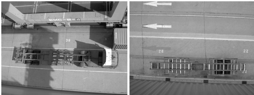
Figure 4.1: A road chassis (left) and a terminal chassis (right), both images taken from the crane structure.
