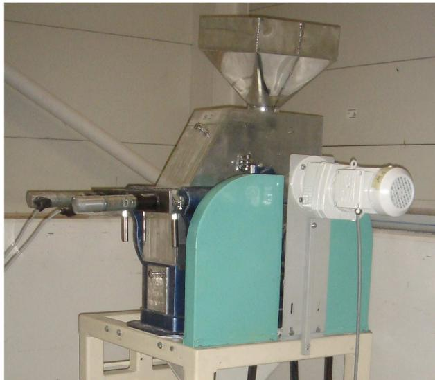
**Figure 2.1:** *The roller mill experimental machine.*
