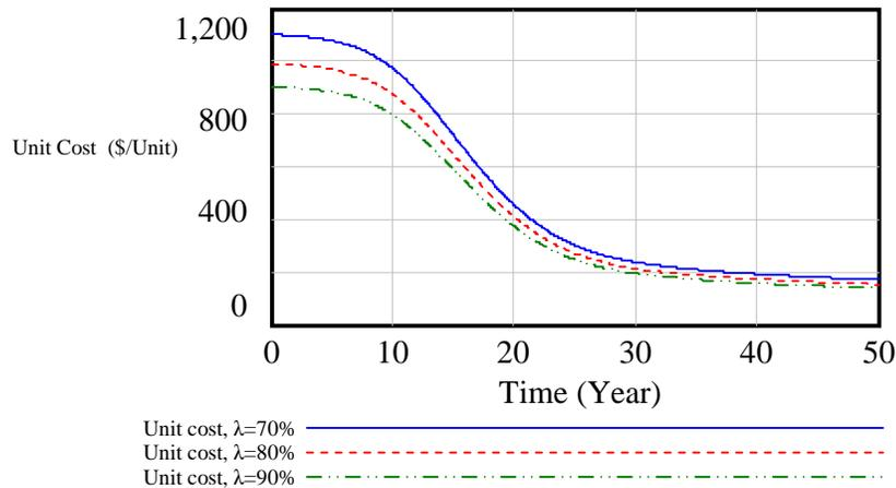
**Figure 4.10** Time dominant plot of unit cost  $C_u$ , considering different capacity utilization ratios
