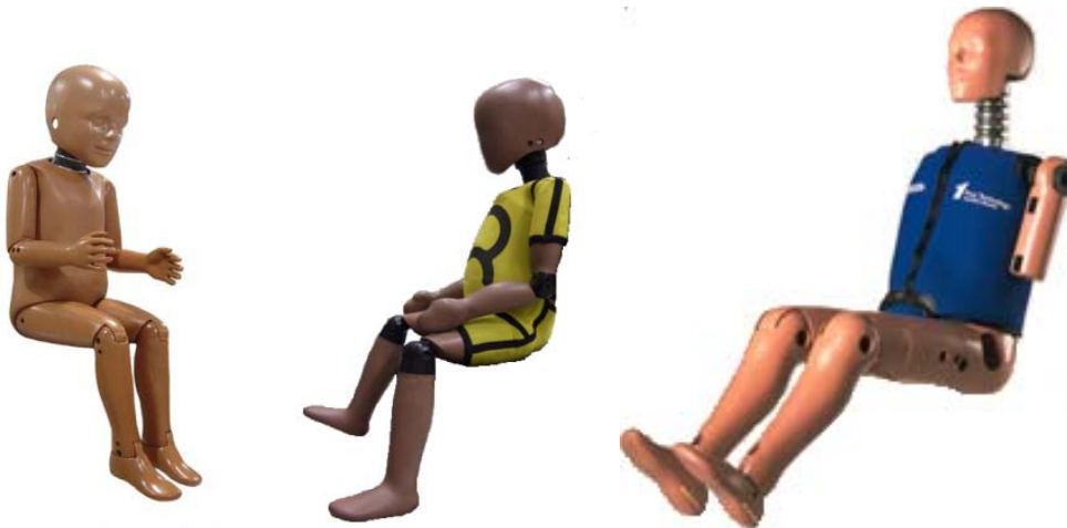
Figure 3. The Hybrid III 3-year-old ATD (left); the Q3 ATD (centre); the SID-II's 5 th percentile adult female ATD (right). (Pictures not to scale)
