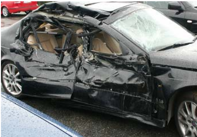
Case 8. The sill was pulled up by the B-pillar but was not directly involved.
