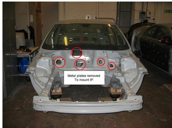
**Figure A.3.:** Metal plates removed to mount the IP.
