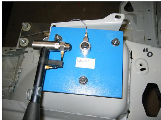
**Figure 3.30.:** Cap fixture with an impact hammer for point inertance measurement.
