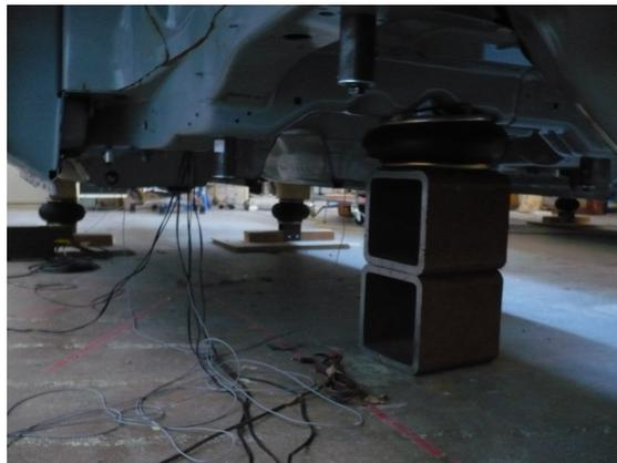
**Figure 3.1.:** Air-mounts positions
