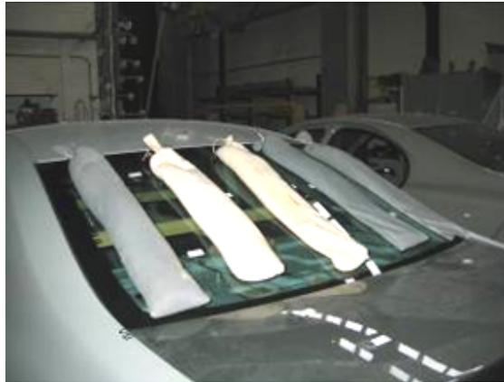
**Figure 3.27.:** Mass-loading the rear window with sandbags.
