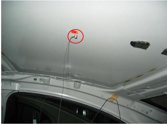
(a) Accelerometer position on the roof.
