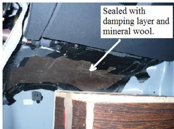
**Figure 3.13.:** IP lower cavities sealed with damping layer and mineral wool.
