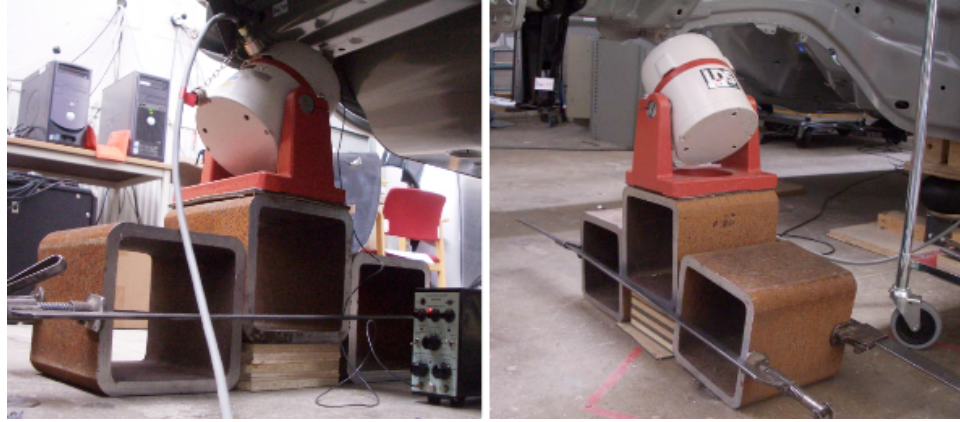
Figure 4.11: Preliminary test shakers set-up for 45-degrees excitation (left: rear shaker, right: front shaker)
