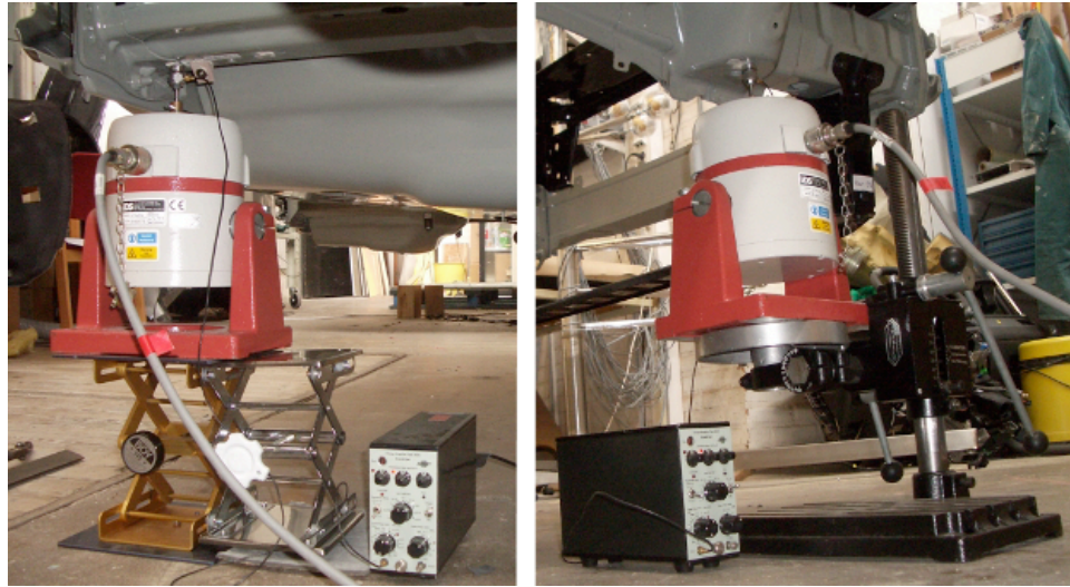
Figure 4.7: Preliminary test shakers set-up (left: rear shaker, right: front shaker). Shakers on height-adjustable supports
