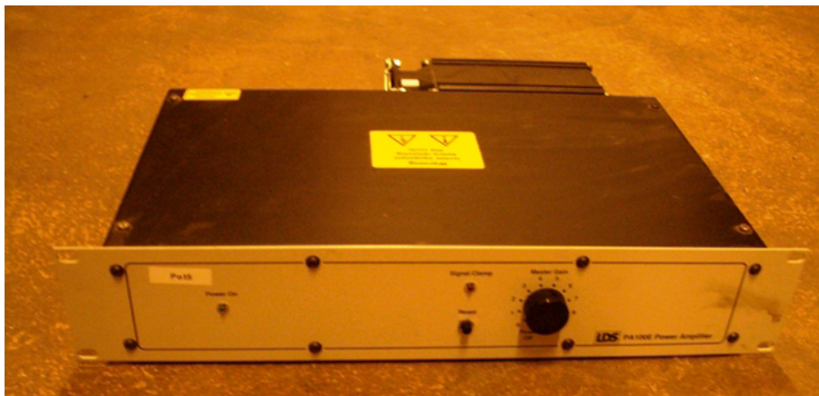
Figure E.2: Power amplifier
