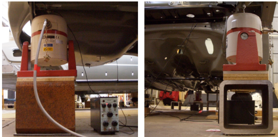
Figure 4.9: Preliminary test shakers set-up for vertical excitation (left: rear shaker, right: front shaker)
