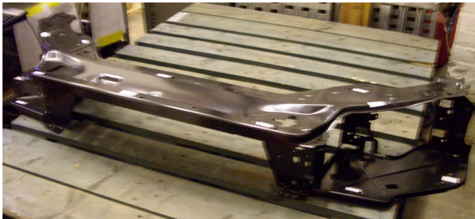
Figure 4.1: Grill Overhanging Reinforcement: GOR
