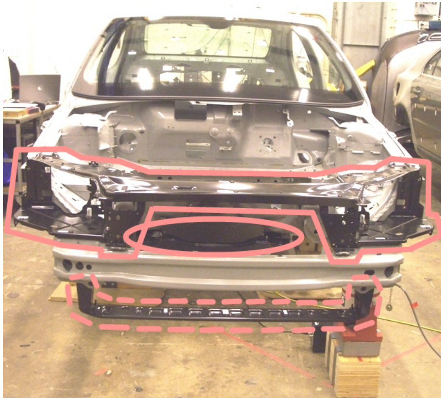
Figure 1.1: Bolted items: Grill Over-hanging Reinforcement (polygon), Radiator Beam (dash-line) and Tunnel Brace (ellipse)
