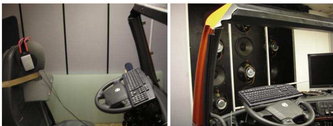
Picture 3 Listening test setup: demo of a truck cabin and custom built subwoofer
