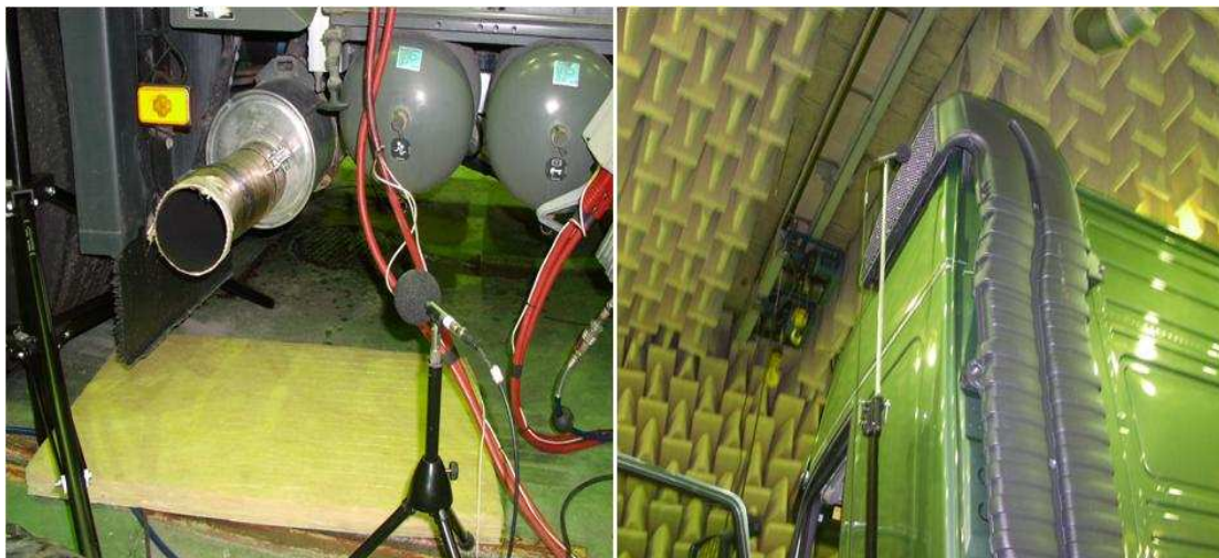
Picture 2 Microphone positions during recording intake and exhaust noises
