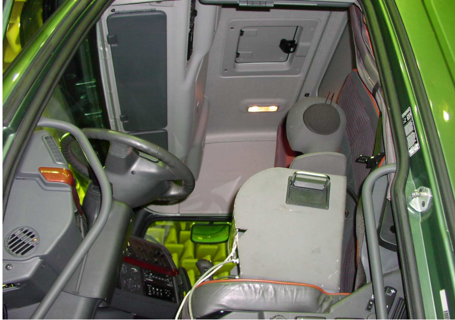
Picture 1 Position of the artificial head during measurements in semi-anechoic room at Volvo Noiselab
