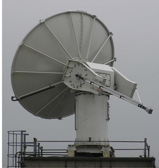
**Figure 2.1: Reflector and Standard Horn antennas, Courtesy of SELEX-SI Gematronik Co.**
