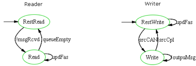
figure 2.3: The reader and writer from figure 2.2, modelled as Automata. It is important to know that they have separate alphabets. The “!” character means that the event is uncontrollable.
