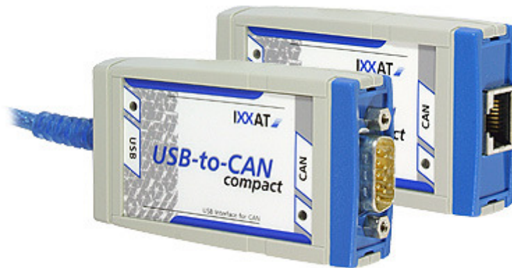
Figure 11: With an USB to CAN device it is possible for a regular PC without CAN-port but with a USB-port to communicate over CAN. The front device where used in this project.
