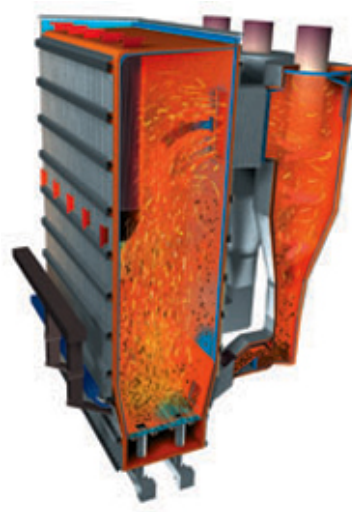
Figure 2: The world's largest (550 MW th ) biomass-fired CFB boiler in Alholmens Kraft (Finland). a. Photo of plant (courtesy of Alholmens Kraft, plant owner) b. Illustration of circulating loop (courtesy of Metso Power, manufacturer)
