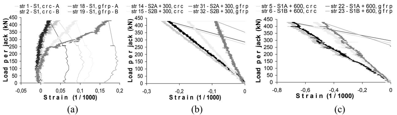
Figure 41. Strain measurements at the corresponding sides of the bimaterial interface in the deck for side A and side B of the beam (measured above the centre of the beam flanges) at various distances from the supports: (a) at support 1, (b) 300 mm from support 2 and (c) 600 mm from support 1.
