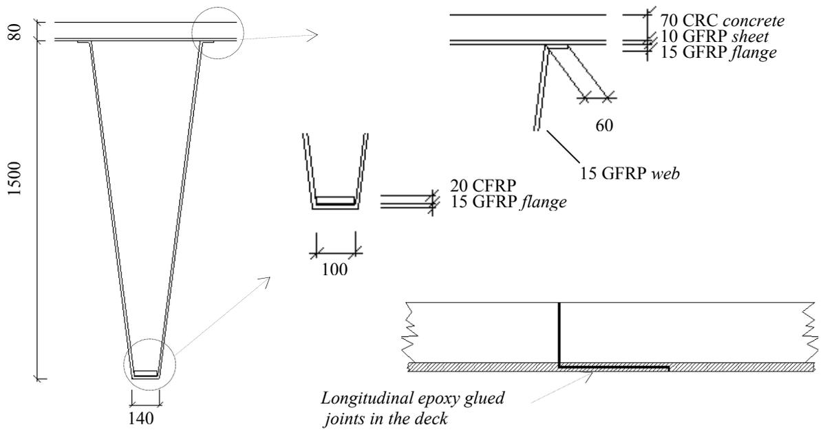
Fig. 4: Detailed dimensions (in mm).
