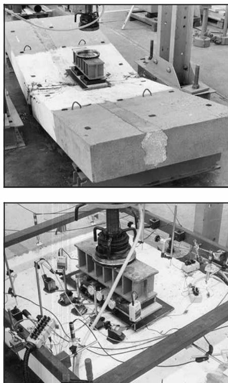
Fig. 4: Above is one of the specimens of fatigue test series UP3, after ultimate static loading to failure. Below is a close view of the set-up for the same series. The eccentric longitudinal joint and the centric loading simulating a wheel's pressure can be seen in the pictures
