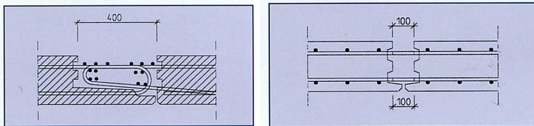
**Figure 1.** Comparison of joints between prefabricated deck slabs; the conventional joint (left) and the new joint (right).
