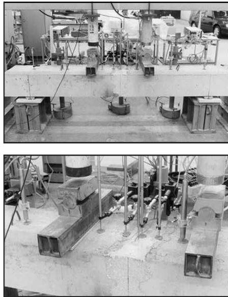
Fig. 3: Above is the set-up for static loading test. Loading consists of two symmetric point loads. Specimens span 2000 mm and the space between loading points is 600 mm. Below is a close view of the set-up. Vertical deflection was gauged by displacement transducers and strain gauges were attached to the reinforcing bars to be spliced, one at each side of the interface between the CRC and the ordinary concrete. Essentially the same set-up is used for two of the series in the fatigue test
