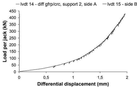
**Figure 8.** Differential displacement between the bottom of the GFRP deck sheet and the centre of the CRC overlay at support 2. Notice the significant displacement taking place on side A of the beam (the side which was damaged during transportation), while the displacement is practically zero on side B (the graph is almost parallel to the load axle).
