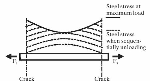
Fig. 7: Schematic presentation of the variation in tensile stress between two cracks due to bond action for a reinforcing bar in tension while unloading from maximum load. Mainly tensile loading is assumed.  $F_s$  is the tensile force in the rebar
