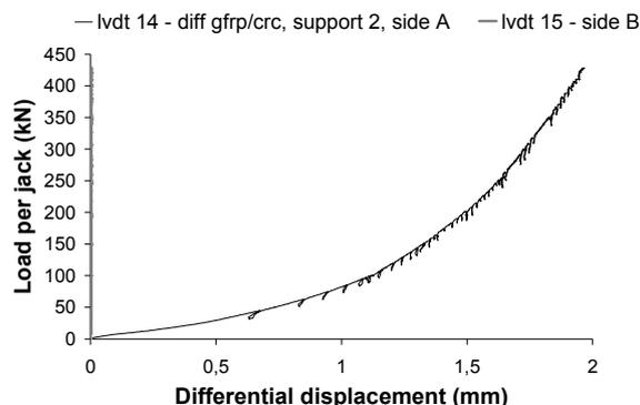
Figure 37. Differential displacement between the bottom of the GFRP deck sheet and the centre of the CRC overlay at support 2. Notice the significant displacement taking place on side A of the beam (the side which was damaged during transportation), while the displacement is practically zero on side B (the graph is almost parallel to the load axle).
