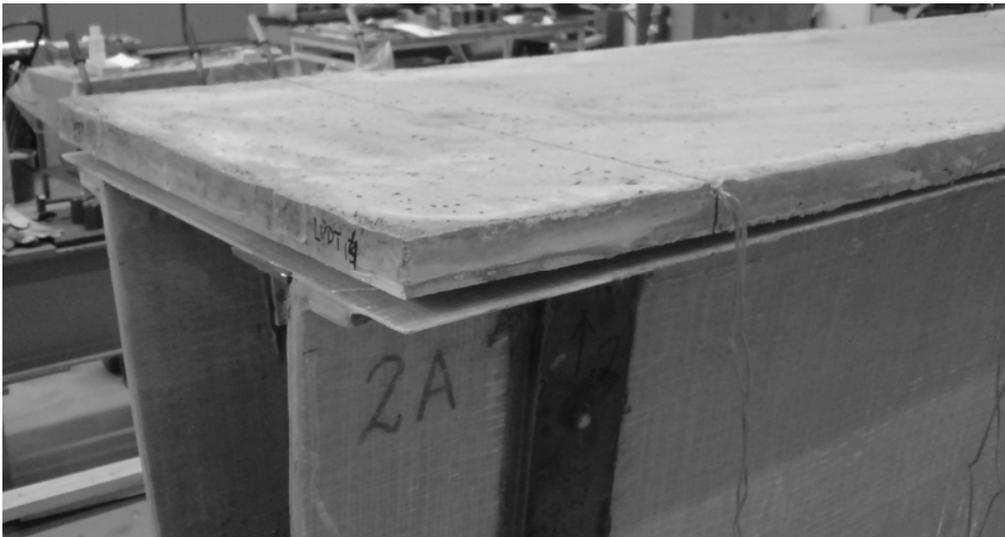
**Figure 9.** The test beam after loading to failure.
