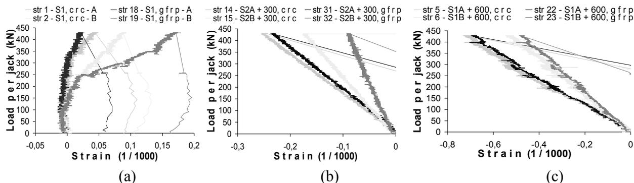
**Figure 12.** Strain measurements at the corresponding sides of the bimaterial interface in the deck for side A and side B of the beam (measured above the centre of the beam flanges) at various distances from the supports: (a) at support 1, (b) 300 mm from support 2 and (c) 600 mm from support 1.
