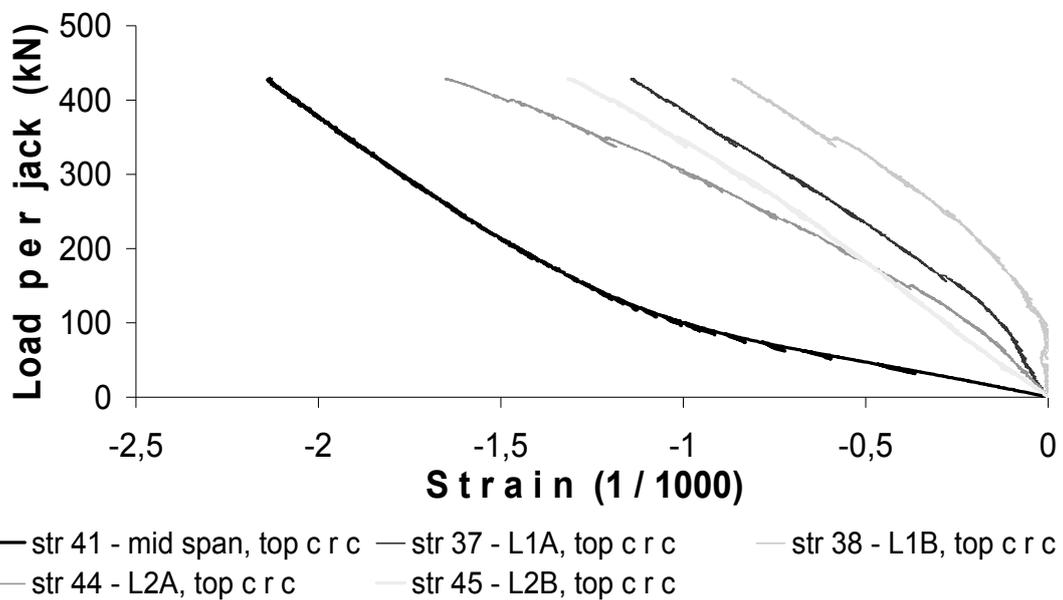
Figure 39. Strain measurements at mid-span and at the loading points for the top surface of the CRC. The mid-span strain was measured in the centre of the beam, while strains at the loading points were measured above the centre of the beam flanges on both sides just outside the load distribution device (towards the supports).
