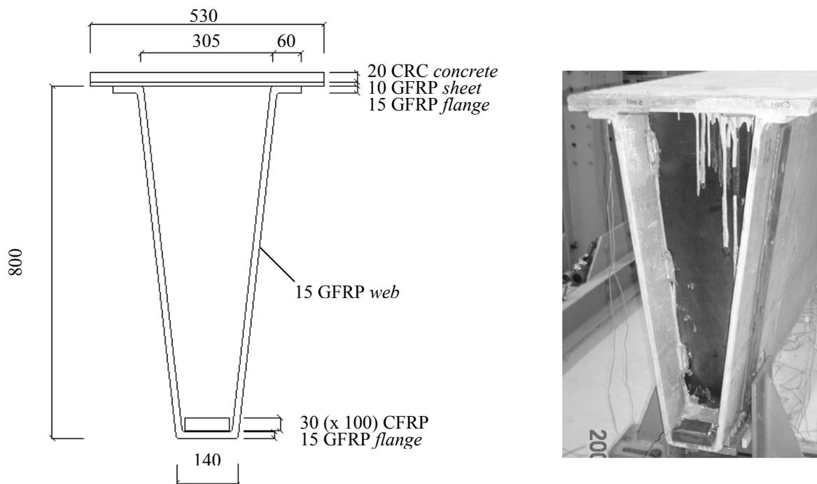
Figure 31. The cross-section of the prototype beam (to the left) and a picture showing the beam after casting of the concrete in the deck (to the right). Dimensions in mm.
