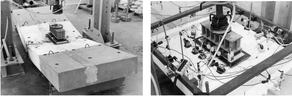
Figure 12. *At left is one of the specimens of fatigue test series UP3, after ultimate static loading to failure. At right is a close view of the set-up for the same series. The eccentric longitudinal joint and the centric loading simulating a wheel's pressure can be seen in the pictures.*
