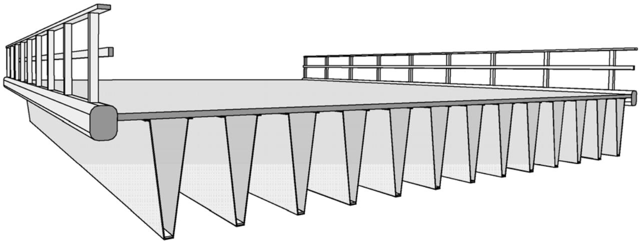
Figure 17. Outline of the *i-bridge* concept, a perspective sketch illustrating the major components of the bridge.
