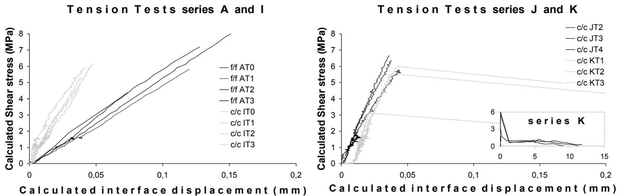
**Figure 7.** Test results for the epoxy-jointed surfaces, calculated average tension stress vs. calculated average displacement in the interface. To the left series A and I, to the right series J and K (with cut-in descending branch for K).
