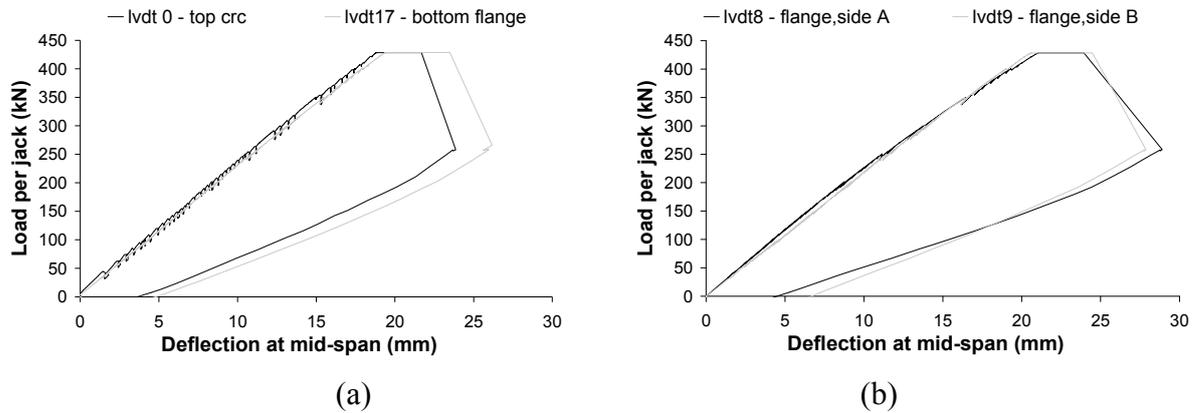
Figure 40. Load–deflection curves at mid-span; (a) for the top and bottom in the centre of the beam, and (b) for the underside of the GFRP deck sheet at the edges.
