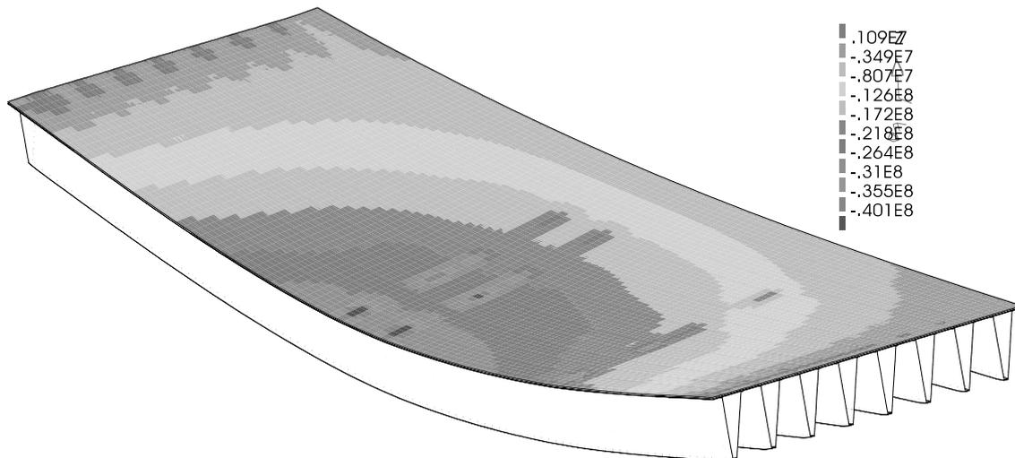
*Fig. 7: Contour plot of the CRC concrete in the bridge deck on the deformed shape from the FE analysis. Normal stresses [Pa] in the longitudinal (x) direction at full traffic load (two lanes with three axles each).*
