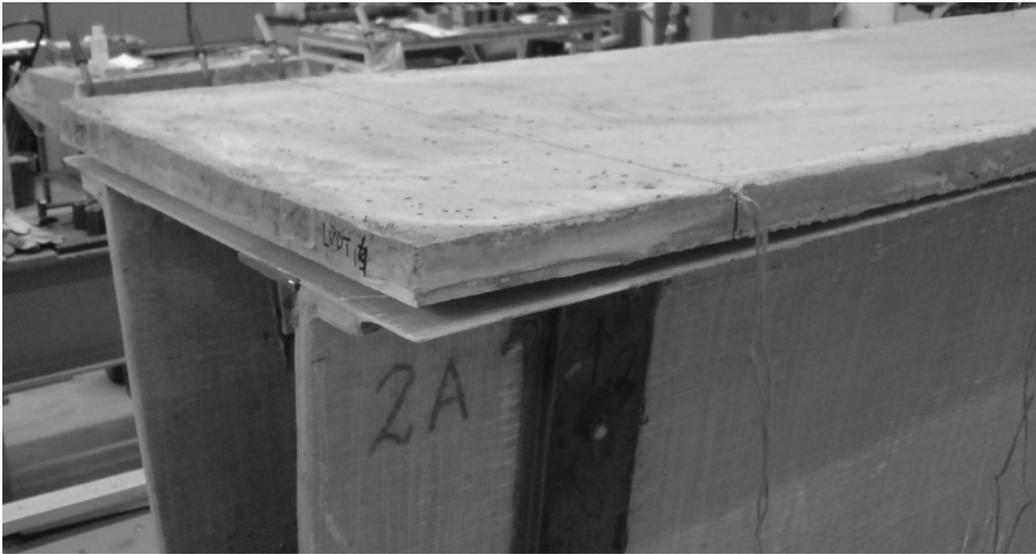
Figure 38. The test beam after loading to failure.
