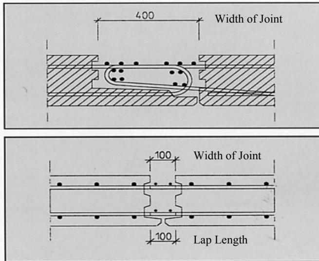
Figure 8. Comparison of joints between prefabricated deck slabs: a conventional joint (above) and the new joint (below).
