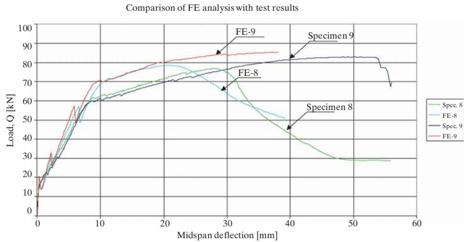
Fig. 6: Comparison of FE analysis with test results for specimens with (Specimen 9) and without (Specimen 8) transverse rebars in the joint
