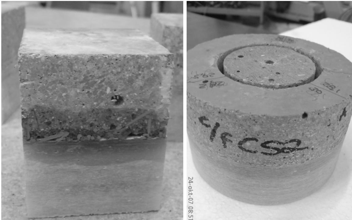
Figure 24. Test specimens before testing, to the left for shear test (test sheet F, before cutting of slots), and to the right for tension tests (test sheet C).
