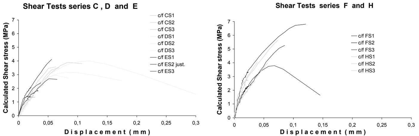
Figure 27. Test results for all interfaces between concrete and GFRP, calculated shear stress vs. displacement. To the left series C, D and E, to the right series F and H.
