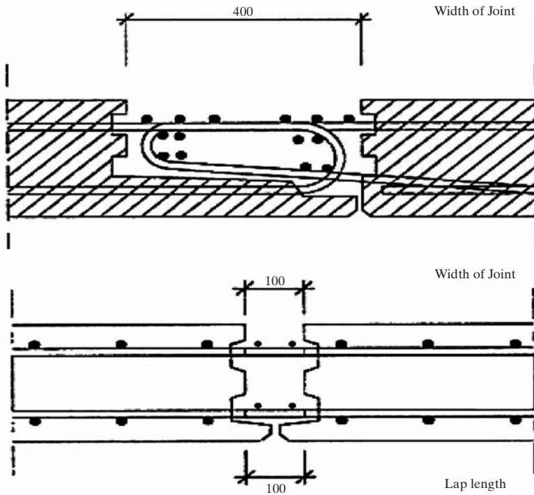
Fig. 1: Comparison of joints between prefabricated deck slabs: a conventional joint and new joint
