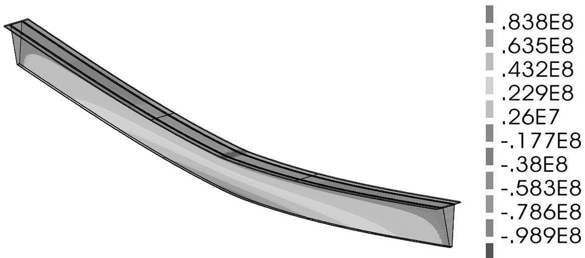
Figure 34. Contour plot of the deformed shape from FE analysis of the 25 m span full-scale bridge beam. Normal stresses [Pa] in longitudinal (x) direction at a central load of 900 kN.
