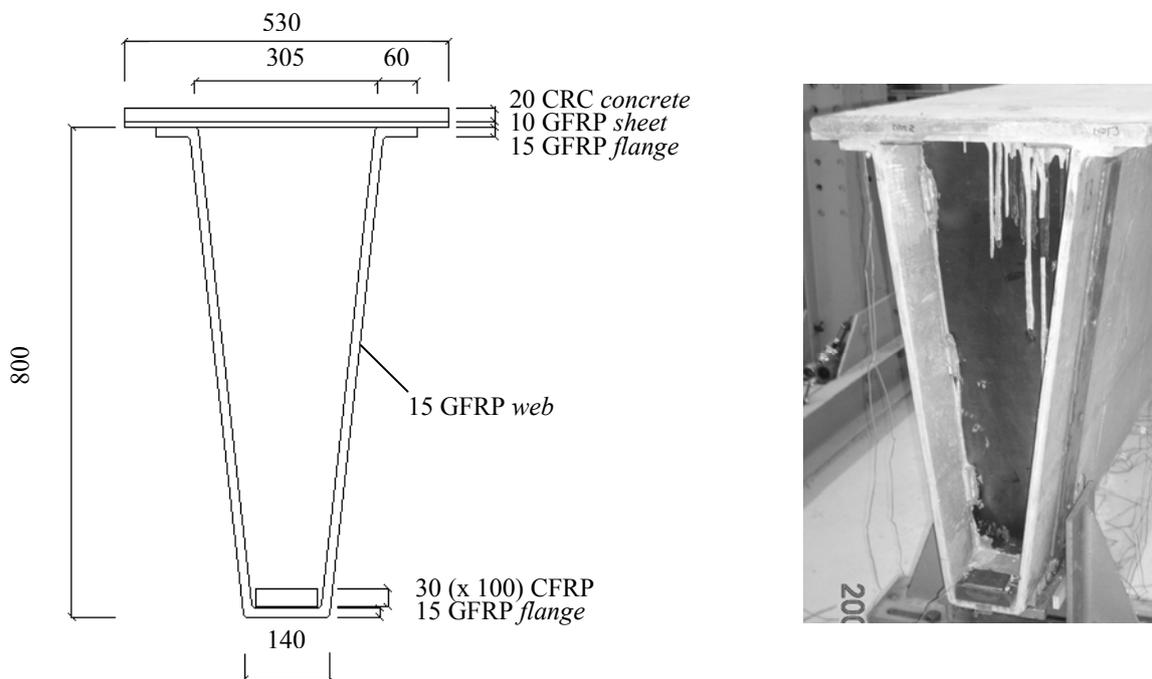
**Figure 2.** The cross-section of the prototype beam (to the left, dimensions in mm) and a picture showing the beam after casting of the concrete in the deck (to the right).
