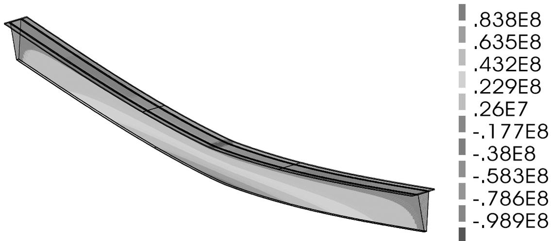
**Figure 5.** Contour plot of the deformed shape from FE analysis of the 25 m span full-scale bridge beam. Normal stresses [Pa] in longitudinal (x) direction at a central load of 900 kN.
