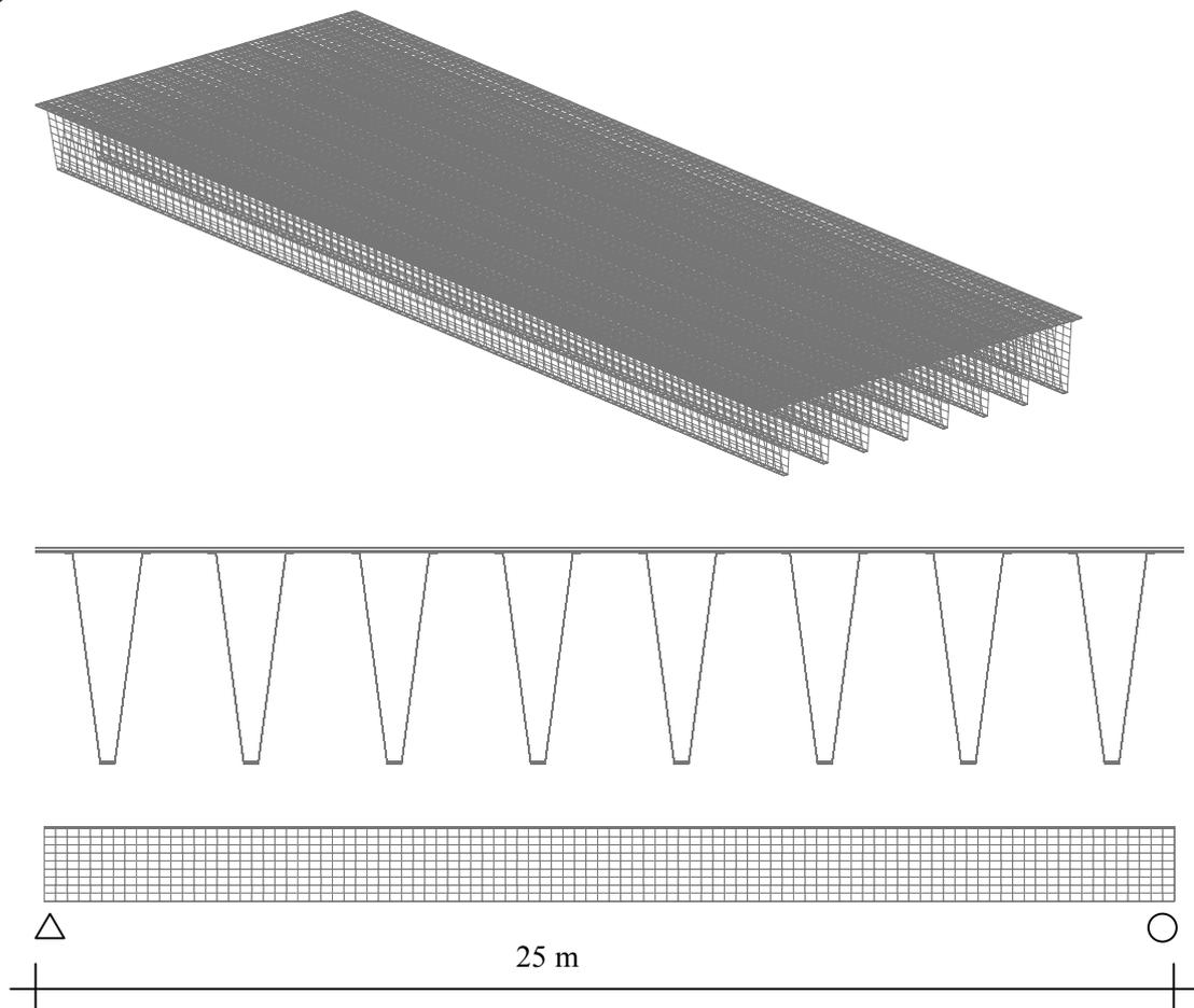
*Fig. 6: The element mesh of the global 3D model.*
