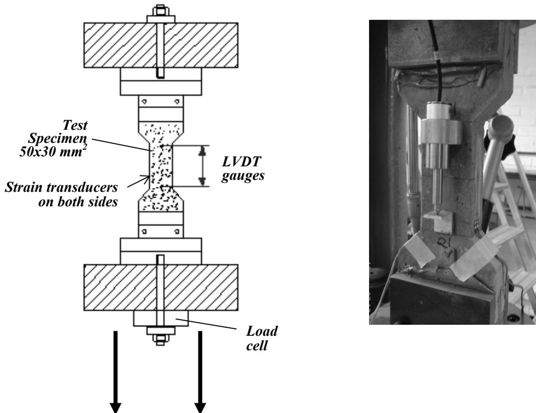
Figure 29. The principles and the set-up for the tension tests of CRC.
