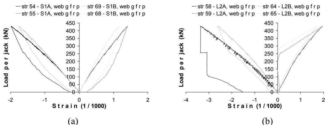
**Figure 13.** Strain measurements on the outer sides of the web surfaces in the two diagonal directions, at locations of maximum shear force: (a) at support 1 close to the bottom of the webs just outside the crossbeam, (b) at loading point 2 close to the top of the webs just outside the load distribution device.
