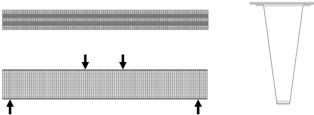
Figure 32. The mesh of the 3D FE model of the prototype beam, from above, a side view and the cross section.
