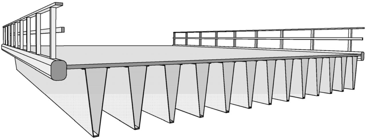
Figure 17. Outline of the *i-bridge* concept, a perspective sketch illustrating the major components of the bridge.
