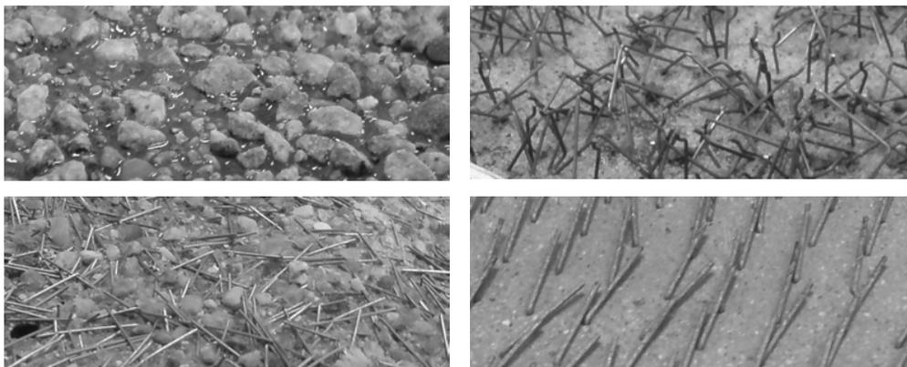
**Figure 1.** Details of some of the surfaces of the tested interfaces before casting of concrete or epoxy-gluing. Above left is surface D, above right is surface F (before removal of loose sand), below left is surface J and below right is surface K.
