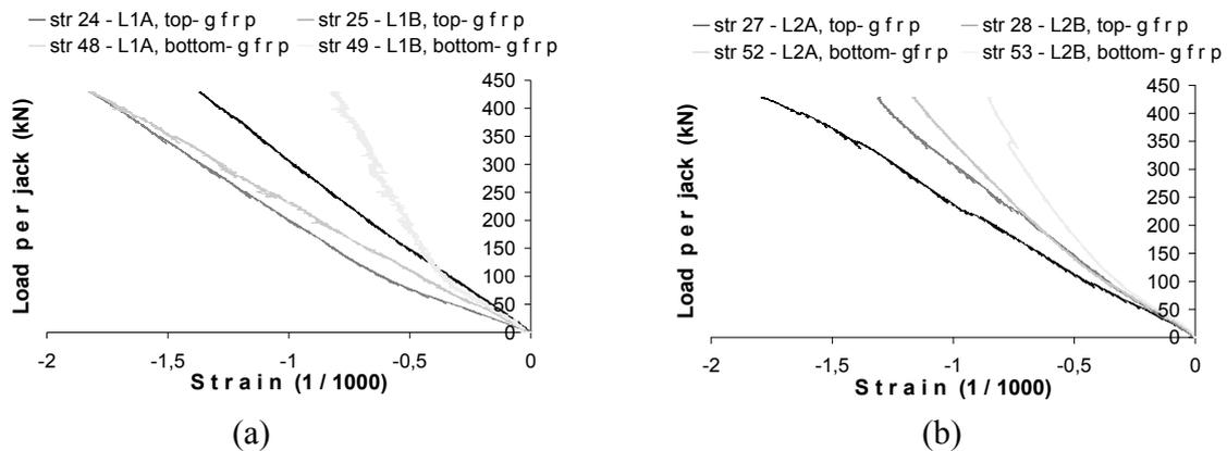
**Figure 15.** Strain measurements from the top (above centre of upper beam flanges) and bottom (just outside the edges of the beam flanges) of the GFRP deck sheet at loading points just outside the loading device (towards the supports) for beam sides A and B: (a) at loading point 1, (b) at loading point 2.
