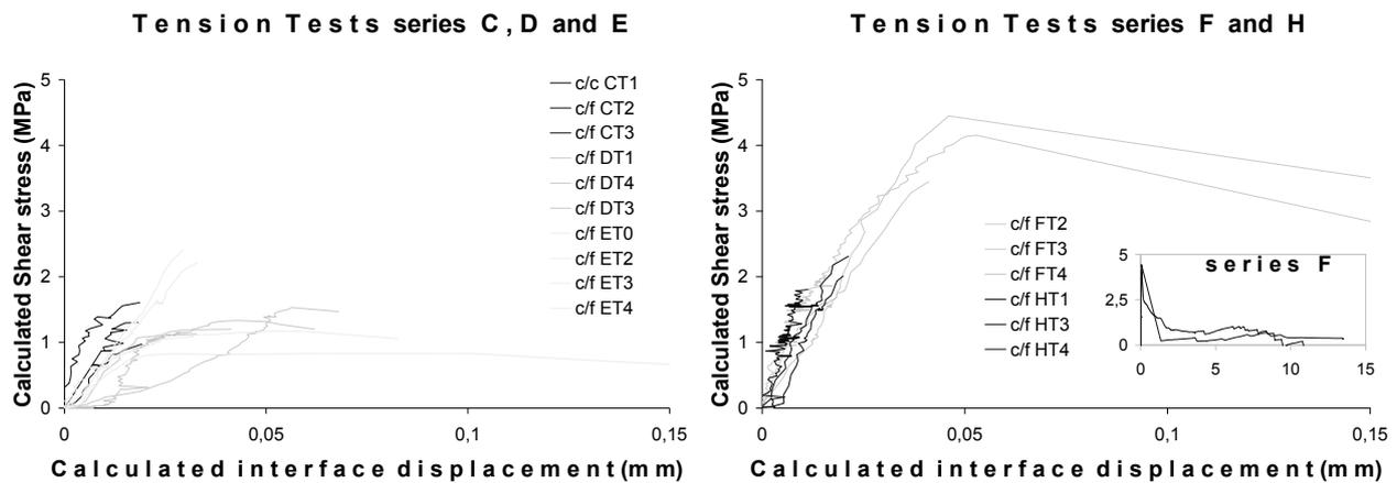
**Figure 6.** Test results for the interfaces between concrete and GFRP, calculated average tension stress vs. calculated average displacement in the interface. To the left series C, D and E, to the right series F and H (with cut-in descending branch for F).
