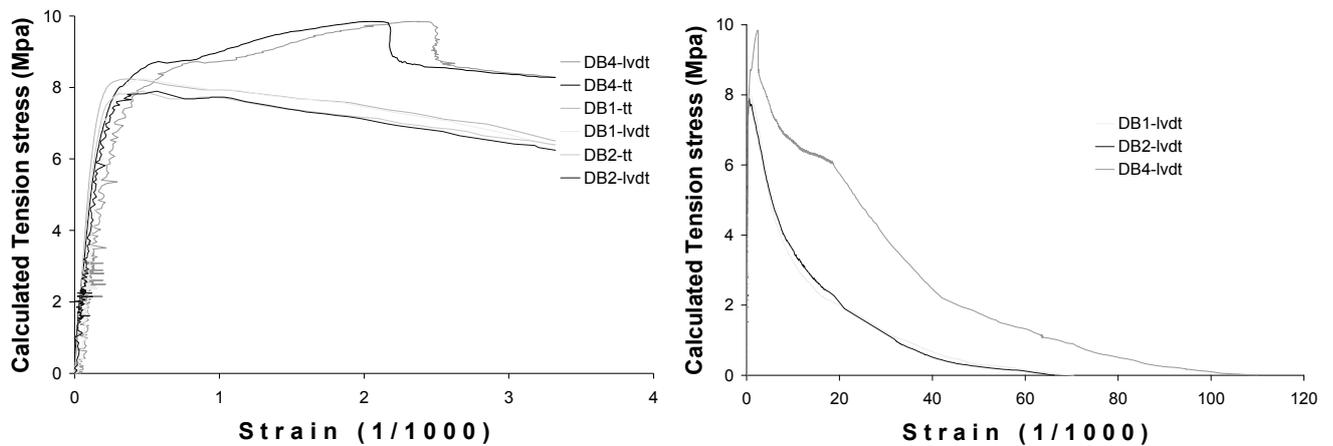
**Figure 9.** Test results for specimens DB1, DB2 and DB4, calculated tension stress vs. strain. To the left average measurements for strain gauges and LVDT gauges (calculated strain), to the right the descending branch for the LVDT gauges. Notice the different scales.
