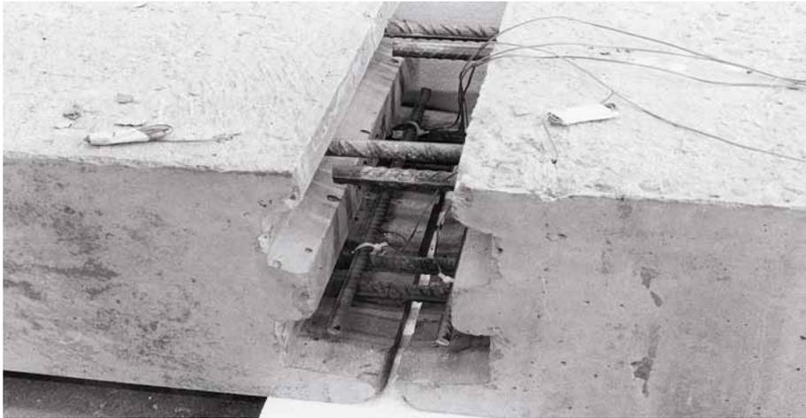
**Figure 2.** The joint before casting with the reinforcement to be spliced and the transverse bars on top.
