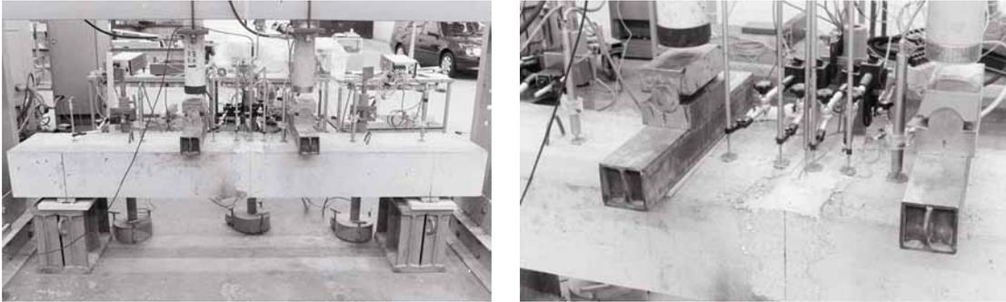
Figure 10. At left is the set-up for the static loading test. At right is a close view of the set-up. Vertical deflection was gauged by displacement transducers and strain gauges were attached to the reinforcing bars to be spliced. Essentially the same set-up was used for two of the series in the fatigue test.
