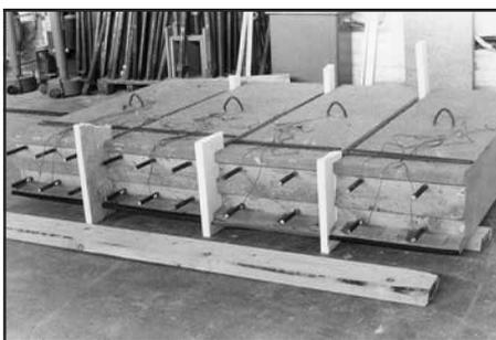
Fig. 2: Above is joint before casting with reinforcement to be spliced and transverse bars on top. Below are four halves of specimens before jointing
