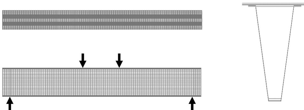
**Figure 3.** The mesh of the 3D FE model of the prototype beam, from above, a side view and the cross section.
