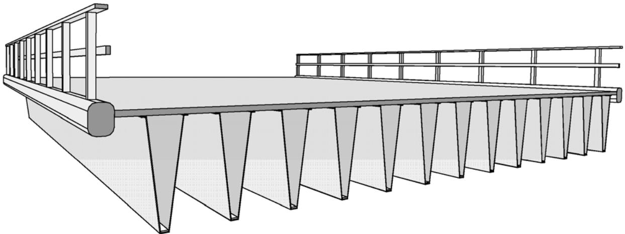
*Fig. 2: Outline of the i-bridge concept, a perspective sketch illustrating the major components of the bridge.*
