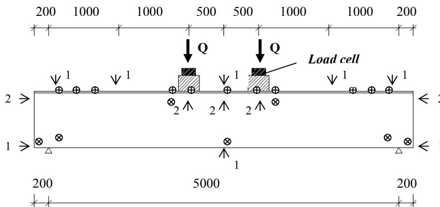
Figure 35. Set-up for the load test. Arrows denote LVDT transducers (number stands for one transducer in centre of beam and two transducers on corresponding sides respectively). Cross denote schematic placement of strain gauges (vertical cross for gauges in the deck and diagonal cross for gauges on the FRP beam).
