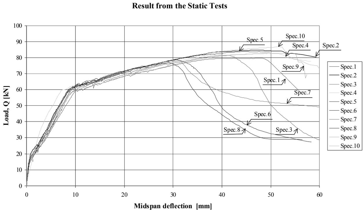
Figure 11. Load versus mid-span deflection for all specimens in the static tests.
