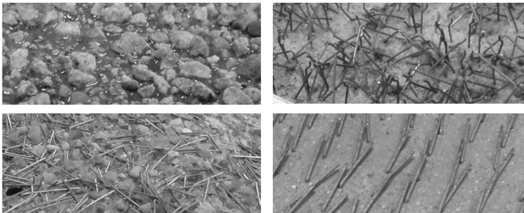
Figure 23. Some of the surfaces of the tested interfaces before casting of concrete or epoxy-gluing. Above left is surface D, above right is surface F (before removal of loose sand), below left is surface J and below right is surface K.
