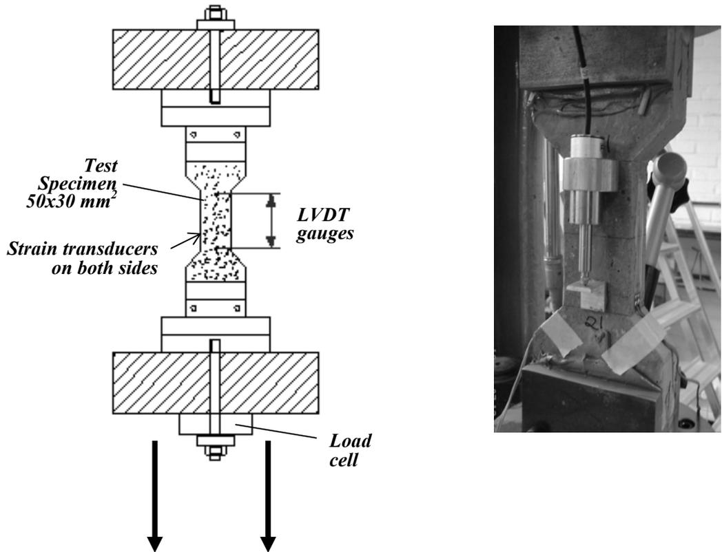
**Figure 8.** The principles and the set-up for the tension tests of CRC.
