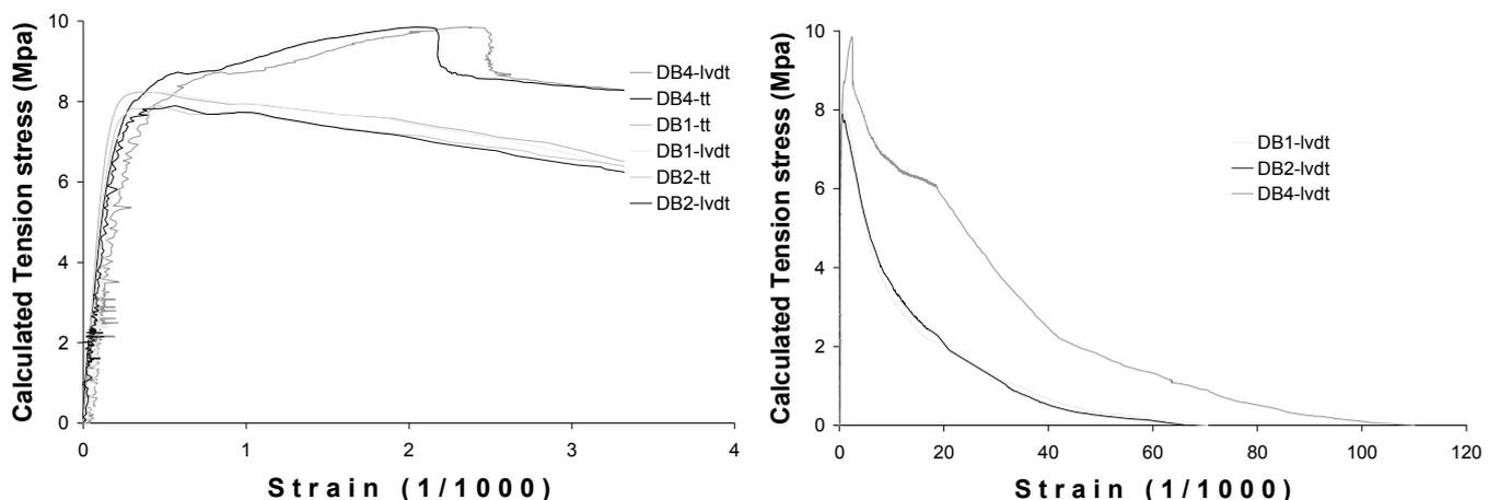
Figure 30. Test results for specimens DB1, DB2 and DB4, calculated tension stress vs. strain. To the left average measurements for strain gauges and LVDT gauges (calculated strain), to the right the descending branch for the LVDT gauges. Notice the different scales.
