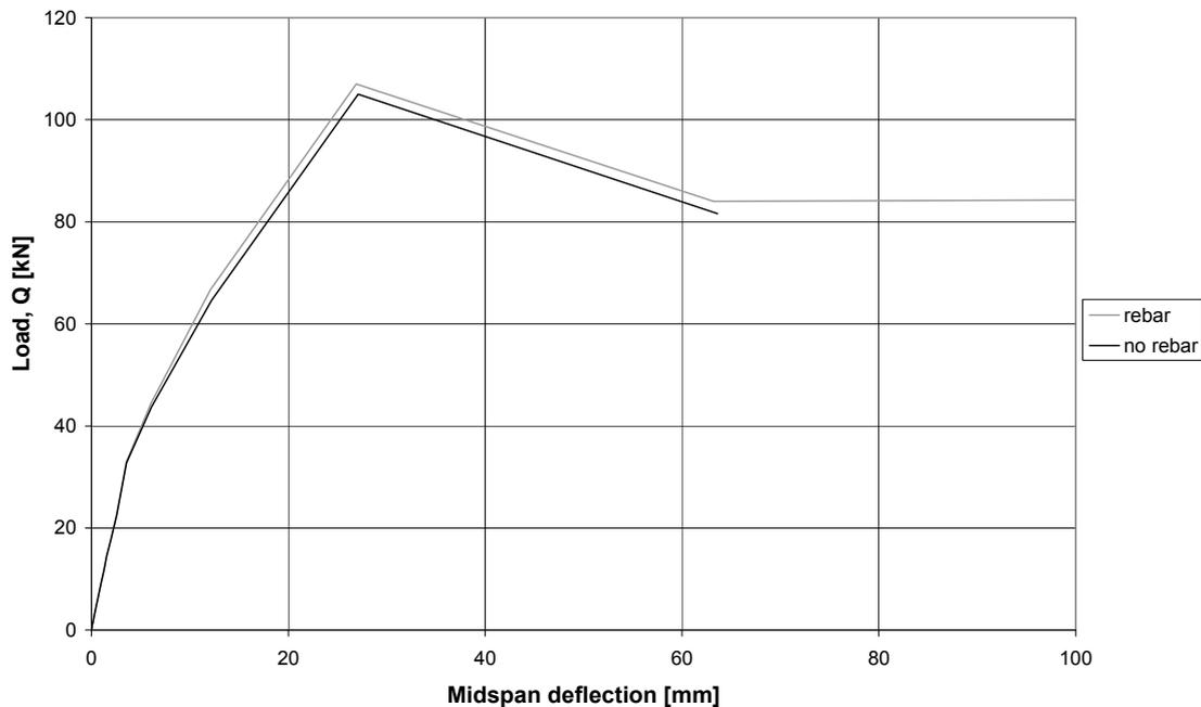
Figure 16. Results from the two FE analyses – with and without transverse rebar in the joint – for load versus mid-span deflection.
