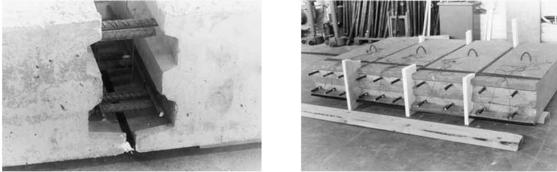
Figure 9. At left is the joint before casting, with the reinforcement to be spliced and the transverse bars on top. At the right are four halves of specimens before jointing.
