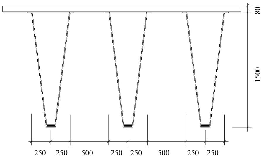
Figure 18. Major dimensions of the cross section (in mm).
