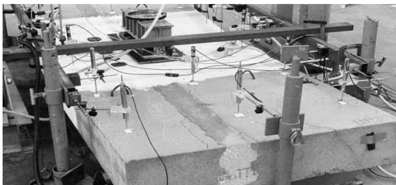
**Figure 4.** Setup for the fatigue test of series UP3, with the eccentric longitudinal joint and the centric loading simulating a wheel pressure.
