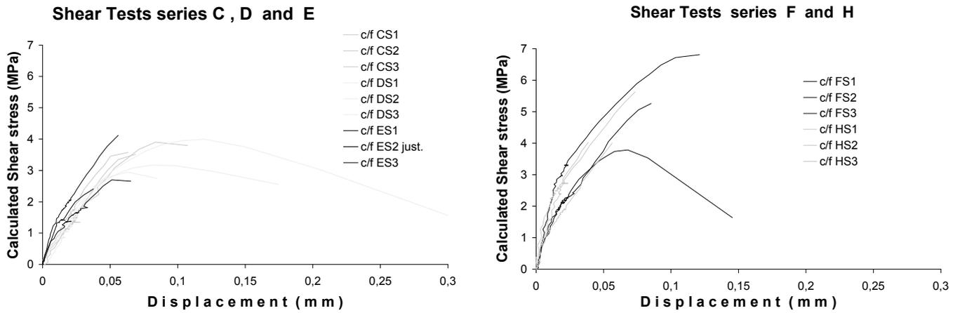
**Figure 3.** Test results for all interfaces between concrete and GFRP, calculated shear stress vs. displacement. To the left series C, D and E, to the right series F and H.
