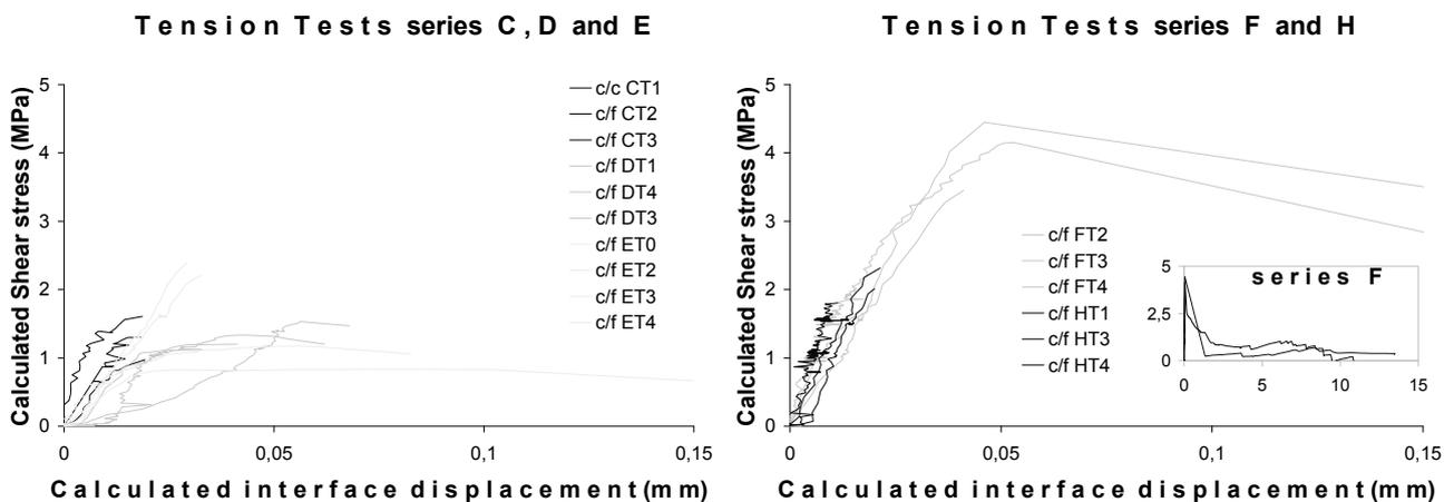
Figure 28. Test results for the interfaces between concrete and GFRP, calculated average tension stress vs. calculated average displacement in the interface. To the left series C, D and E, to the right series F and H (with cut-in descending branch for F).
