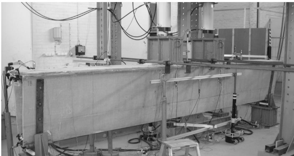
Figure 36. The prototype beam before loading.
