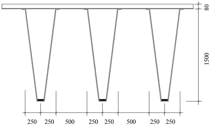
Fig. 3: Major dimensions of the cross section (in mm).
