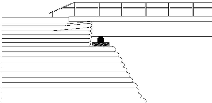
*Fig. 5: An elevation showing principles for the proposed foundation and substructure of the bridge.*
