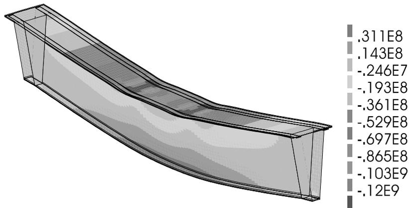
Figure 33. Contour plot of the deformed shape from FE analysis of the 5 m span prototype beam. Normal stresses [Pa] in longitudinal (x) direction at a load of 2 x 430 kN (placement of load according to Figure 35).
