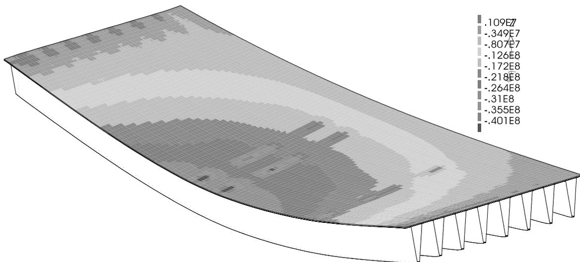
Figure 22. Contour plot of the CRC concrete in the bridge deck on the deformed shape from the FE analysis. Normal stresses [Pa] in the longitudinal (x) direction at full traffic load (two lanes with three axles each).
