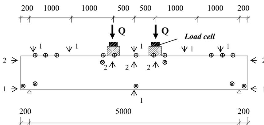
**Figure 6.** Set-up for the load test. Arrows denote LVDT transducers (number stands for one transducer in centre of beam and two transducers on corresponding sides respectively). Cross denote schematic placement of strain gauges (vertical cross for gauges in the deck and diagonal cross for gauges on the FRP beam).
