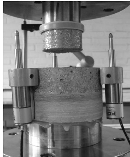
**Figure 5.** Test principles and the set-up for the tension tests (after loading).
