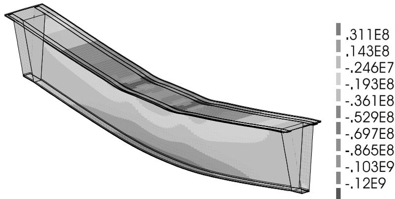
**Figure 4.** Contour plot of the deformed shape from FE analysis of the 5 m span prototype beam. Normal stresses [Pa] in longitudinal (x) direction at a load of  $2 \times 430$  kN.
