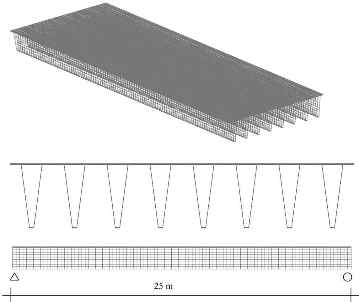
*Figure 21. The element mesh of the global 3D model.*
