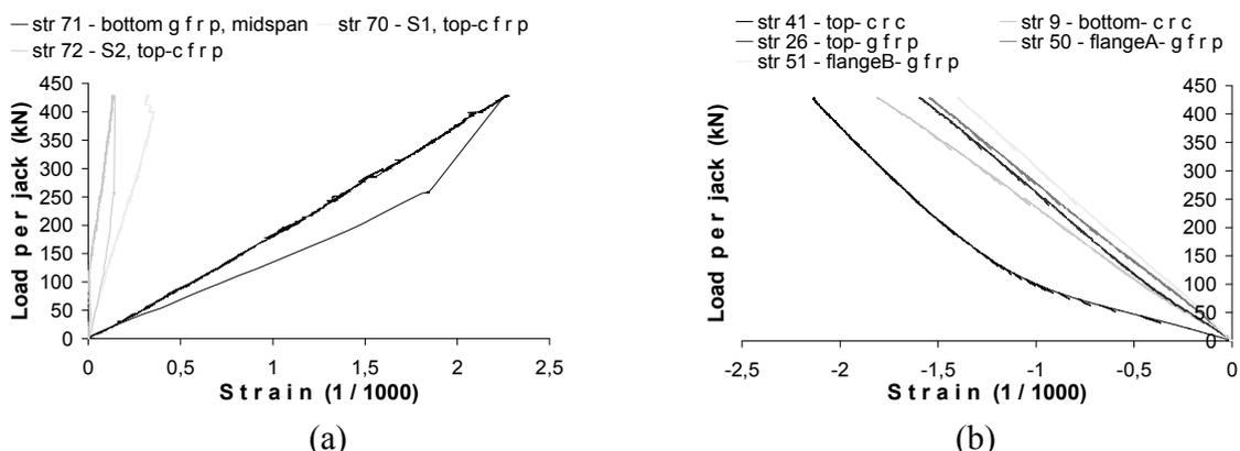
**Figure 14.** Strain measurements: (a) for bottom flange of GFRP at mid-span and top of CFRP on the protruding part just outside the crossbeam, and (b) at mid-span for top and bottom of CRC and top of GFRP deck sheet in the centre of the beam along with undersides of the GFRP deck sheet close to the edges.
