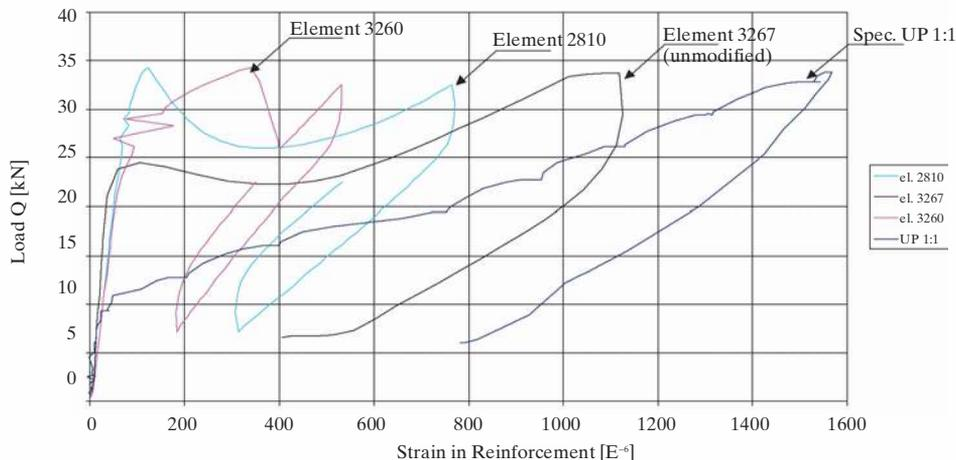
Fig. 8: Comparison of steel strains from analysis of the modified and unmodified FE models with measured values
