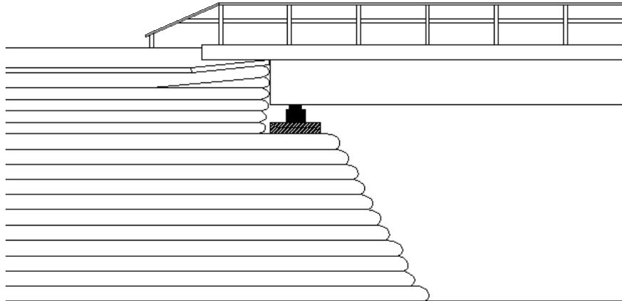
Figure 20. Elevation showing principles for the proposed foundation and substructure of the bridge.
