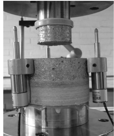
Figure 26. Test principles and the set-up for the tension tests (to the right after testing).
