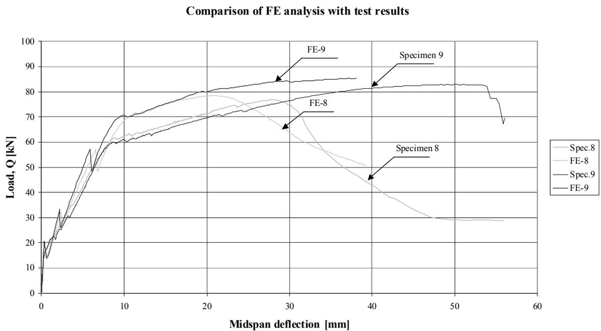
Figure 14. Comparison of 2D FE analysis with test results for specimens with (specimen 9) and without (specimen 8) transverse rebars in the joint.
