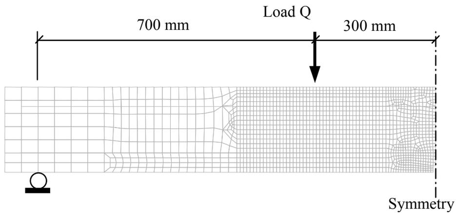
Figure 13. The mesh of the 2D FE model.
