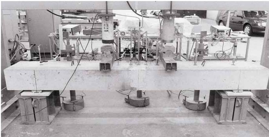
**Figure 3.** Setup for the static loading test. The loading is a symmetric two point load. The specimens span 2000 mm and the space between the loading points is 600 mm. Principally the same setup is used for series UP1 and UP2 in the fatigue test.
