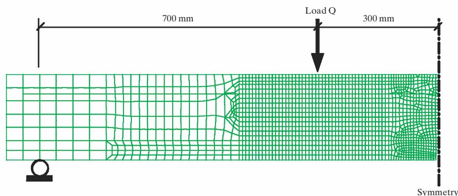
Fig. 5: The mesh of FE model
