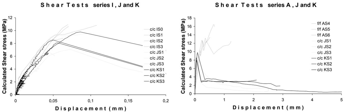
**Figure 4.** Test results for all epoxy-jointed surfaces, calculated shear stress vs. displacement. To the left series I, J and K, to the right series A, J and K. Notice the different scales.
