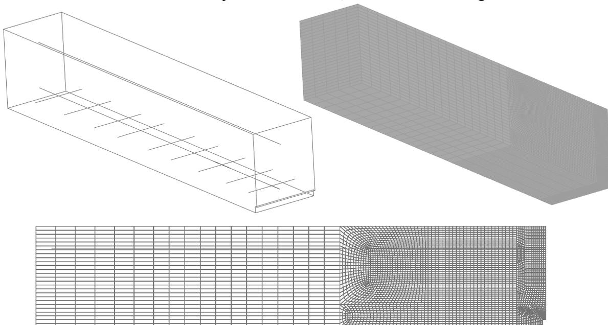
*Figure 15. The mesh of the 3D FE model, at top left an outline with the rebars, at top right the “hidden sides” and at bottom a side view. Load and supports etc. are the same as in Figure 13.*
