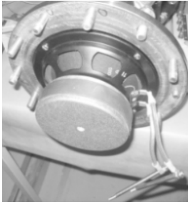
Figure 4.3: The driver is mounted to the resonator and the box is then mounted separately over the back of the loudspeaker. The cable passage through the loudspeaker box has to be gastight. A copper block passes through the wall of the box, wires connect the block on the inside to the loudspeaker and on the outside to the amplifier.
