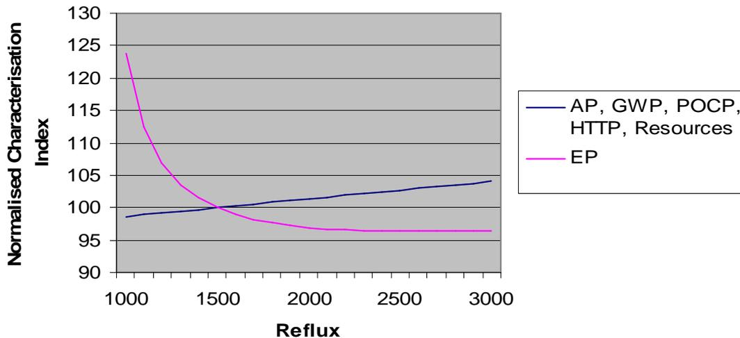
**Figure 7.** Normalised (reference reflux is 1500 kg/h) characterisation indexes as a function of reflux. Characterisation indicators from CML (2002) were used.
