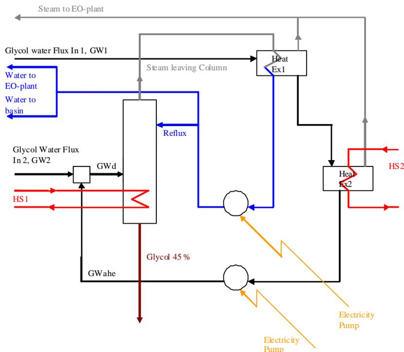
**Figure 5.** Flowchart of distillation system. This is also the foreground system of the eco-efficiency study.
