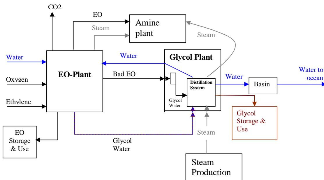
**Figure 3.** The ethylene amine plant at Site Stenungsund, which also is the operational environment of the glycol plant. Only flows relevant for this study are shown.
