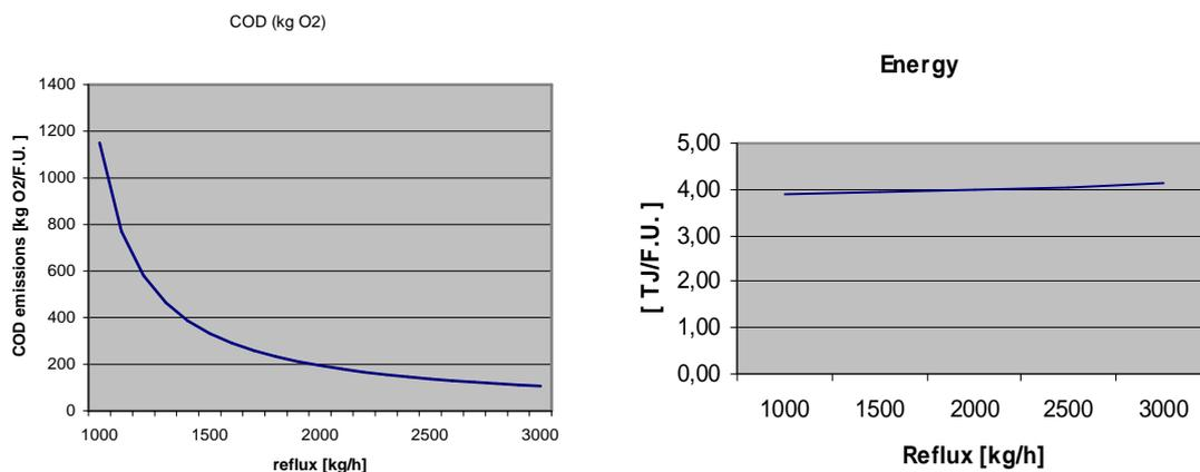
**Figure 6.** Emissions of COD to water and energy consumed by the distillation system, as functions of the reflux to the distillation column.
