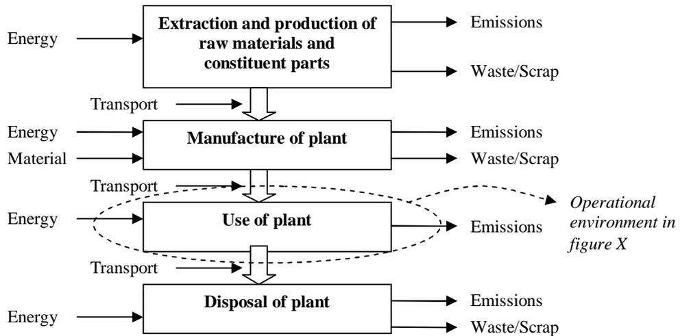
**Figure 4.** Lifecycle of the glycol water treatment plant
