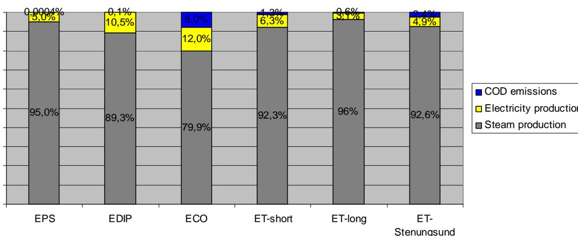
**Figure 8.** Contribution to the total environmental load of COD emissions, electricity production and steam production. Reflux is 1500 kg/h.
