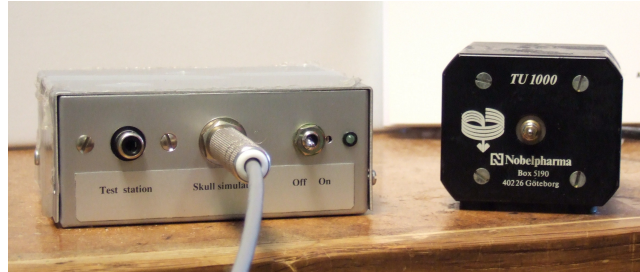
Figure 4. The skullsimulator TU-1000 to the right and its power supply unit to the left.
