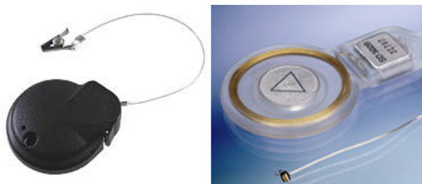
Figure 15. To the left is the audio processor, AP, with a microphone and a transmitting coil. To the right are the receiver coil and the envelope detector. The two coils are together called the inductive link. Below the receiver coil is the floating mass transducer can be seen, which in this thesis is replaced with a BEST [ 10].
