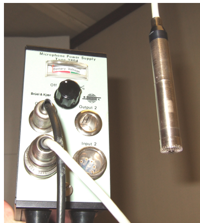
Figure 5. The condenser microphone with its power supply.
