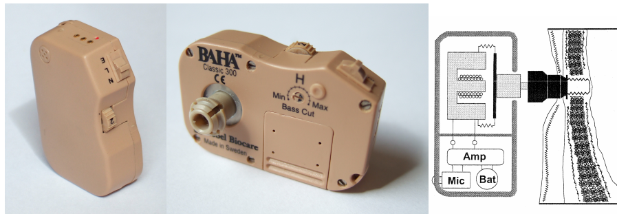
Figure 11. The BAHA Classic 300 system. In the left picture the front side of the BAHA is shown, in the middle picture the back side with the snap coupling and in the right figure [ 7] the generic design of the percutaneous system.
