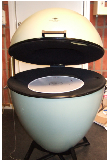
Figure 7. Brüel & Kjær Anechoic Test Chamber Type 4222.
