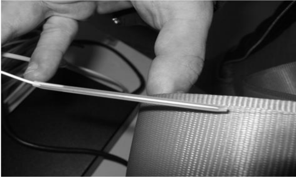
Figure 18. The welded patch cable and free fiber end from the safety belt.
