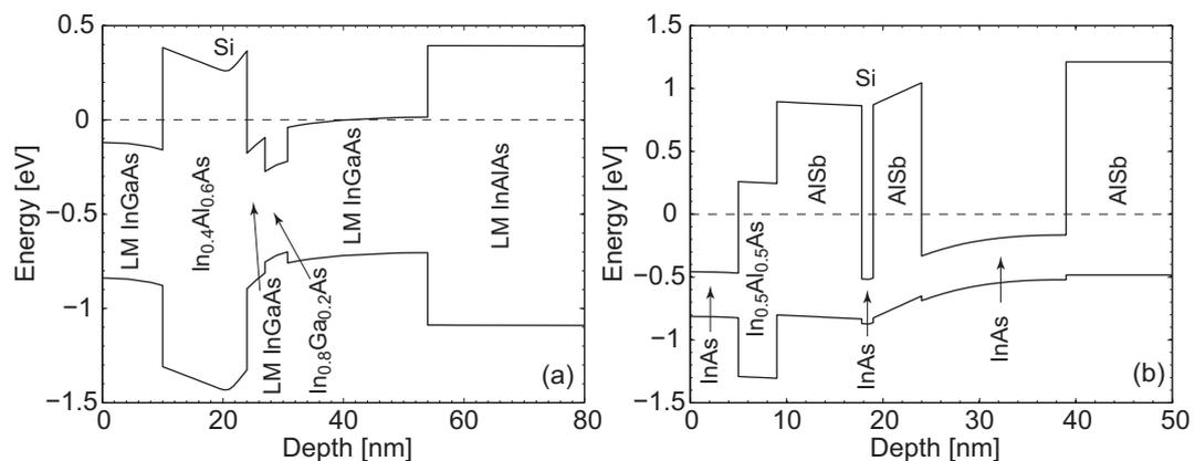
**Figure 3.1** TCAD simulated energy-band diagrams at thermal equilibrium and 300 K for (a) an InGaAs/InAlAs HEMT (LM = lattice-matched to InP) and (b) an InAs/AlSb HEMT.
