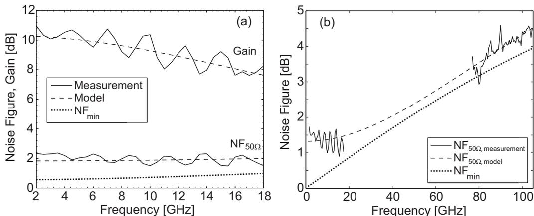
**Figure 4.6** Measured and modeled noise for  $2 \times 50 \mu\text{m}$  gate width (a) 225 nm gate-length InAs/AlSb HEMT and (b) 130 nm gate-length InGaAs/InAlAs HEMT.
