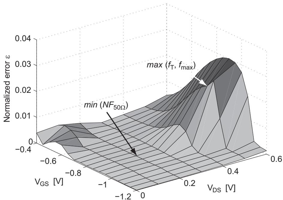
**Figure 4.3** Normalized error of the extracted  $S$ -parameters versus bias for a  $2 \times 50 \mu\text{m}$  gate-width InAs/AlSb HEMT.  $\max(f_T, f_{\max})$  and  $\min(NF_{50\Omega})$  are the  $\varepsilon$  corresponding to the bias points in Figure 4.2.
