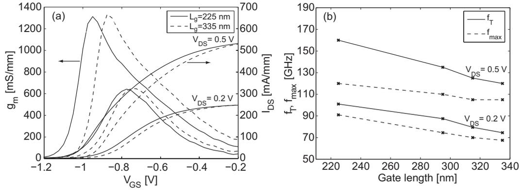
**Figure 5.1** Influence of  $L_g$  on (a)  $g_m$  and  $I_{DS}$  as a function of  $V_{GS}$  and (b)  $f_T$  and  $f_{max}$  for a  $2 \times 50 \mu\text{m}$  gate-width InAs/AlSb HEMT biased at  $V_{DS} = 0.2$  V and  $V_{DS} = 0.5$  V.
