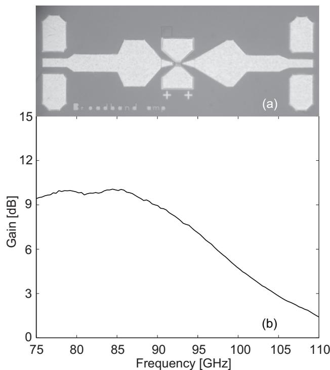
**Figure 8.2** (a) A photograph and (b) measured gain of a 94 GHz amplifier based on a 70 nm gate-length InGaAs/InAlAs HEMT technology. Chip size  $1.7 \text{ mm} \times 0.5 \text{ mm}$ .
