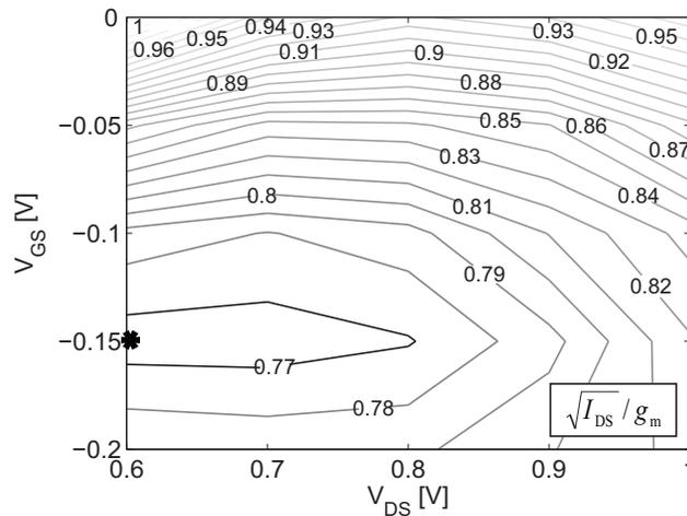
**Figure 3.12** Estimation of the bias point corresponding to minimum NF. The bias point corresponding to the measured  $NF_{50\Omega}$  is marked with a star (\*).
