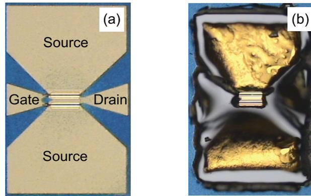
**Figure 3.4** Optical microscope pictures of an InAs/AlSb HEMT (a) with and (b) without AlSb oxidation, caused by different mesa-etch depths.
