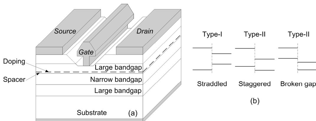
**Figure 2.1** Schematics of (a) the HEMT structure and (b) the different heterostructure energy band alignments: straddled (type-I), staggered and broken gap (type-II).
