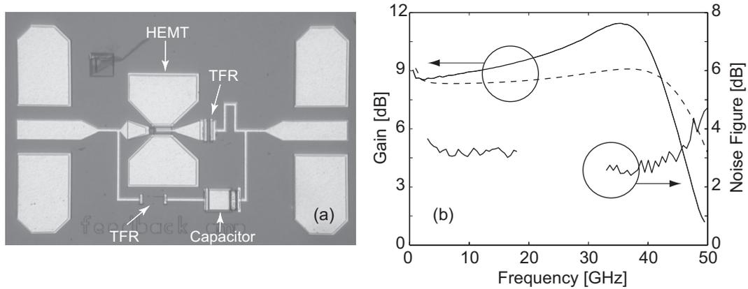
**Figure 8.1** A 0-42 GHz broadband MMIC amplifier based on a 50 nm gate-length InGaAs/InAlAs HEMT technology. (a) photograph of the amplifier with a chip size of  $0.9 \text{ mm} \times 0.6 \text{ mm}$  and (b) measured (solid) and modeled (dashed) gain, and measured noise figure (solid) for the amplifier at  $V_{DS} = 1.0 \text{ V}$  and  $V_{GS} = -0.2 \text{ V}$ .
