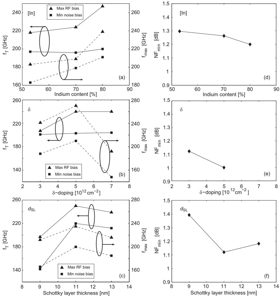
**Figure 6.3** Extrinsic  $f_T$ ,  $f_{\text{max}}$  for maximum RF and lowest noise bias, and  $NF_{\text{min}}$  (@ 26 GHz) versus [In],  $\delta$  and  $d_{\text{SL}}$ , for 130 nm gate-length InGaAs/InAlAs HEMTs.
