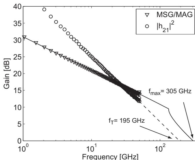
**Figure 3.10** Extraction of  $f_T$  and  $f_{max}$  for a 130 nm gate-length InGaAs/InAlAs HEMT through extrapolation from measured S-parameters.
