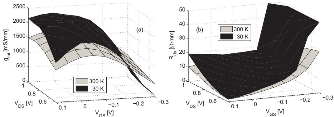
**Figure 4.5** (a)  $g_{mi}(V_{GS}, V_{DS})$  and (b)  $R_{ds}(V_{GS}, V_{DS})$  at 300 K and 30 K of an InGaAs/InAlAs HEMT.
