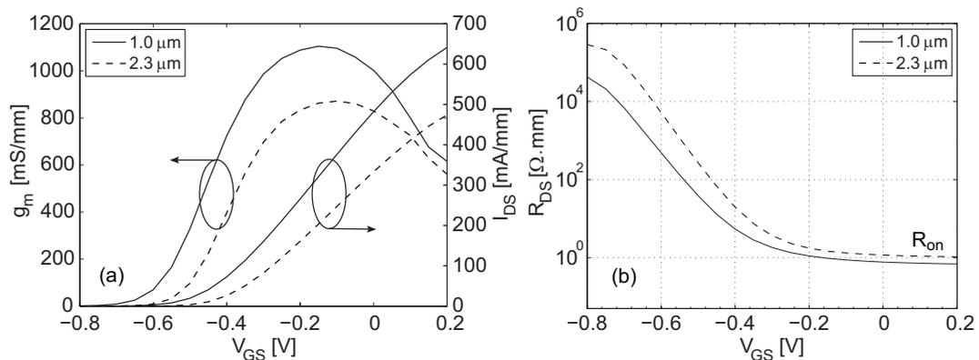
**Figure 5.3** Influence of source-to-drain distance  $L_{\text{SD}}$  on (a)  $g_m(V_{\text{GS}})$ ,  $I_{\text{DS}}(V_{\text{GS}})$  at  $V_{\text{DS}} = 1.0 \text{ V}$  and (b)  $R_{\text{DS}}(V_{\text{GS}})$  at  $V_{\text{DS}} = 50 \text{ mV}$  for InGaAs/InAlAs HEMTs.
