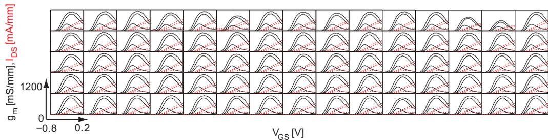
**Figure 3.7**  $I_{DS}(V_{GS})$  and  $g_m(V_{GS})$  at  $V_{DS} = 0.3, 0.7$  and  $1.0$  V of 75 InGaAs/InAlAs HEMTs (from the upper right quarter of Figure 3.6(a)).
