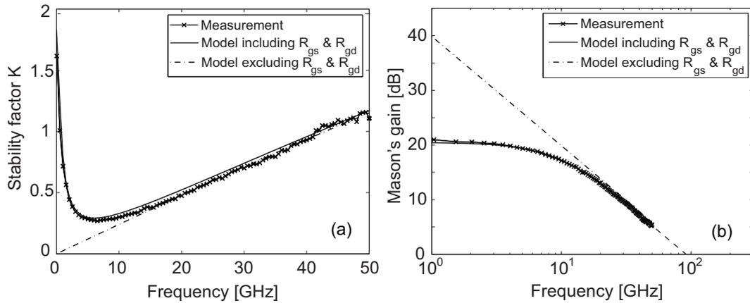
**Figure 4.4** Measured and modeled (a)  $K$ -factor and (b) Mason's gain for an InAs/AlSb HEMT.
