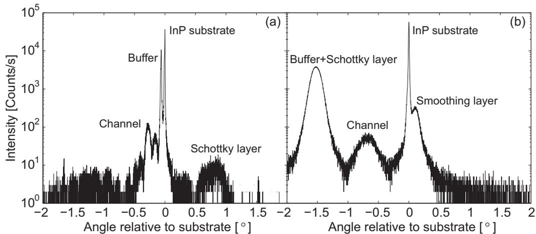
**Figure 3.2** X-ray diffraction measurement on the (004) plane of (a) an InGaAs/InAlAs HEMT and (b) an InAs/AlSb HEMT. Both measured results were normalized to the InP substrate.
