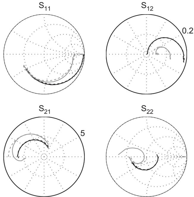
**Figure 4.2** Measured (solid) and modeled (dashed)  $S$ -parameters for a  $2 \times 50 \mu\text{m}$  gate-width InAs/AlSb HEMT biased for either low noise (black) or high frequency (grey) operation.
