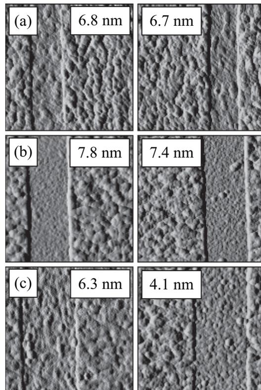
**Figure 7.2**  $1\ \mu\text{m} \times 1\ \mu\text{m}$  AFM images of the gate recess evolution of InAs/AlSb HEMTs, two days (left column) and two weeks (right column) after the recess etch as a function of recess depth. Recess down to (a) 3D grown InAlAs, (b) 2D grown InAlAs and (c) AlSb Schottky layer.
