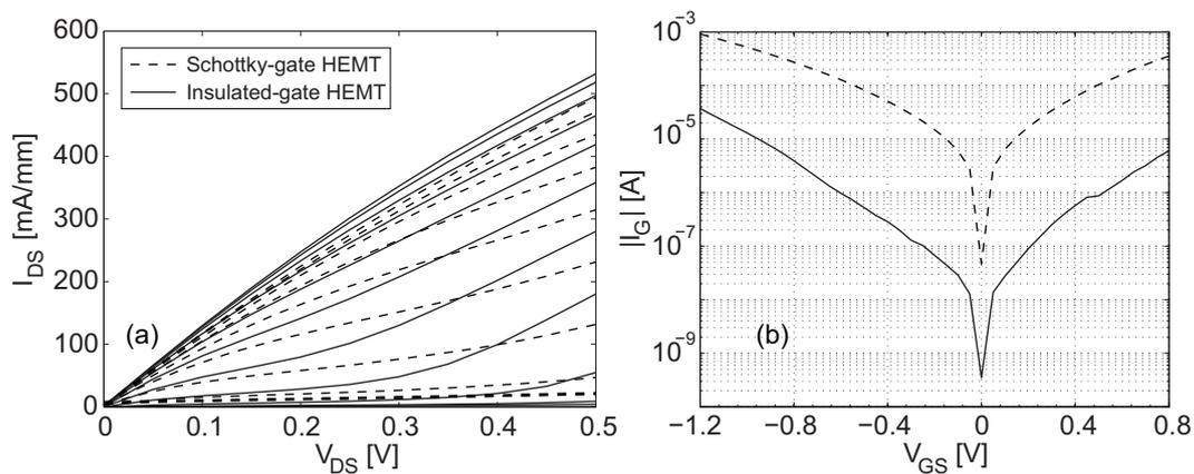
**Figure 7.3** DC performance of Schottky-gate InAs/AlSb HEMT versus insulated-gate InAs/AlSb HEMT. (a)  $I$ - $V$  output characteristics at  $V_{GS}$ : -1.2 V to -0.2 V in steps of 0.1 V and (b) diode characteristics at  $V_{DS} = 0$  V.
