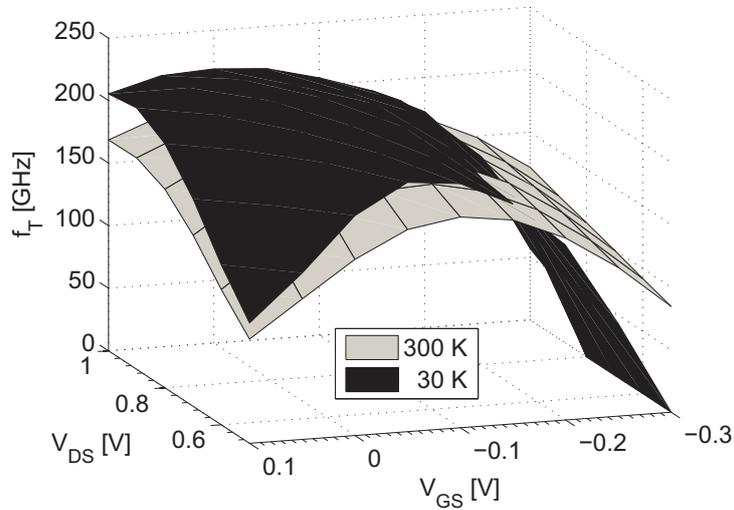
**Figure 3.14** Extrinsic  $f_T(V_{GS}, V_{DS})$  at 300 K and 30 K for an InGaAs/InAlAs HEMT.
