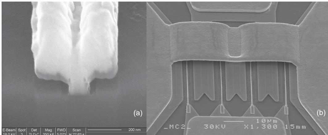
**Figure 3.5** (a) FIB-SEM cross-section image of a gate and (b) SEM image of an InGaAs/InAlAs HEMT.
