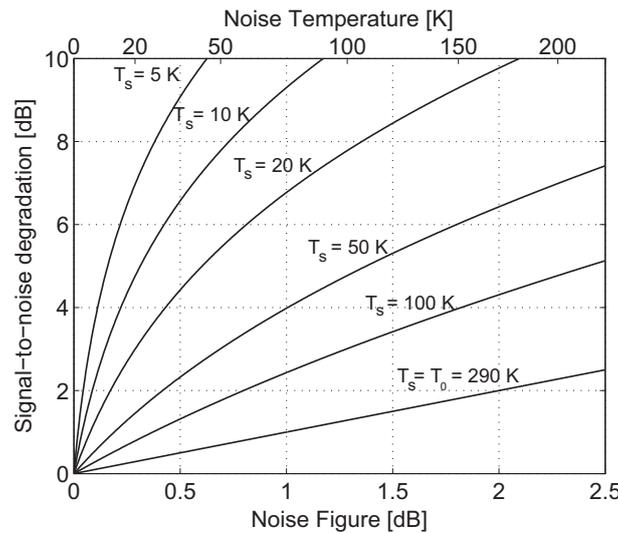
**Figure 2.3** Signal-to-noise degradation as a function of the device noise figure  $NF$  (and equivalent noise temperature  $T_e$ ) with different source temperatures.  $T_s = 290$  K corresponds to the definition of  $NF$ .
