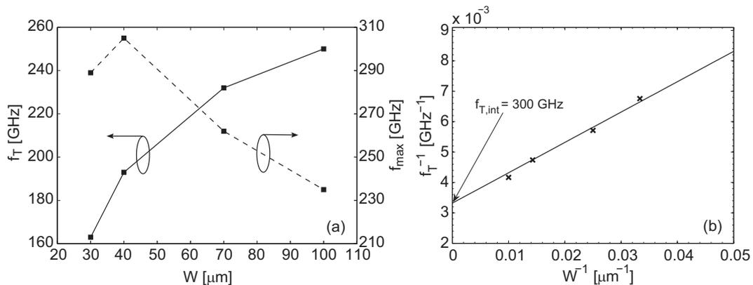
**Figure 5.4** Influence of the gate-width  $W$  on (a) extrinsic  $f_T$  and  $f_{max}$  and (b) the corresponding intrinsic  $f_T$  value extraction for InGaAs/InAlAs HEMTs.
