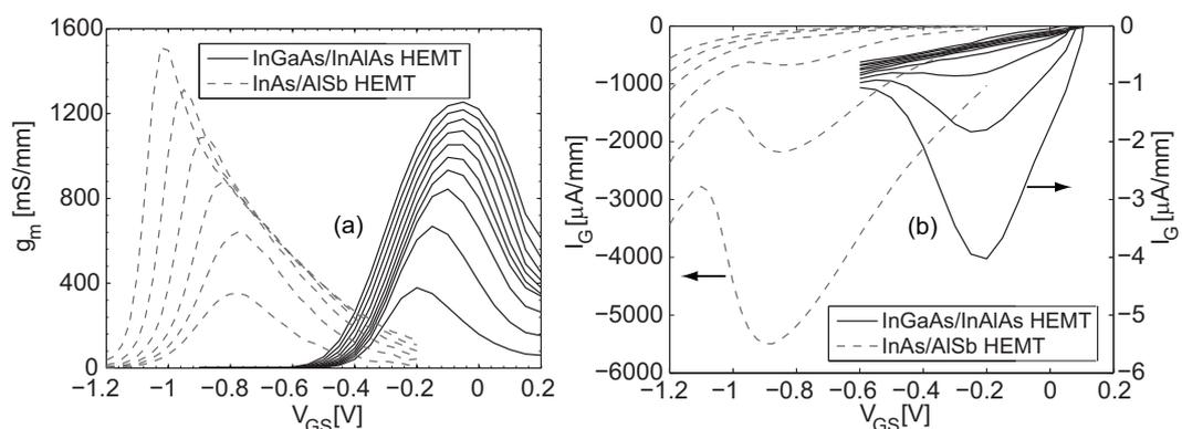
**Figure 3.8** DC characteristics of 225 nm gate-length InAs/AlSb HEMTs (dashed) at  $V_{DS}$ : 0.1 V to 0.6 V, and 130 nm gate-length InGaAs/InAlAs HEMTs (solid) at  $V_{DS}$ : 0.1 V to 1.0 V, in steps of 0.1 V. (a)  $g_m(V_{GS})$  and (b)  $I_G(V_{GS})$ . Note the factor 1000 difference in the y-scale in (b).
