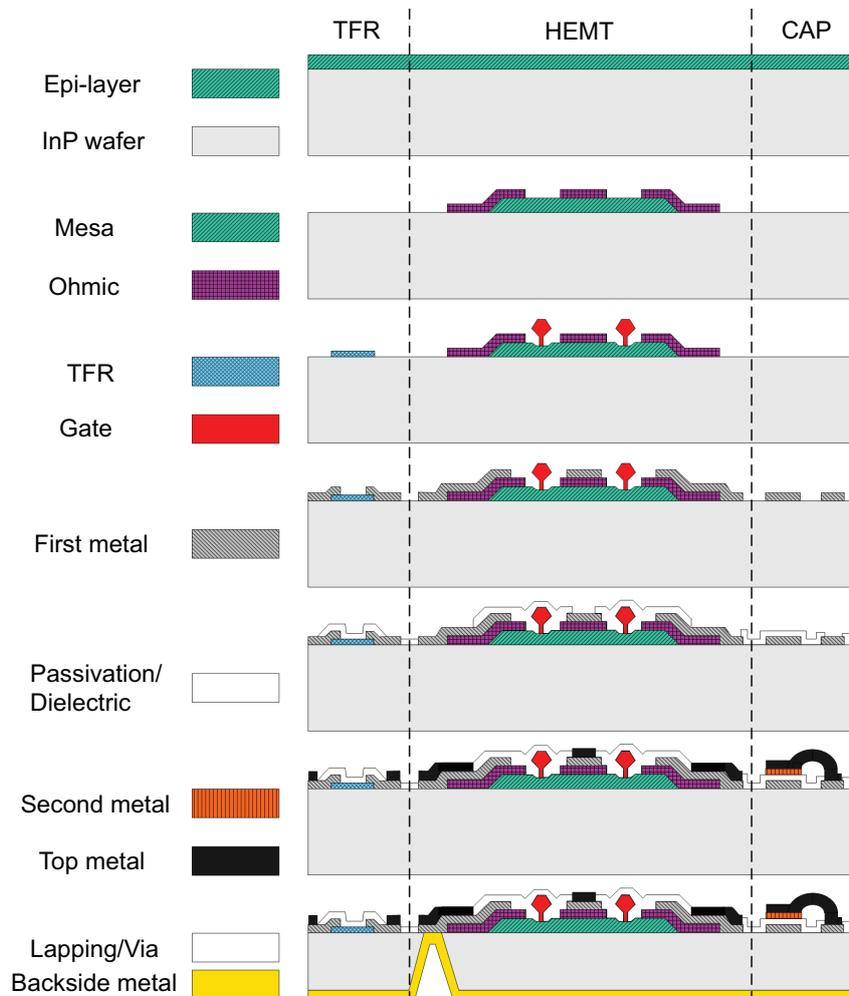
**Figure 3.3** MMIC process sequence for the investigated narrow bandgap technologies, including a HEMT, a thin-film resistor (TFR) and a capacitor (CAP).
