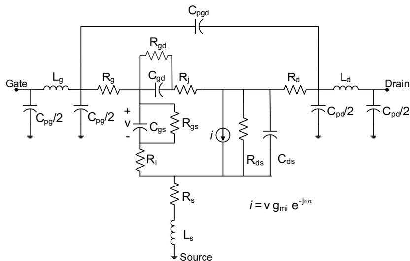
**Figure 4.1** Small-signal model of the narrow bandgap HEMT.
