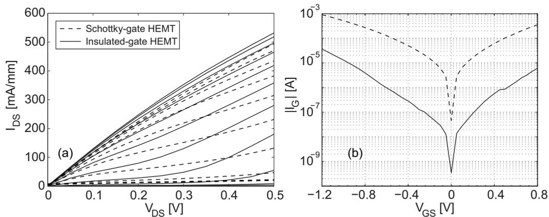
**Figure 7.3** DC performance of Schottky-gate InAs/AlSb HEMT versus insulated-gate InAs/AlSb HEMT. (a)  $I$ - $V$  output characteristics at  $V_{GS}$ :  $-1.2$  V to  $-0.2$  V in steps of  $0.1$  V and (b) diode characteristics at  $V_{DS} = 0$  V.
