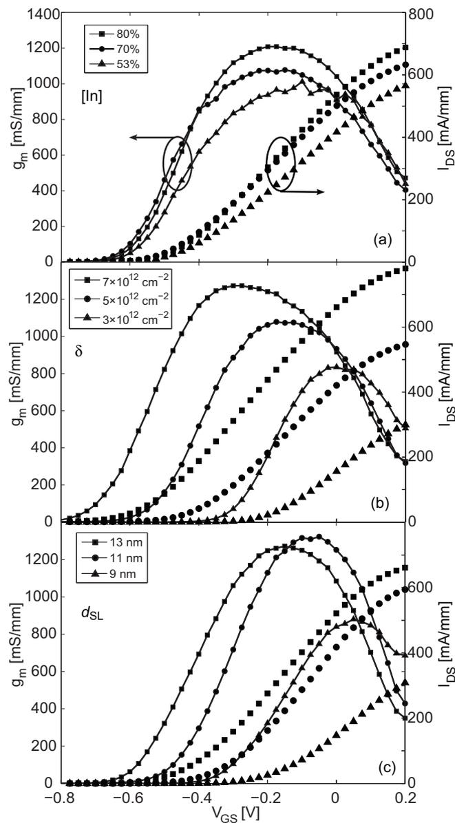
**Figure 6.2** Measured  $g_m(V_{GS})$ ,  $I_{DS}(V_{GS})$  versus (a)  $[In]$ , (b)  $\delta$  and (c)  $d_{SL}$  for 130 nm gate-length InGaAs/InAlAs HEMTs biased at  $V_{DS} = 1.0$  V.
