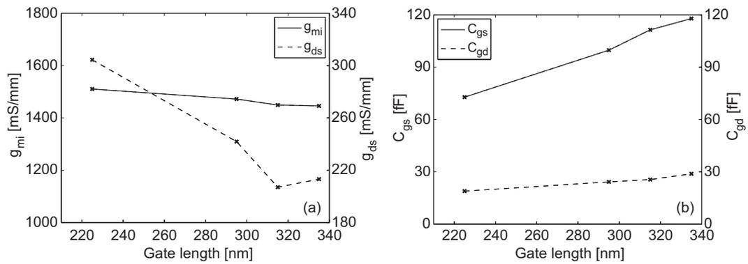
**Figure 5.2** Small-signal parameter (a)  $g_{mi}$  and  $g_{ds}$  (b)  $C_{gs}$  and  $C_{gd}$  dependence on  $L_g$  for a  $2 \times 50 \mu\text{m}$  gate-width InAs/AlSb HEMT biased at  $V_{DS} = 0.6$  V.
