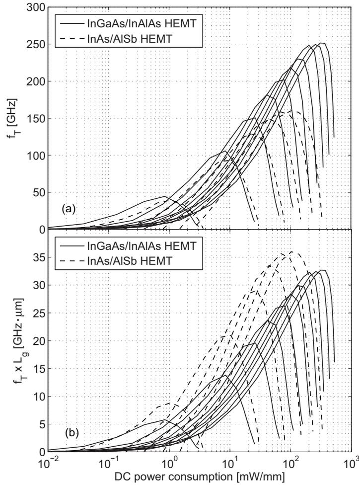
**Figure 3.11** Comparison of the (a) extrinsic  $f_T$  and (b) extrinsic  $f_T \times L_g$  product versus DC power consumption for 130 nm gate-length InGaAs/InAlAs HEMTs and 225 nm gate-length InAs/AlSb HEMTs.
