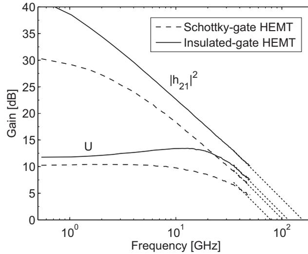
**Figure 7.4** RF performance of Schottky-gate InAs/AlSb HEMT versus insulated-gate InAs/AlSb HEMT.
