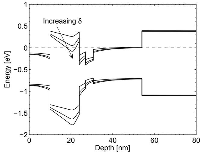
**Figure 6.1** TCAD simulated energy-band diagram with different  $\delta$ -doping concentrations for an InGaAs/InAlAs HEMT at thermal equilibrium (for epitaxial layer details see Figure 3.1(a)).
