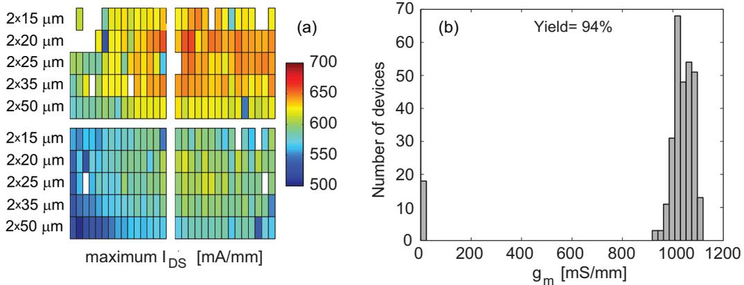
**Figure 3.6** DC wafer mapping of 300 InGaAs/InAlAs HEMTs at  $V_{DS} = 1.0$  V showing (a) the maximum  $I_{DS}$  and (b) a statistical distribution of the corresponding  $g_m$ , revealing a device yield above 90%.
