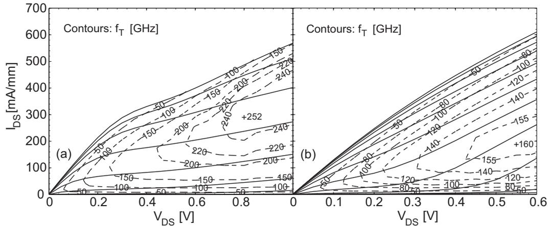
**Figure 3.9**  $I$ - $V$  output characteristics with  $f_T$  contours for (a) 130 nm gate-length InGaAs/InAlAs HEMT with 1.0  $\mu\text{m}$  source-to-drain distance and (b) 225 nm gate-length InAs/AlSb HEMT with 2.3  $\mu\text{m}$  source-to-drain distance.
