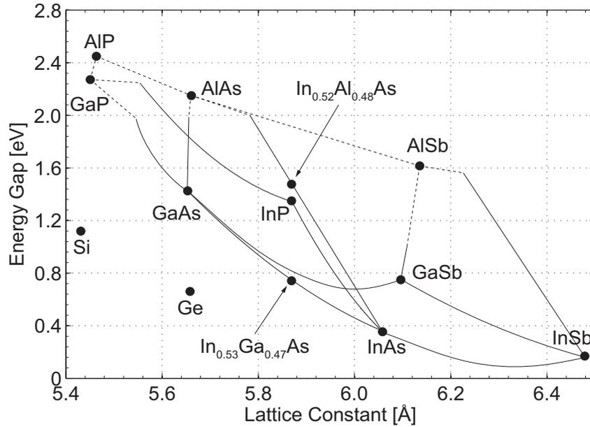
**Figure 2.2** Energy gap versus lattice constant at room temperature for the III-V semiconductors with various alloys (excluding the nitrides) [11, 12, 14, 20]. The dashed lines correspond to an indirect bandgap and the solid lines to a direct bandgap. Si and Ge are included as references.
