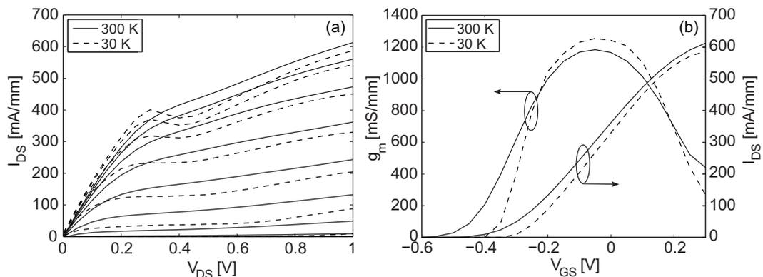
**Figure 3.13** InGaAs/InAlAs HEMT (a)  $I$ - $V$  output characteristic at  $V_{GS}$ : -0.5 V to 0.3 V in steps of 0.1 V and (b)  $g_m(V_{GS})$  and  $I$ - $V$  transfer characteristics at  $V_{DS} = 1.0$  V, at 300 K and 30 K.
