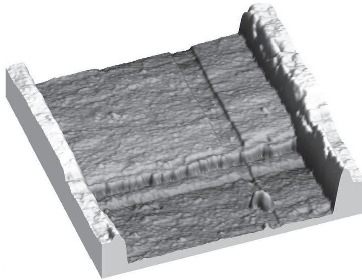
**Figure 7.1** AFM image of an InGaAs/InAlAs HEMT (before gate deposition) with a  $2.3\ \mu\text{m}$  source drain distance, including the mesa edge, the gate recess and part of the ohmic contacts.
