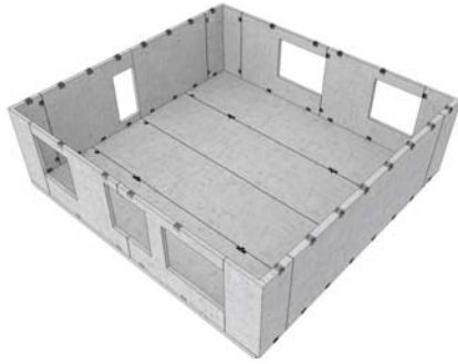
Figure 7.1 Principle sketch of Consolis building system, Consolis (2007).
