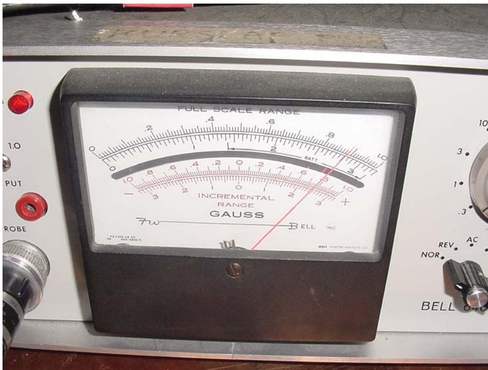
Figure 8 - The display of the Gauss meter which was used during the magnetic field measurements.
