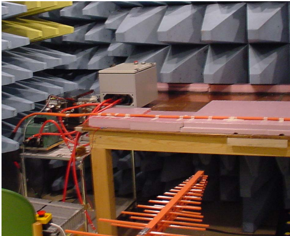
Figure 2 - The antenna, the DC/DC-Converter, the breakers and the test cables in the electric field measurements.
