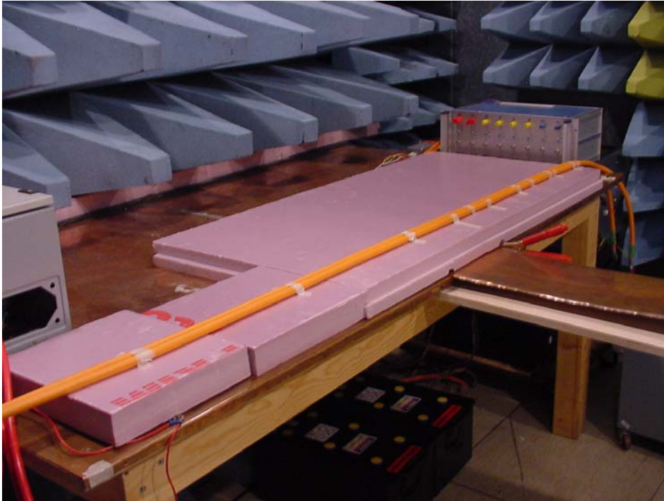
Figure 3 - The shielded cables placed with no distance between them 5 cm from the grounded plane.
