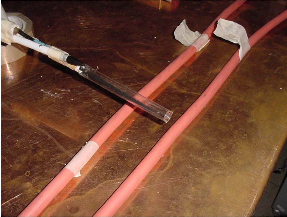
Figure 5 - Measurement of magnetic field with Hall Effect sensor of unshielded cables placed with a distance of 5 cm between them and placed on the grounded plane.
