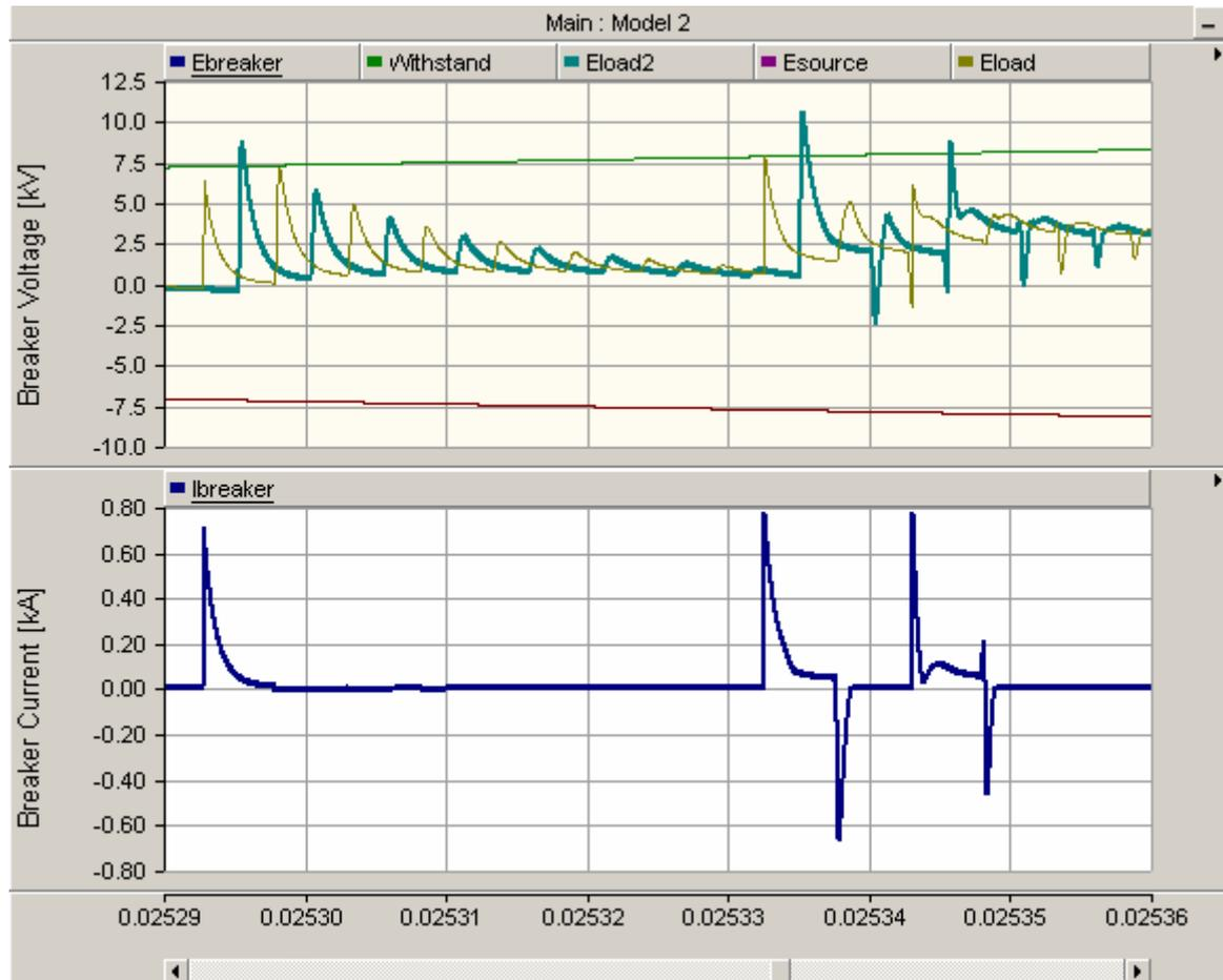
Fig 28: Reflections on the cable
