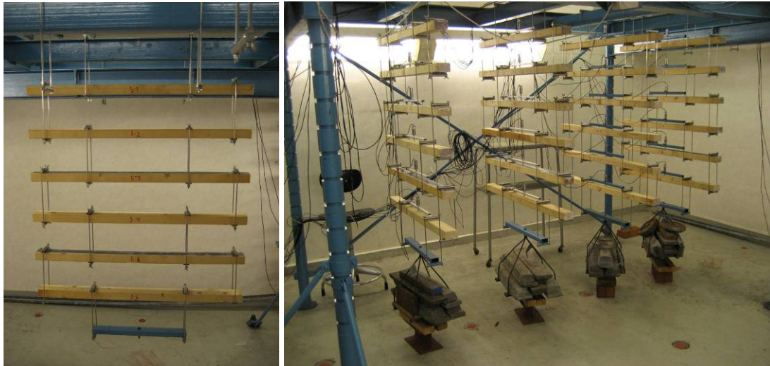
Figure 3.8 Loading arrangement with six specimens in one series (Left). All test specimens loaded (Right).
