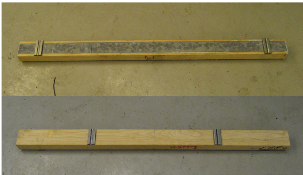
Figure 3.9 Steel plates attached with epoxy on both sides of the beam.
