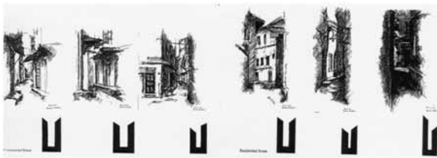
Figure 84 Analysis of the streetscape in Zanzibar showing the narrow and shady streets flanked with three- and four-storey high buildings.
