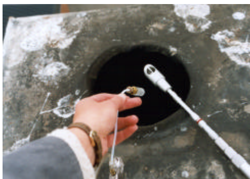
Figure 3.4: Sampling in the chimney pipe
