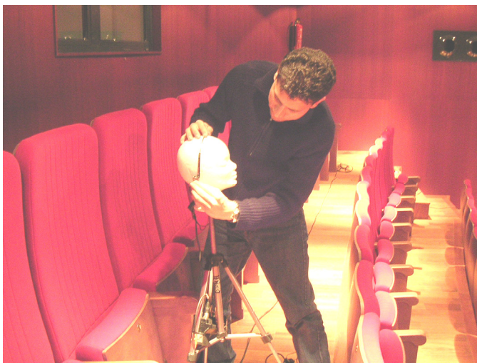
Figure 79: Preparing Setup for IACC measurements
