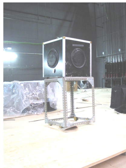
Figure 80: Custom-Made Hexahedron Loudspeaker.
