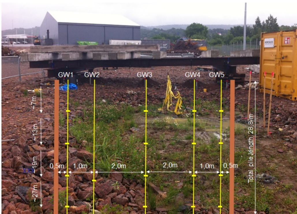
Figure 4.2: Instrumentation for capturing pore pressure and temperature data in the soil profile at different distances from the test piles and at different depth from ground surface. The thermal pile used for heating cycles is the one at the right in the figure. The paired reference pile is to the left.
