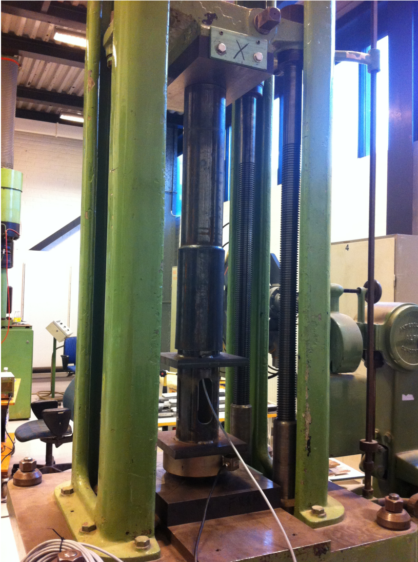
Figure A.8: One of the pile segments under controlled axial compression loading in the laboratory test rig. The pile segment is positioned upside down in the test rig together with the pile hat and load cell, later installed at the pile head in the test field.
