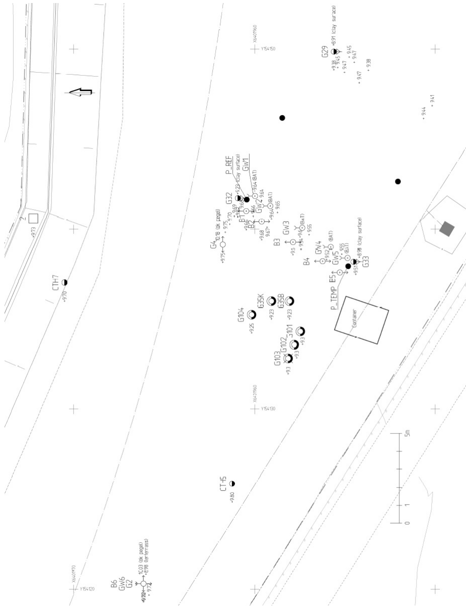
Figure A.2: Plan test field. Geotechnical investigation ID:s. The 4 black circles are steel piles, including the test piles and the supporting piles for the loading rig. Note the external reference point to the west including bellowhose (B6), piezometer pipe (GW6) and levelling plate.
