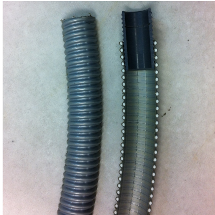
Figure 4.8: Part of a bellowhose used for capturing depth differentiated settlements. The hose in the figure is cut lengthwise to illustrate the position of the ring, in the black socket, responding to the sensor device.
