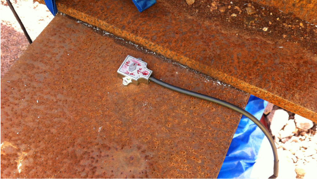
Figure 4.6: Inclinometer sensor fixed at the main beam of the loading rig. The sensor was later covered with an adhesive climate protection mat.
