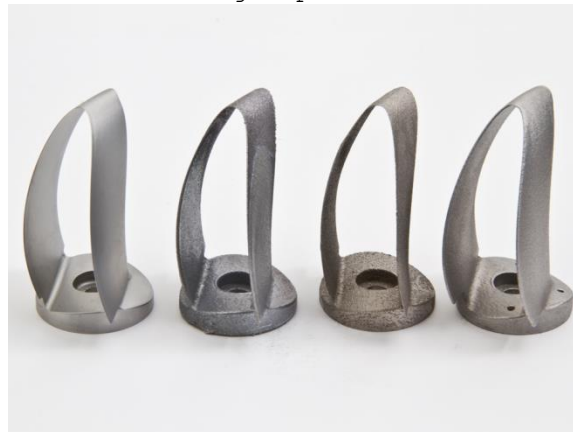
Figure 4 - 50 mm prototype blades manufactured from 1): multi-axis milling/Aluminum/thin profile, 2): SLM/Aluminum/thin profile, 3): SLM/Titanium 4: SLM/Aluminum.
