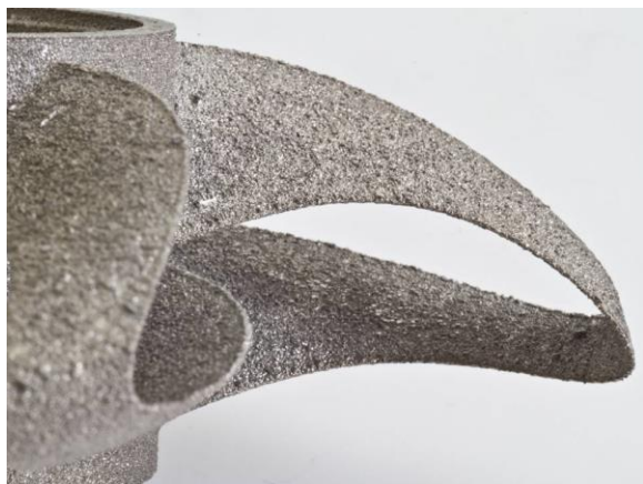
Figure 5 - Close-up of propeller manufactured from EBM/Titanium. 120 mm diameter.
