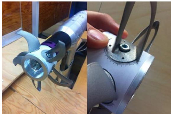
Figure 7 - Final propeller concept with adjustable pitch angles. SLM manufactured aluminum blades with a machined aluminum hub.
