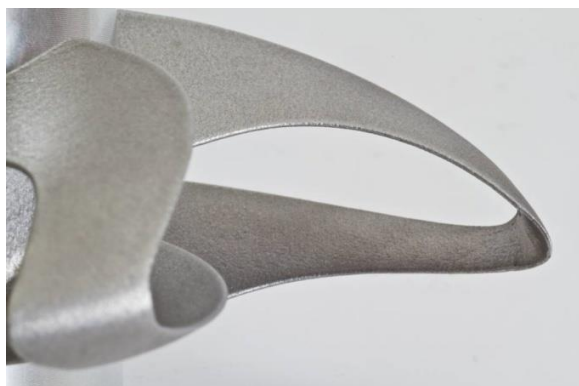
Figure 6 - Close-up of the propeller blade manufactured from SLM/Aluminum.
