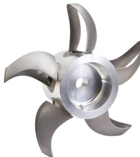
Figure 1 - Prototype of wind tunnel test Boxprop with adjustable pitch blades made by Selective Laser Melting, AlSi10Mg. 150 mm diameter.
