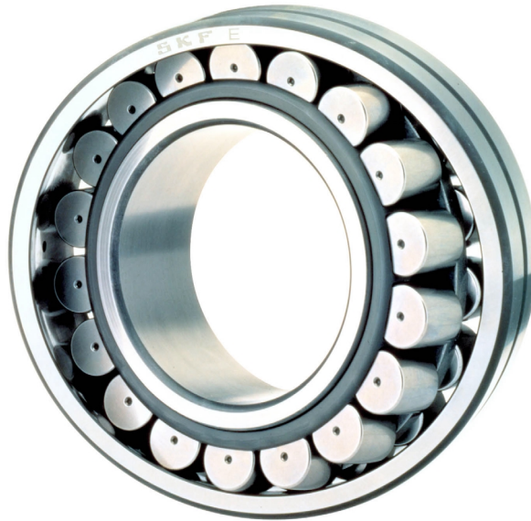
Figure 1: The Spherical Roller Bearing (SRB) is a heavy-duty bearing with very high load carrying capacity due to the two rows of rollers. The bearing is self-aligning and therefore insensitive to errors of alignment. The bearing in the figure is not a SRB 24024 but a spherical roller bearing with fewer rollers. The appearance is however very similar. [SKF Sverige AB]
