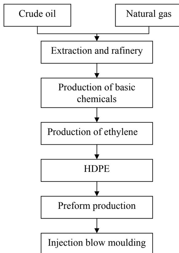
**Figure 6 Simple flow chart of the plastic bottle production**
