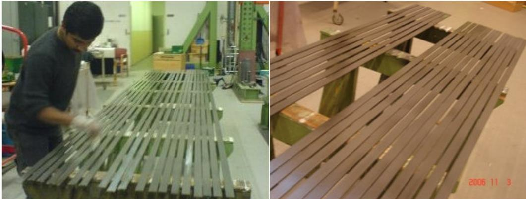
*Figure 5.3 Surface preparation- Primer application for steel reinforcements*
