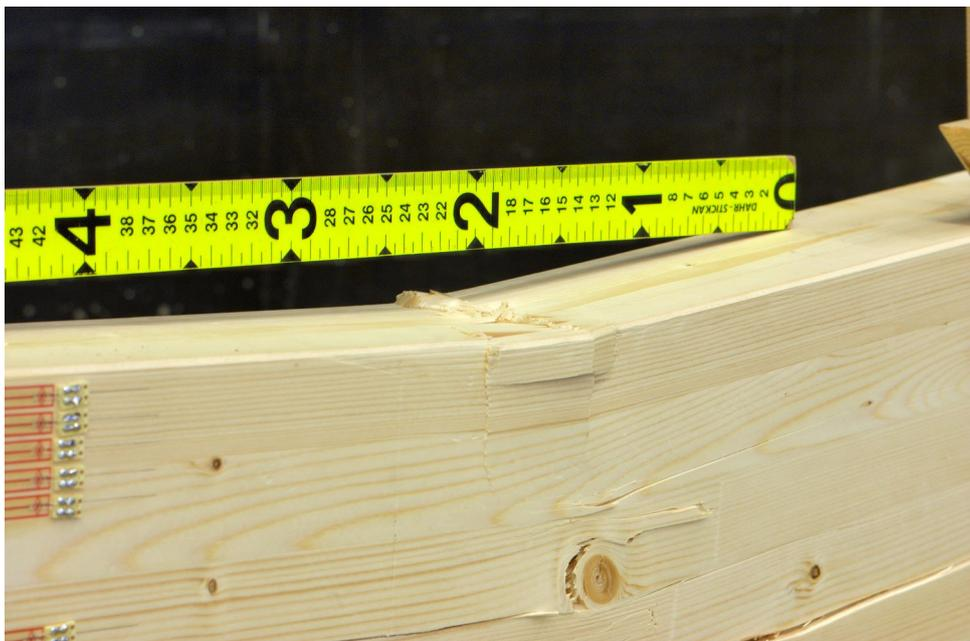
*Figure 5.37 Compressive plastification (crushing of timber)*
