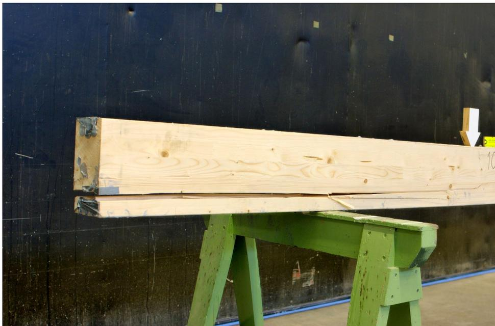
*Figure 5.57 Failure(Beam 10) Shear Failure near to support*
