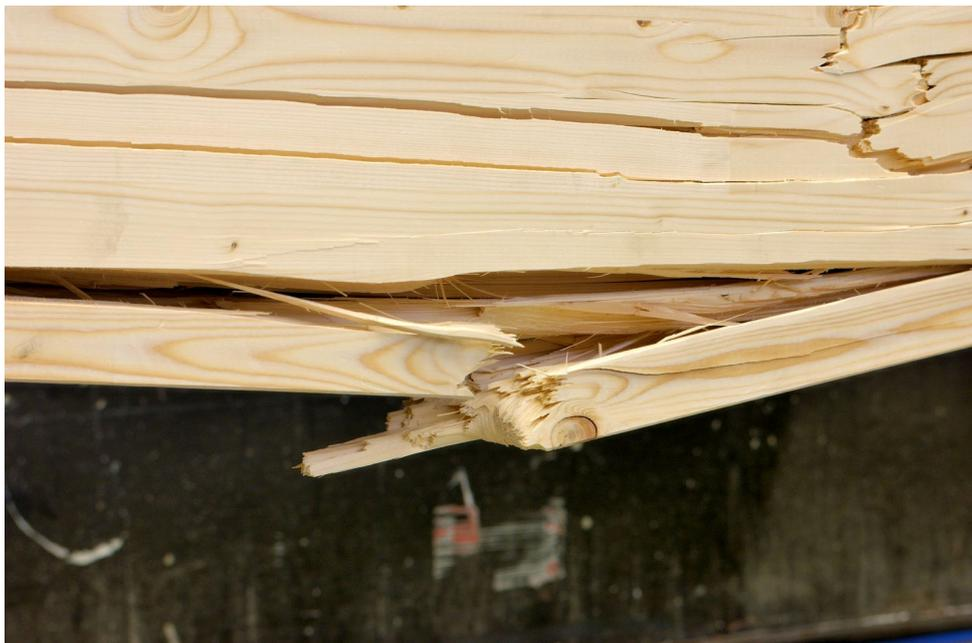
*Figure 5.20 Knot on tension side which initiated tension failure (Beam 2)*
