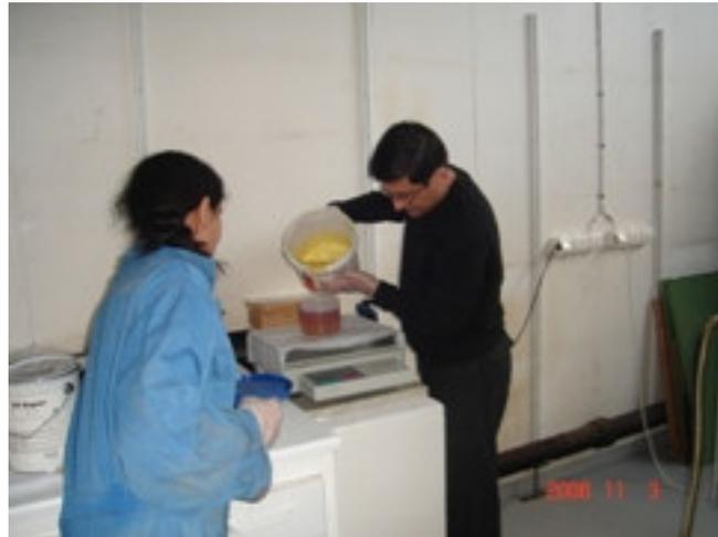
*Figure 5.5 Preparation of Adhesives- Weigh batching of components*
