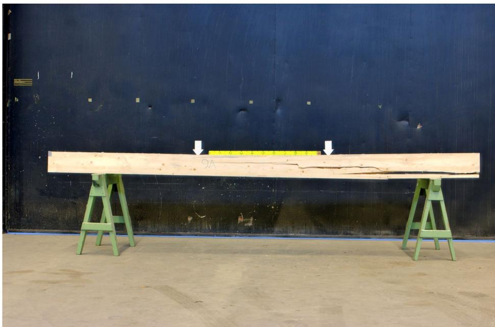
Figure 5.52 Failure (Beam 9)
