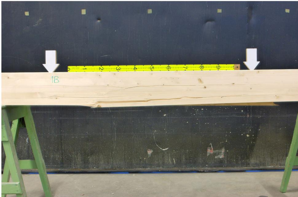
*Figure 5.15 Beam 1 – Tensile failure*
