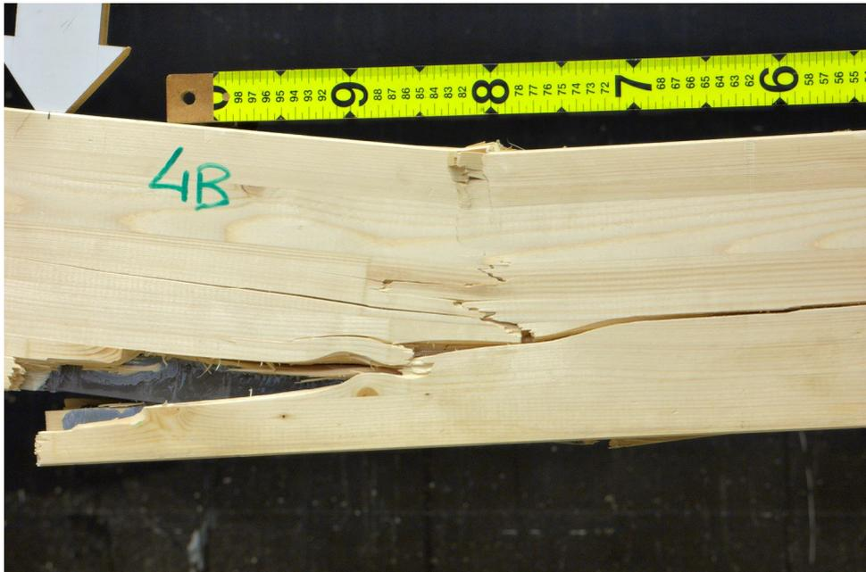
*Figure 5.34 Failure(Beam 4)*
