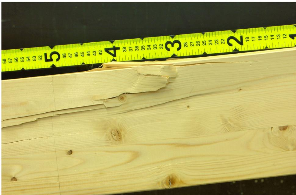
*Figure 5.42 Plastification in the compressive zone*
