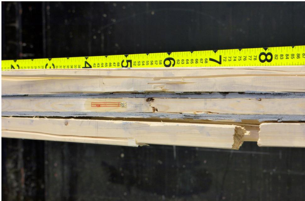
*Figure 5.26 Cause for Failure, knot at the bottom*
