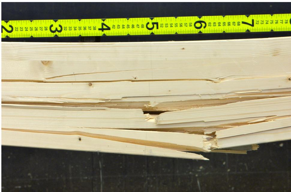
*Figure 5.30 Failure(Beam 5)*
