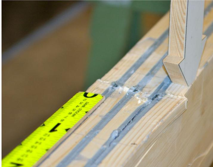
Figure 5.48 Compression failure, crushing of Timber fibers as well as CFRP
