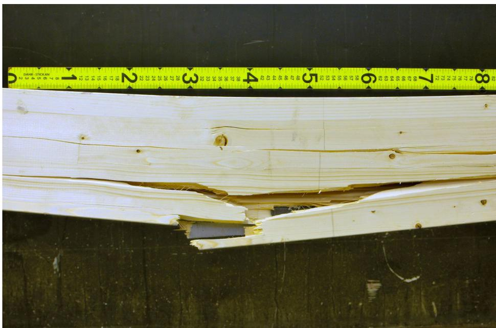
Figure 5.40 Failure (Beam 6)
