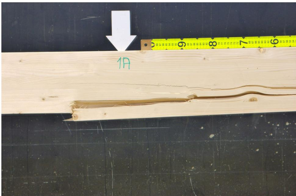
*Figure 5.16 Beam 1 Knot on tension side which initiated tension failure*
