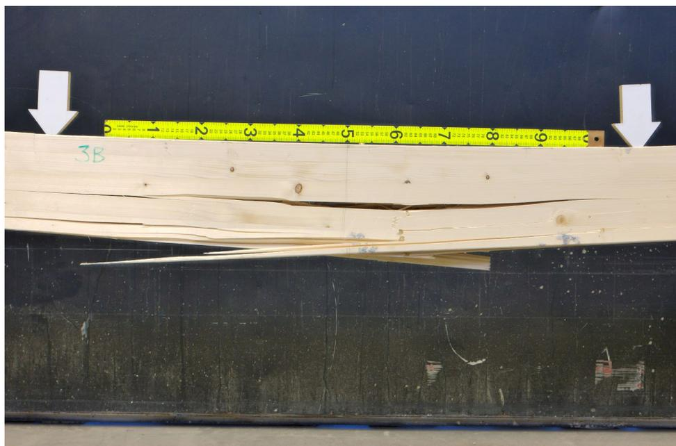
Figure 5.24 Failure (Beam 3)
