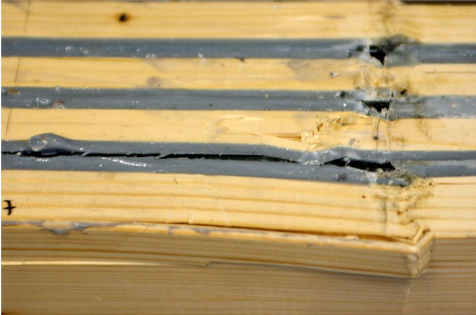
*Figure 5.58 Compressive crushing in timber as well as laminate*
