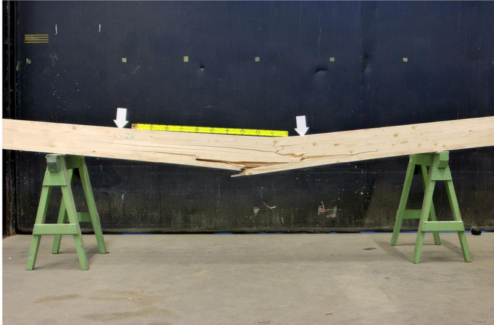
*Figure 5.19 Beam 2 – Tensile failure*
