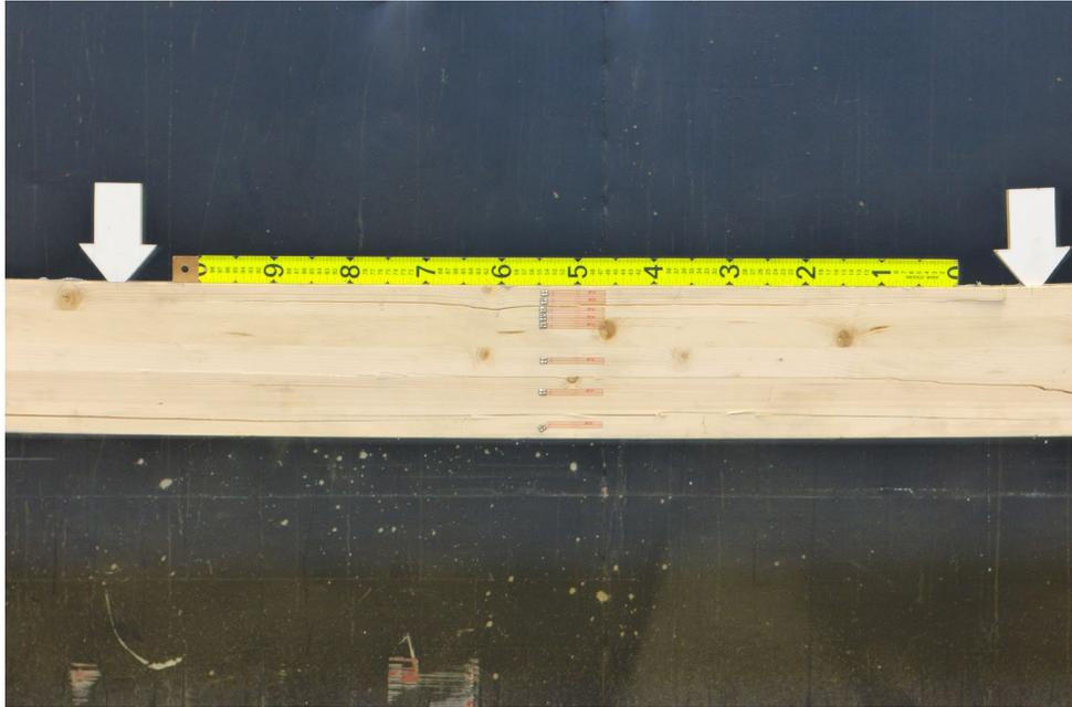
*Figure 5.56 Failure (Beam 10) Split Crack in the compressive zone*
