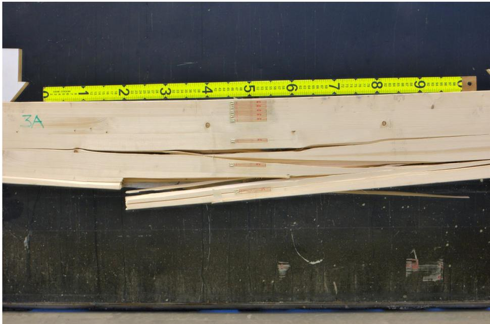
*Figure 5.25 Failure (Beam 3)*
