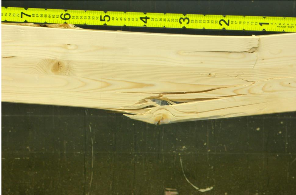
*Figure 5.41 Crack initiation at knot*
