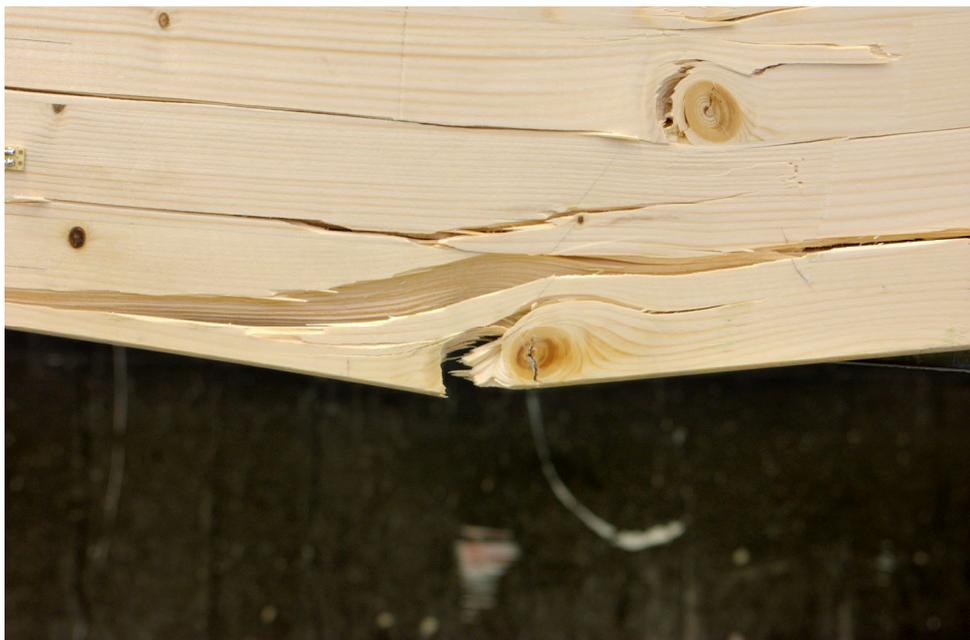
*Figure 5.35 Crack initiation at knot*
