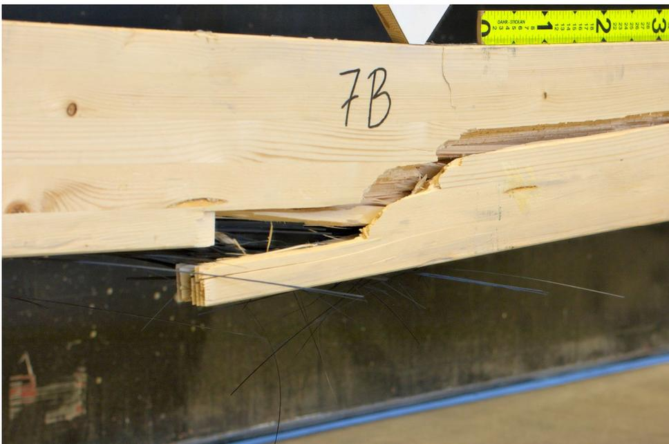
*Figure 5.47 Rupture of the laminate at the finger-joint location*
