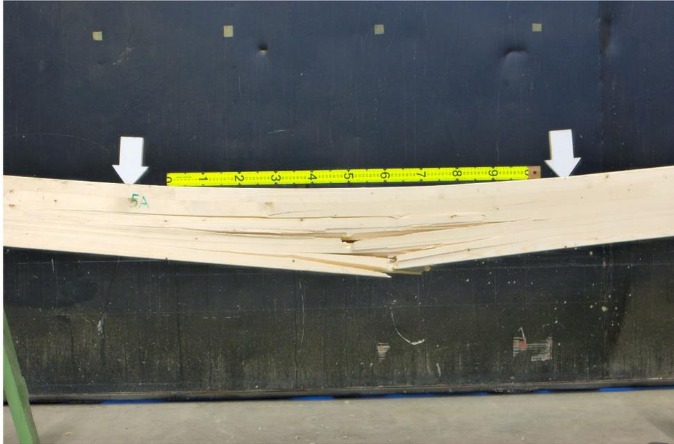
*Figure 5.29 Failure (Beam 5)*
