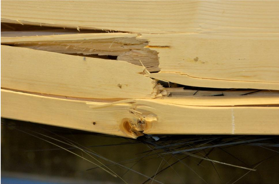
*Figure 5.46 Crack initiation at knot*
