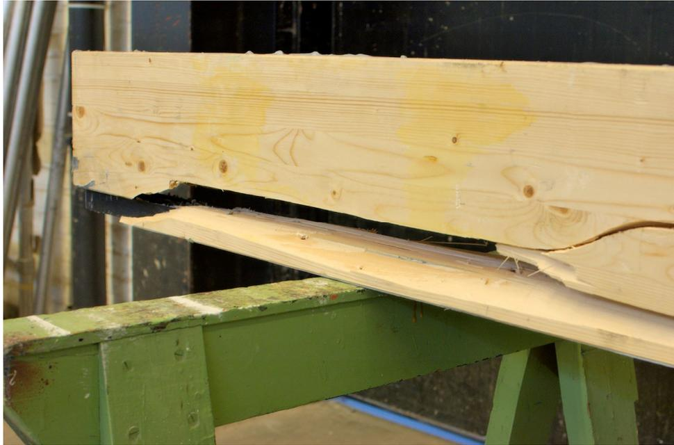
*Figure 5.53 Shear failure near supports (Beam 9)*
