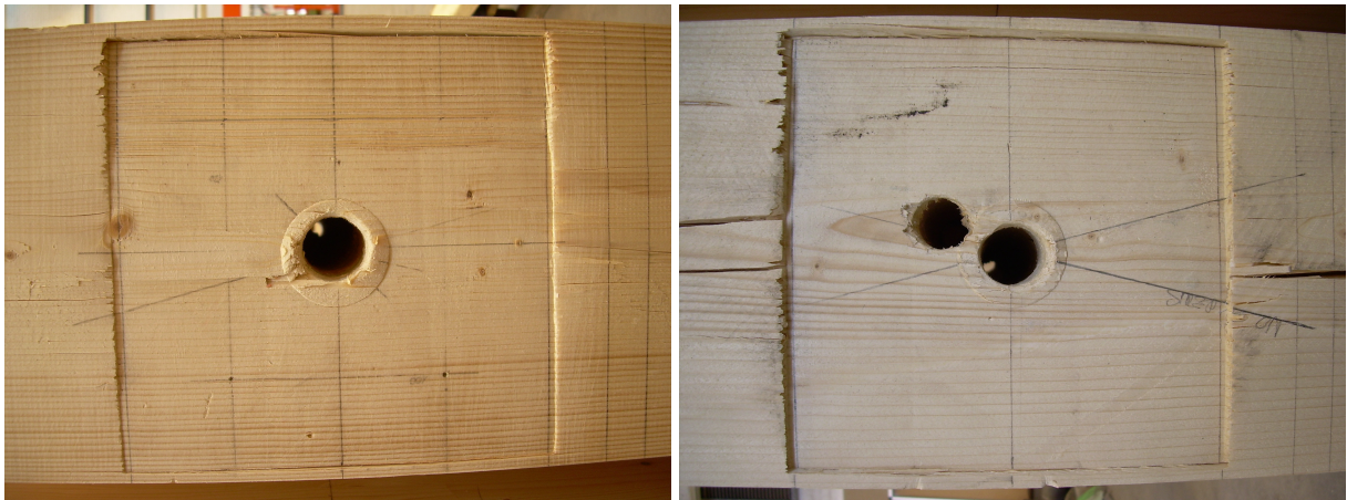
Figure 5.19 Remaining plastic deformations and the imperfection due to mal-production, pLHW
