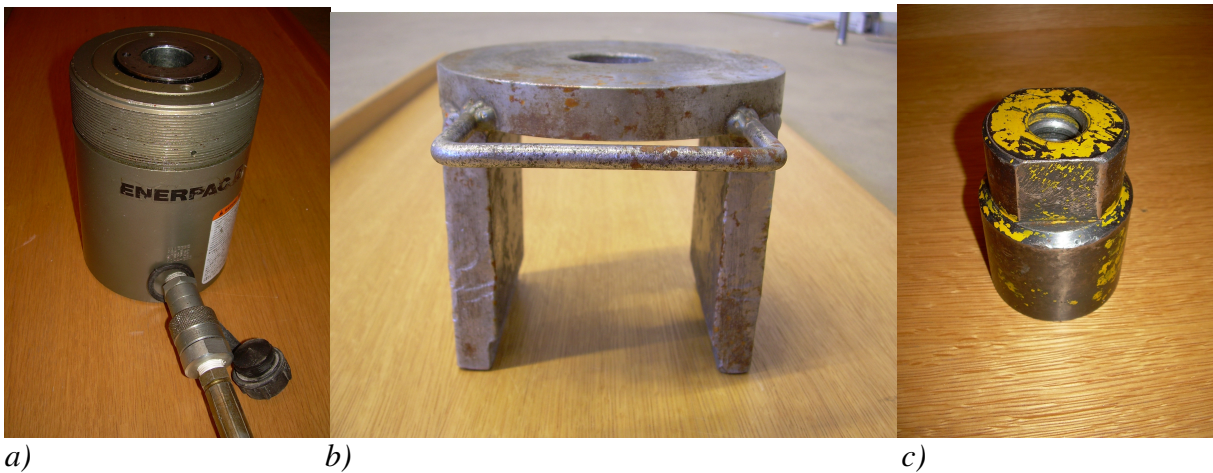
Figure 2.13 Tension equipment: a) hydraulic hollow-core jack, b) tensioning chair and c) backnut
