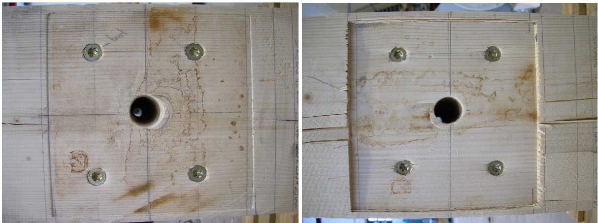
Figure 5.27 Remaining plastic deformations of the reinforced specimen, S12pl20
