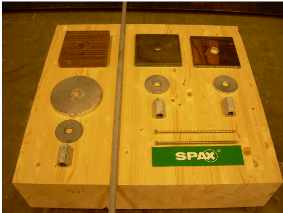
Figure 5.2 Components included in the different anchorage configurations
