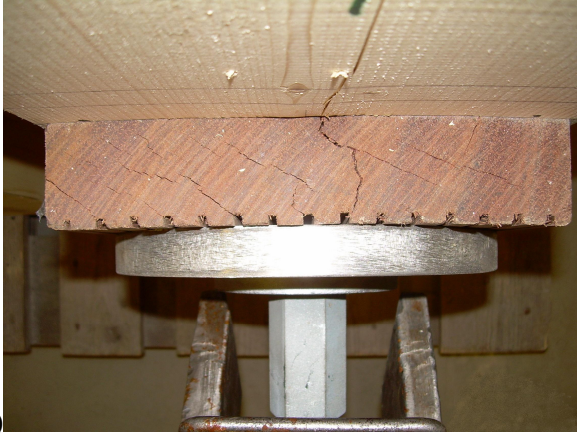
Figure 5.13 a) Hardwood crack due to pre-stressing force ( p_{lHW} ); b) Bending of the 15 mm plate due to pre-stressing force ( p_{l15} )
