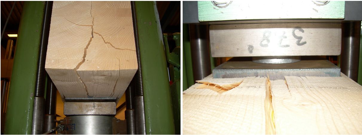
Figure 5.28 Surface crack propagated down the short edge of a test specimen
