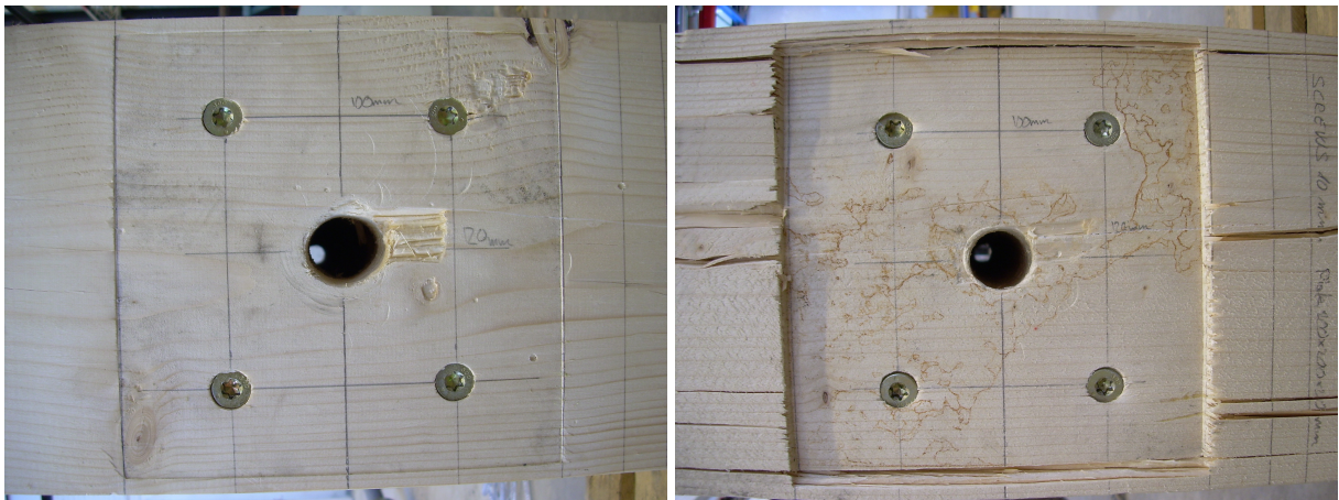
Figure 5.23 Imprint of the plate and the vertical displacement of the screws, S10pl20
