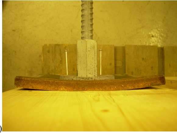
Figure 5.13 a) Hardwood crack due to pre-stressing force ( p_{lHW} ); b) Bending of the 15 mm plate due to pre-stressing force ( p_{l15} )
