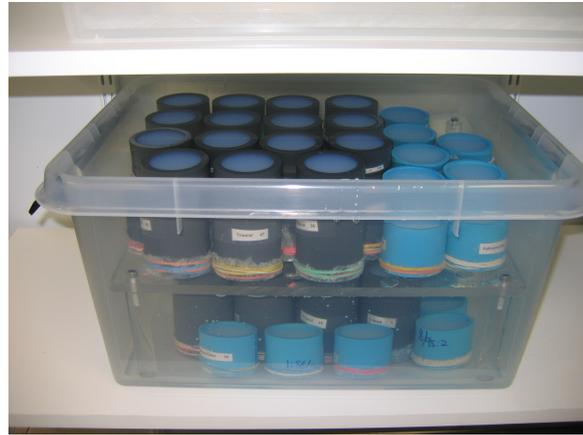
*Figure 3. Climate box with silica sol specimens inside their moulds fully immersed in a solution with pH 11.*
