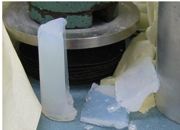
*Figure 15. Vertical failure plane in a silica sol specimen tested 6 days after mixing.*
