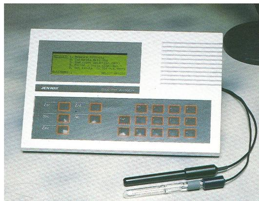
**Figure 13.** The ion selective apparatus used for the diffusion of chlorides from silica sol tests.
