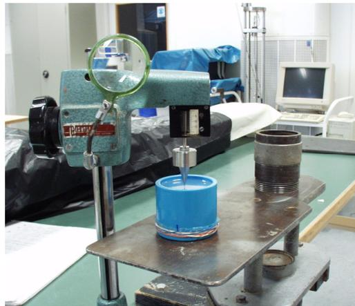
*Figure 5. Silica sol specimen ready to be tested with a fall-cone apparatus.*
