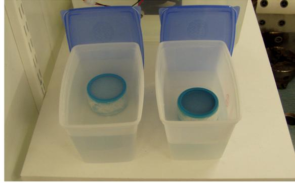
**Figure 12.** Climate boxes used for the diffusion of chlorides from silica gel test. Silica sol specimens inside their boxes in a room with 8°C.
