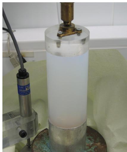
*Figure 4. Silica sol specimen ready to be tested in an unconfined compression test apparatus.*
