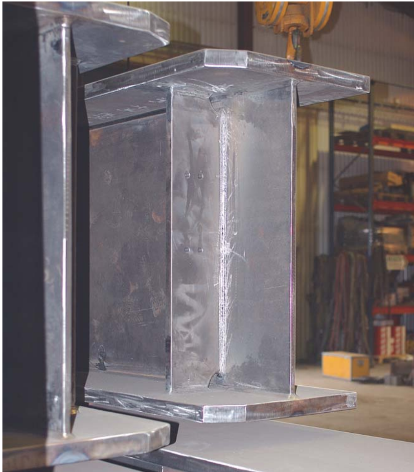
Figure 1.1 Photo of a steel beam with vertical stiffeners, ready to be delivered.
