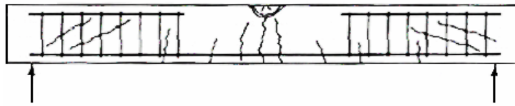
Figure 2.8 Shape of the beam 2 at bending moment failure, from Nadim Hassoun (2002).
