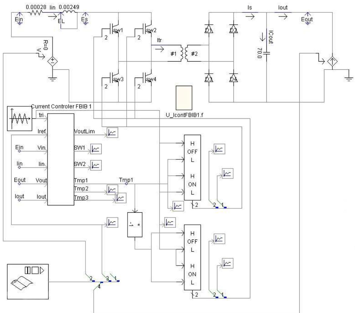
Figure B.1: Printout over the full bridge isolated boost converter implemented in EMTDC<sup>©</sup>
