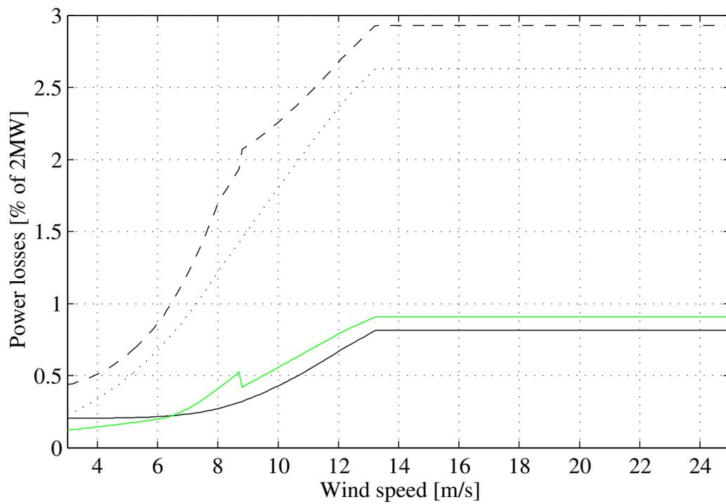
Figure 4.5: The losses of the 2MW semi variable speed wind turbine. Solid transformer losses, dashed generator losses, dotted gearbox losses and grey converter losses.
