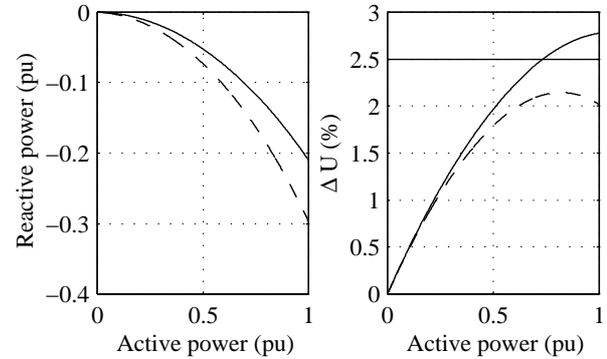
Figure 5. Reactive power consumption for two different induction generators, X/R=1.7.
