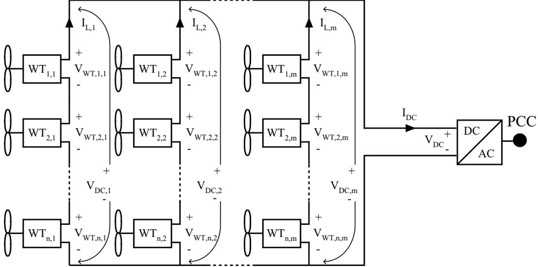
Figure 6.1: The layout of the series connected wind park.
