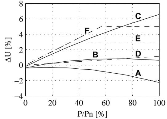
Fig. 8. Voltage level influence by different WECS. A-C Fixed-speed system, D-F variable-speed system. A & D: X/R=5, B: X/R=2, C: X/R=1.1, E: X/R=1.1 over voltage limit 3% and, F: X/R=1.1 over voltage limit 5%.
