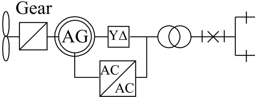
Figure 4.4: Principal scheme of the 2MW semi variable speed wind turbine.
