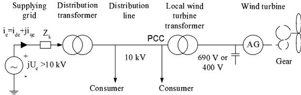
Figure 1. Model of the wind turbine and electrical grid.
