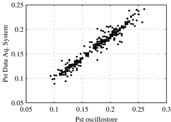
Fig. 3.  $P_{st}$  level on the local 400 V grid determined using Oscillostore and from data acquisition system, during three hours of operation with low flicker levels. One minute  $P_{st}$  values.
