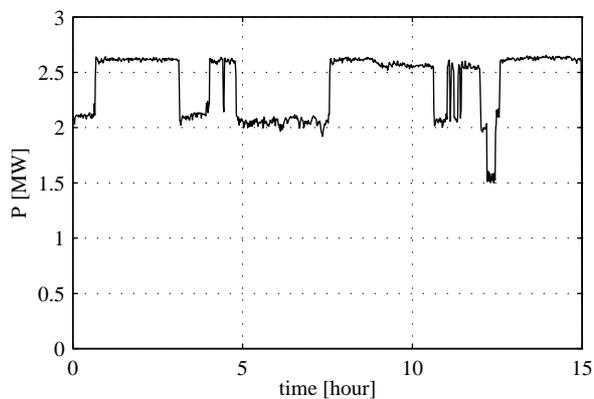
Fig. 11. Active power from Bockstigen during a high wind speed and high load condition.
