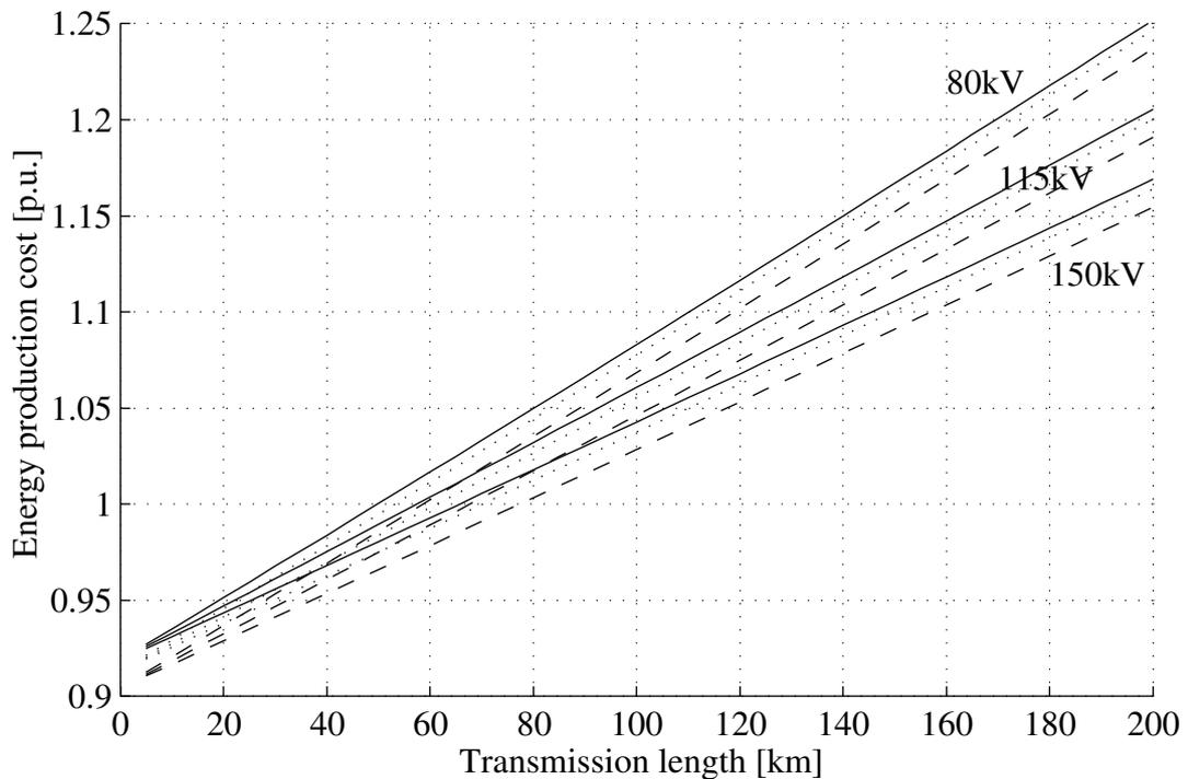
Figure 5.12: The normalized energy production cost for the different configurations of the AC/DC system. For a 300MW wind park, an average wind speed of 10m/s and for different transmission lengths. Solid fix speed wind turbines, dashed wind turbines with the DFIG system and dotted fix speed wind turbines speed controlled with the offshore converter station.
