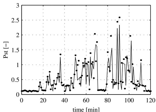
Fig. 4.  $P_{st}$  level on the local 400 V grid determined using Siemens Oscillostore P513 (dots) and from data acquisition system (solid line), operation at high flicker levels.
