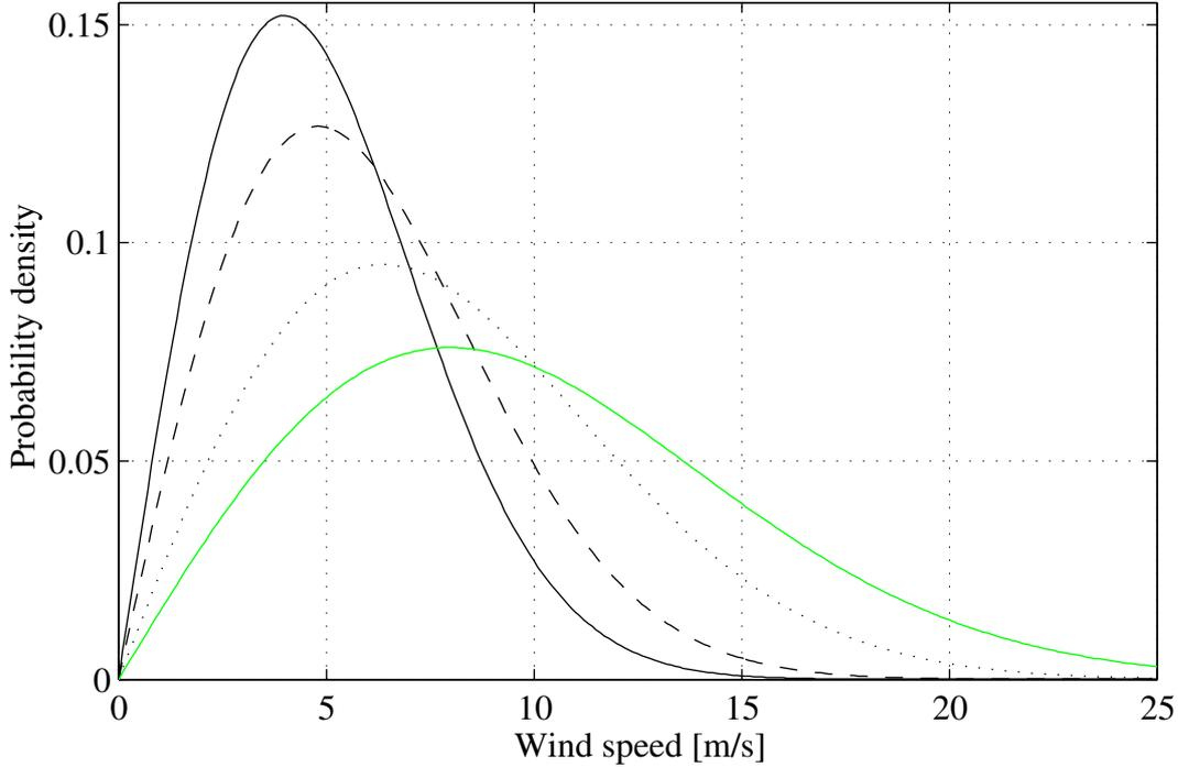
Figure 3.1: Rayleigh distribution function for different mean wind speeds, solid 5m/s, dashed 6m/s, dotted 8m/s and grey 10m/s.
