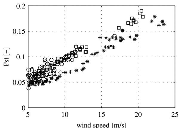
Fig. 6.  $P_{st}$  contribution as function of wind speed, X/R=0.5. \* sea wind, circles forest wind and squares wake operation (255 degrees). Ten minute  $P_{st}$  values.
