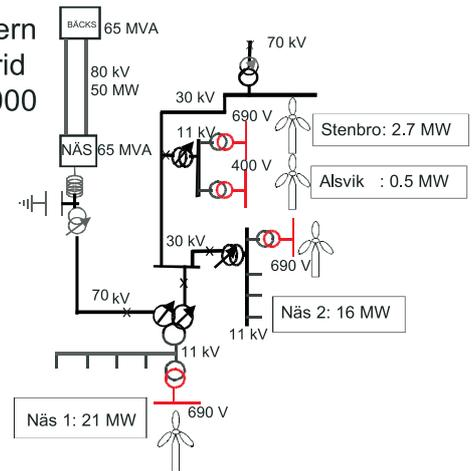
Fig. 2. Schematic sketch of the Näsudden grid.
