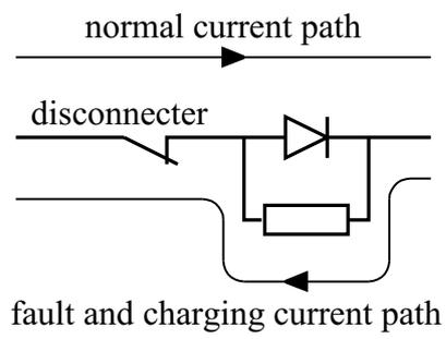
Figure 6.14: Scheme of the DC-breaker.
