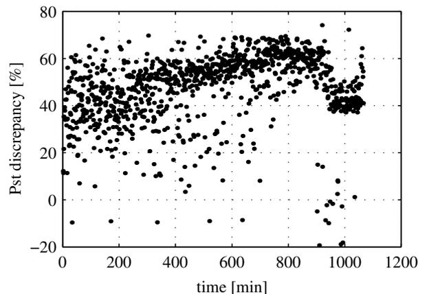
Fig. 13. Discrepancy between the actual flicker emission and the formula from IEC-61400-21, 70 degrees grid impedance angle.
