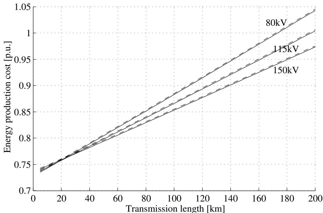
Figure 5.20: The normalized energy production cost for the different configurations of the series DC system. For a  $300\text{MW}$  wind park, an average wind speed of  $10\text{m/s}$  and for different transmissions lengths. Solid maximum 4 failed wind turbines per leg, dashed maximum 8 failed wind turbines per leg.
