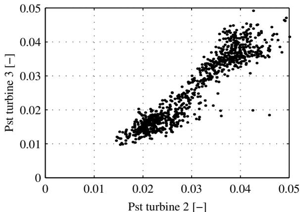
Fig. 11. Flicker emission from the no-loaded generator compared to flicker emission from turbine 3, 70 degrees grid angle. One minute  $P_{st}$  values.
