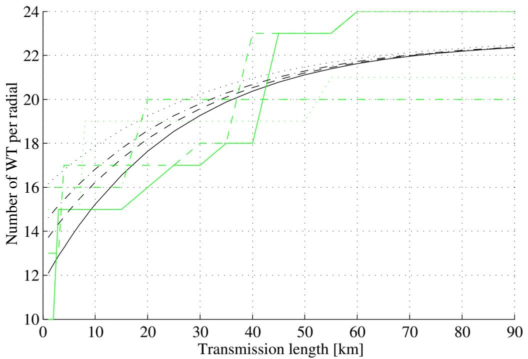
Figure 5.6: Number of wind turbines per radial for 45kV transmission voltage. Black theoretical curves and grey actual curves. Solid 60MW park, dashed 100MW, dash-dotted 160MW and dotted 300MW wind park.
