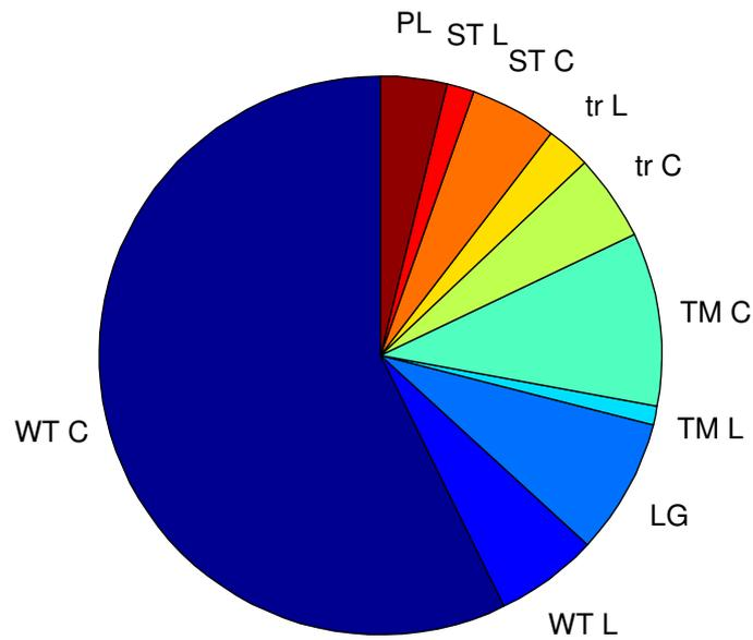
Figure 5.18: The energy production cost divided into components for the large DC wind farm for the reference case.
