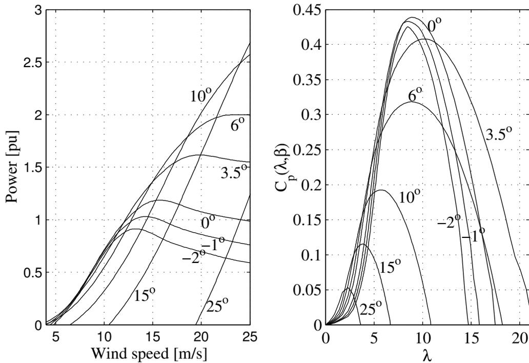
Figure 3.2: The mechanical power as function of wind speed and pitch angle for a fixed rotor speed, left plot, and the aerodynamic efficiency as function of  $\lambda$  and pitch angle, right plot.
