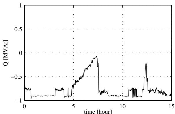
Fig. 13. Reactive power from Bockstigen during a high wind speed and high load condition.
