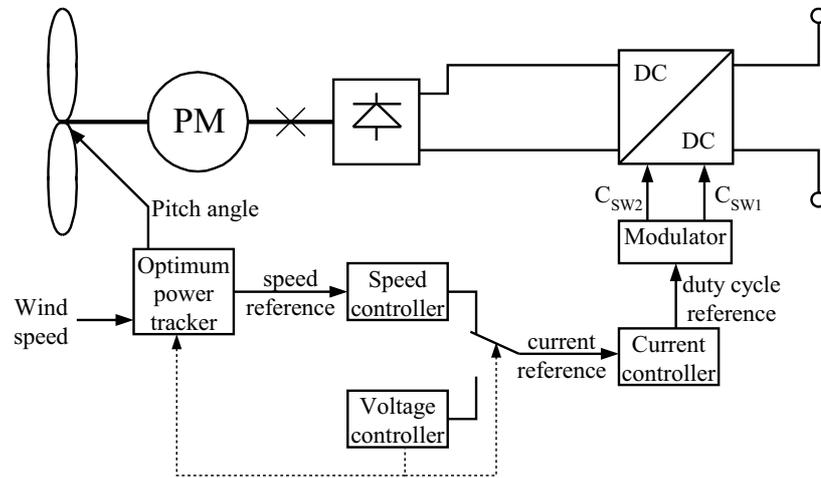
Figure 6.2: The layout of the control system for the series connected wind turbine.
