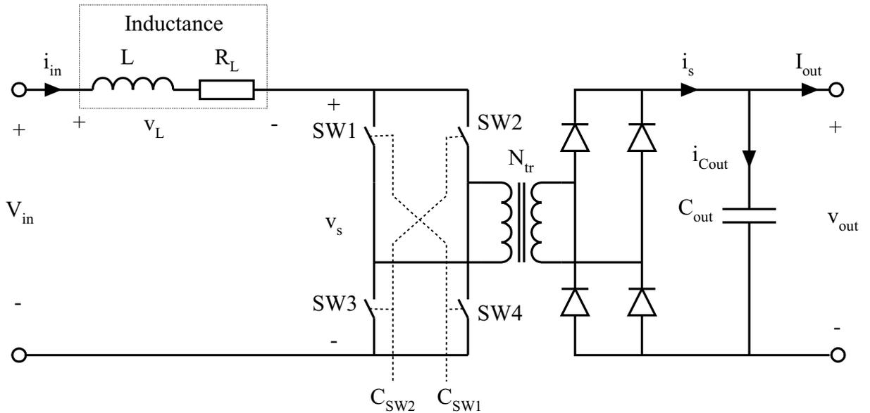
Figure 6.3: The scheme of the full bridge isolated boost converter that is used for derivation of the current controller.
