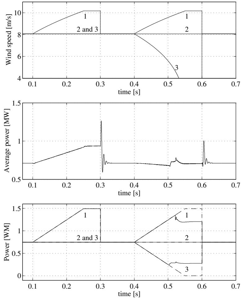
Figure 6.10: The input to the simulations of the three series connected converters, the different inputs to the three wind turbines are numerated 1 to 3. In the top plot the wind speeds for the wind turbines are shown. In the middle plot the average output power and in the bottom plot the optimal turbine power (black dashed lines), actual turbine power (solid black line) are shown.
