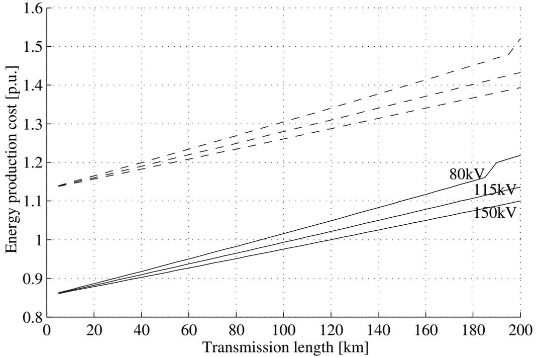
Figure 5.17: The normalized energy production cost for the different configurations of the large DC system. For a 300MW wind park, an average wind speed of 10m/s and for different transmissions lengths.
