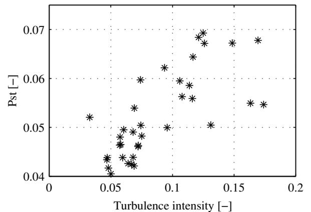
Fig. 10.  $P_{st}$  contribution as function of turbulence intensity, for wind speeds between 12 and 13 m/s.  $X/R=1$ , one minute  $P_{st}$  values.
