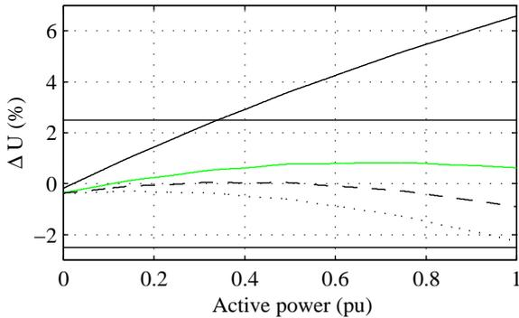
Figure 3. Voltage change as a function of produced power for various X/R-ratios. The grid strength is 10 times the rating of the turbine. Solid XR=0.5, Grey XR=2, Dashed XR=3, Dotted XR=5. The 2.5 % limits are marked with solid lines.
