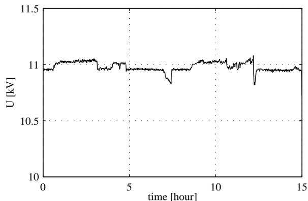
Fig. 12. Voltage level at Bockstigen during a high wind speed and high load condition.
