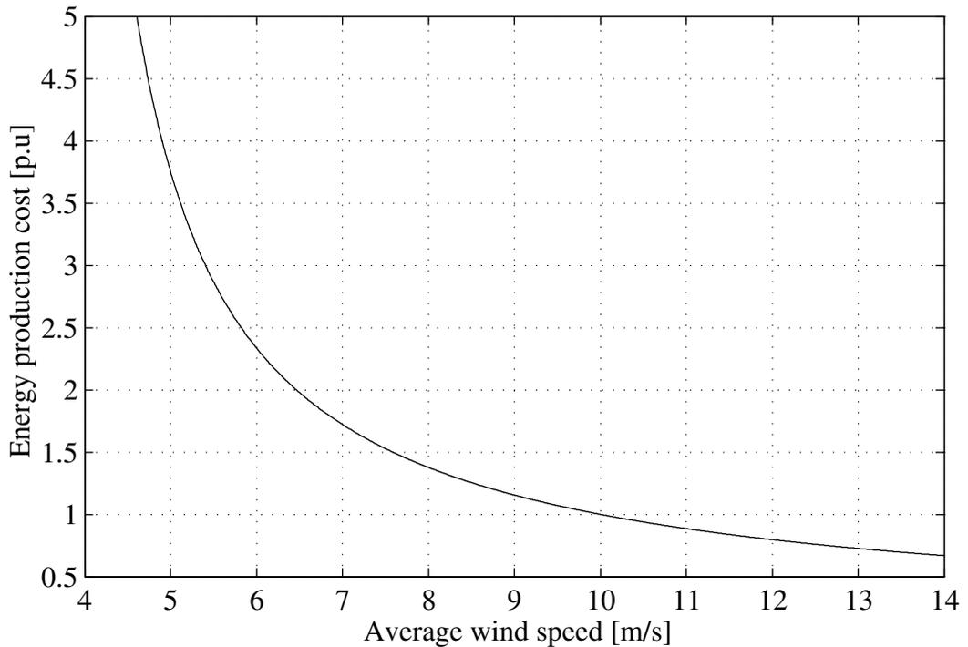
Figure 5.3: Energy production cost as function of the average wind speed, normalized with the prize at a average wind speed of 10m/s.
