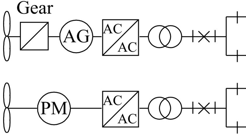
Figure 4.6: Principal schemes of the 2MW full variable speed turbine, top with asynchronous generator and bottom with permanently magnetized generator.
