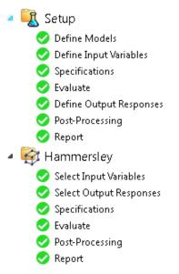
Figure 3.2: The different steps of a setup and a Hammersley DOE in HyperStudy
