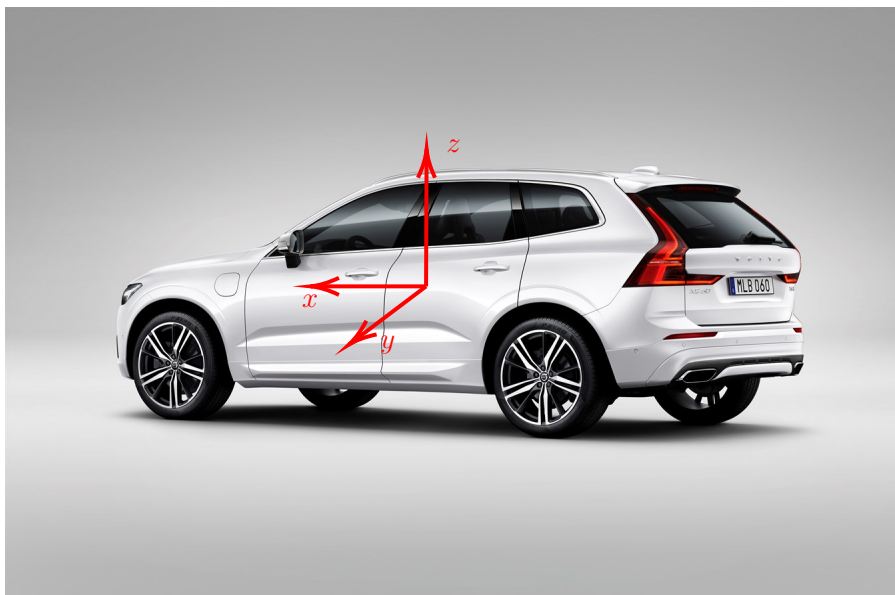
Figure 3.2: The GNSS/INS's approximate location together with its coordinate system. The GNSS/INS is placed as close to the centre of the car body as possible, just above the mid console and between front and back seats.
