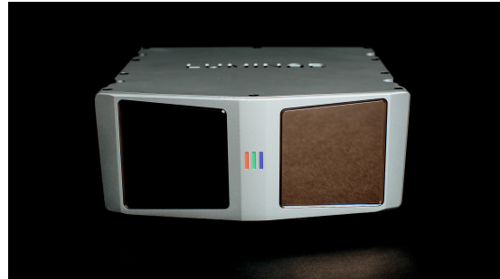
(b) Appearance of the Luminar LiDAR with two optical transmitters
