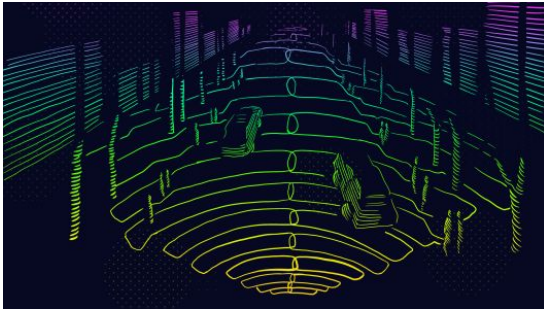
(a) Approximate scanning pattern for the used LiDAR sensor
