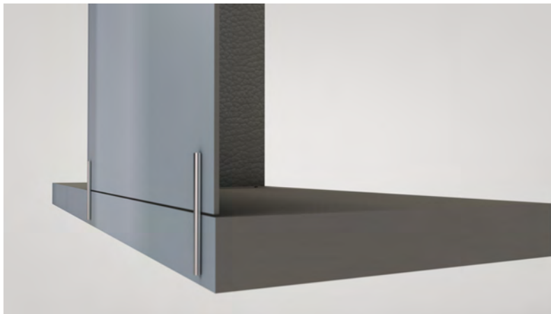
Figure 6.14: Section view of a wall, illustrating the pegs in a locked position.
