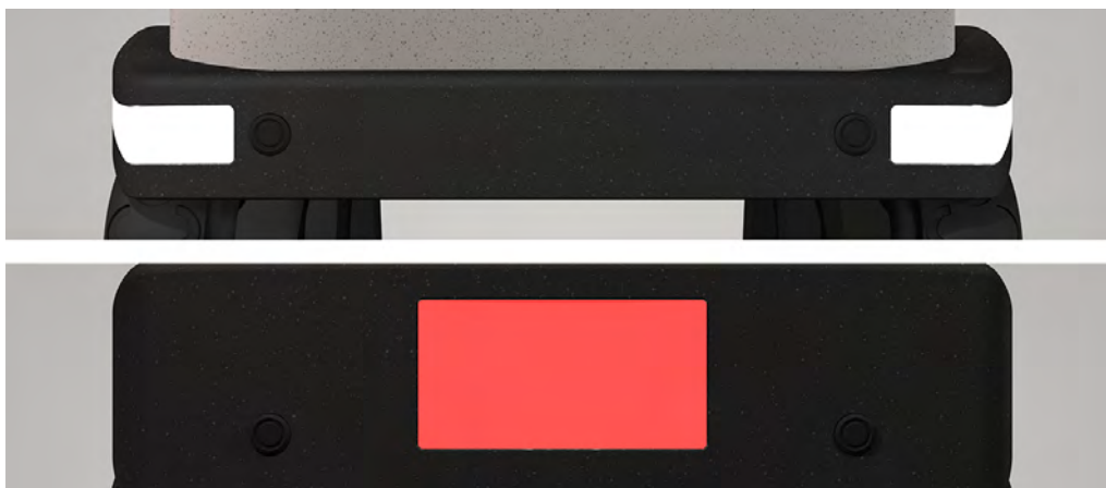
Figure 6.19: At the top: Two front sensors and two head lights. At the bottom: Two back sensors and the rear light.
