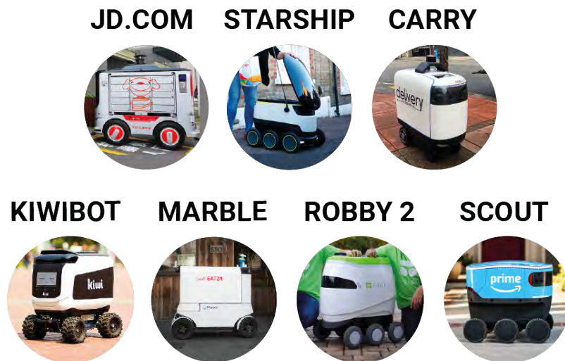
Figure 2.1: Images of delivery robots currently operating or being tested in public areas; 1. JD robot, 2. Starship, 3. Dispatch Carry, 4. Kiiwibot, 5. Marble, 6. Robby 2, 7. Scout.
