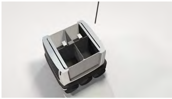
(a) Section view and compartment orientation.
