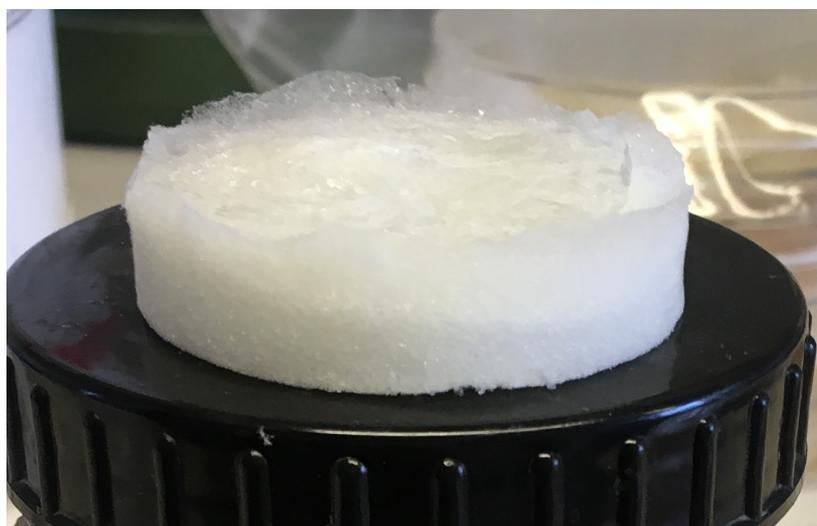
*Figure 12. Oxidized CNC resulted in a foam like material.*
