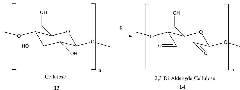
*Scheme 5. Oxidation of both micro- and nano- crystalline cellulose under conditions g: H<sub>2</sub>O, NaIO<sub>4</sub>, acetic acid at 45°C for 4 hours.*
