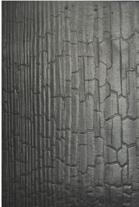
Figure 56. | Photo of chosen cladding material. Shou sugi ban named "Kärnfuru, Kraftigt bränd. Linoljad" from the Swedish company Tree .
