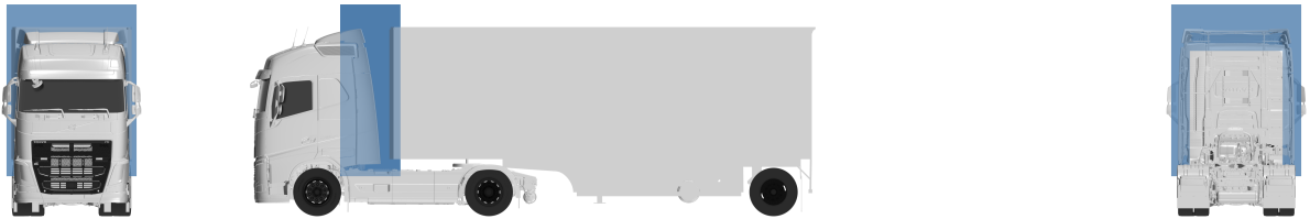
(c) Tractor-trailer gap ring, note that the trailer is hidden in the rear view
