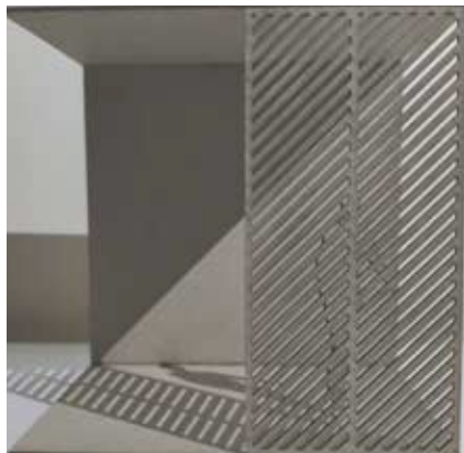
Diagonal pattern only lets light through from one direction.
