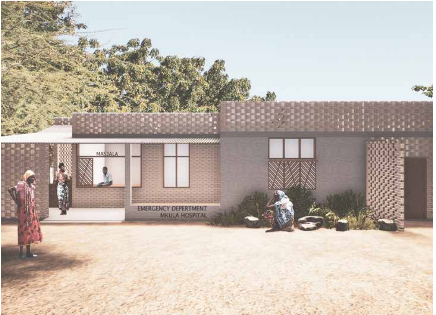
Exterior perspective of casualty, the entrance is marked by a porch structure that highlights the entrance and provides shelter from the sun.
