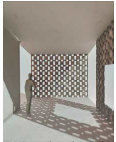
Brick pattern loosened for more light and a window for more openness.
