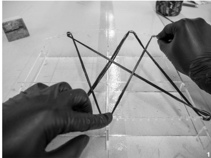
Figure 20. Carbon fiber weaving, Stop Motion Photo 1. Author's own copyright.
