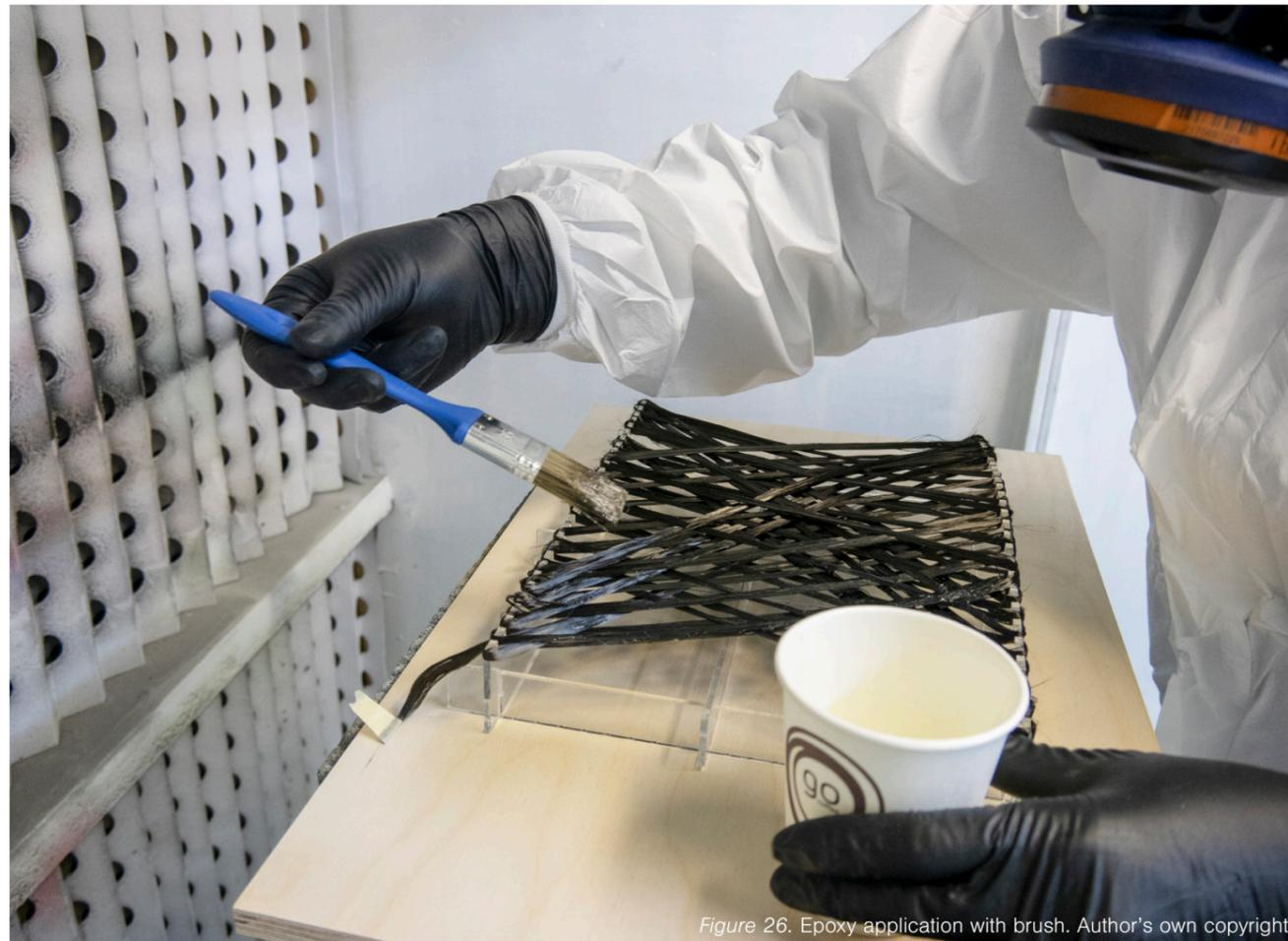
Figure 26. Epoxy application with brush. Author's own copyright.
