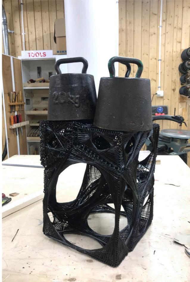
Figure 99. Final model, 60kg test load. Author's own copyright.
