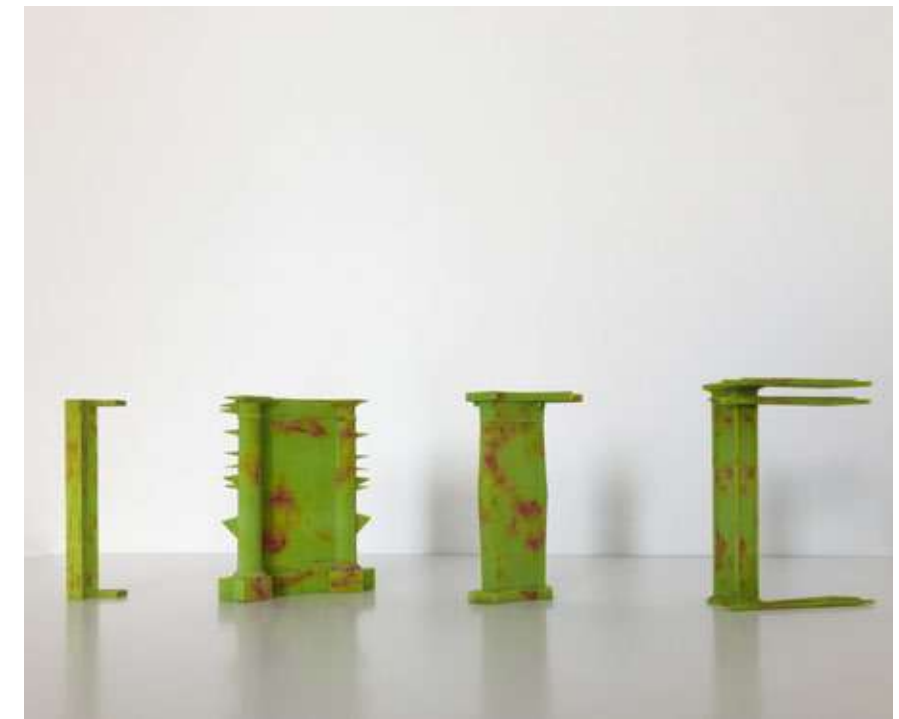
3D printed columns Four of the columns printed in the gypsum printer
